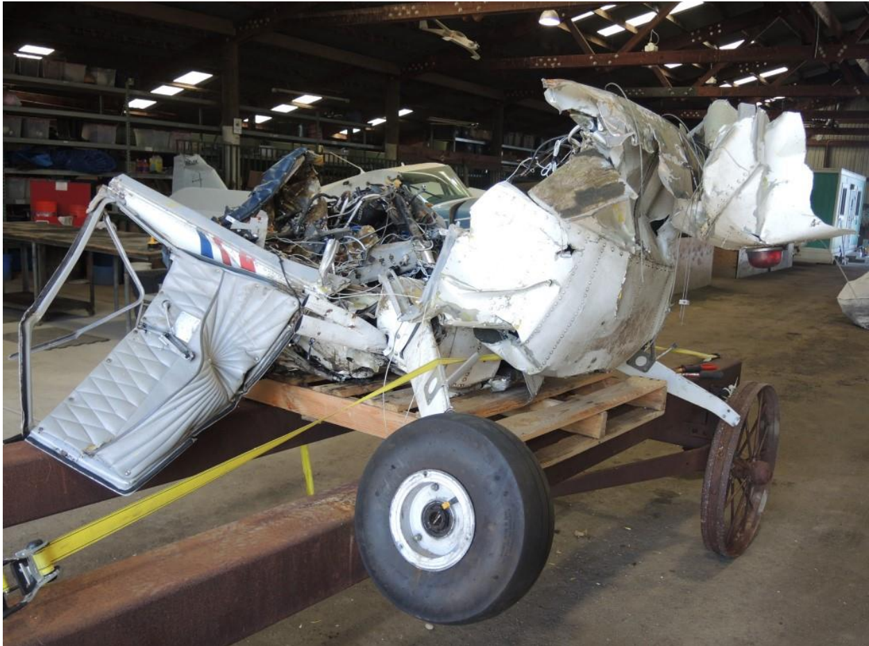
Figure 3 - Lower Cabin/Cockpit (After engine removal)
