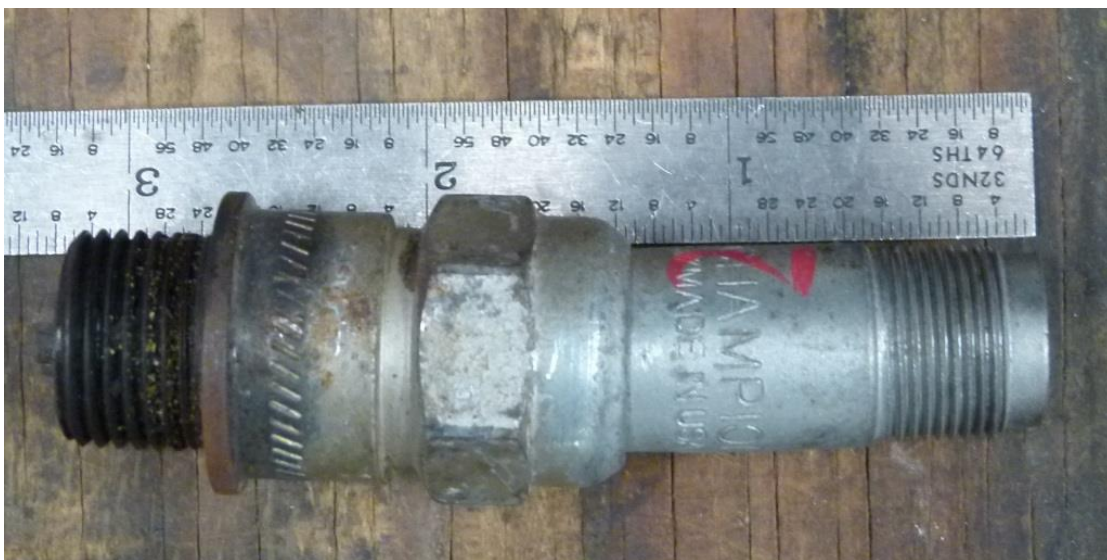
Figure 10 - Cylinder 2 Top Spark Plug Deformation
