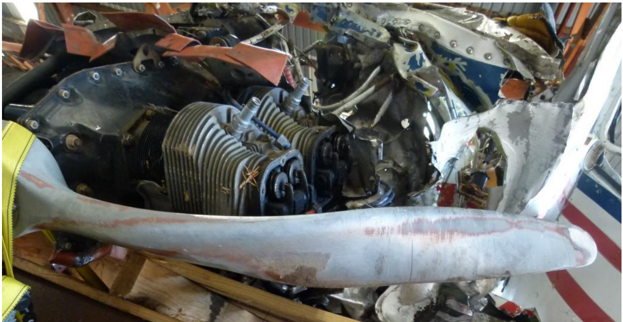
Figure 14 - Propeller Blade with "S-Bending"
