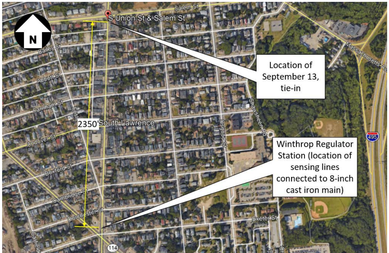
Figure 8 -- Relative location of Feeney Brothers crew to regulator vault location
