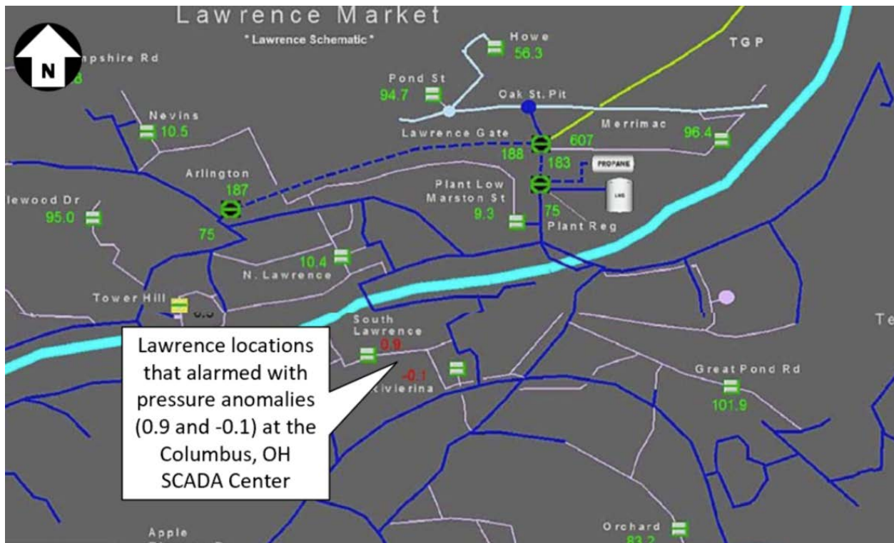
Figure 3 -- Lawrence locations that alarmed at the Columbus, OH SCADA Center
