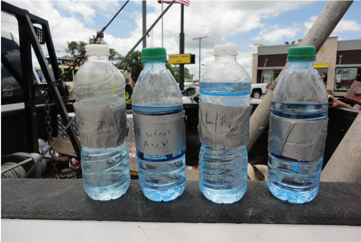
Fuel samples taken at the scene. From the left: right main tank, right aux, left aux, left main tank.
