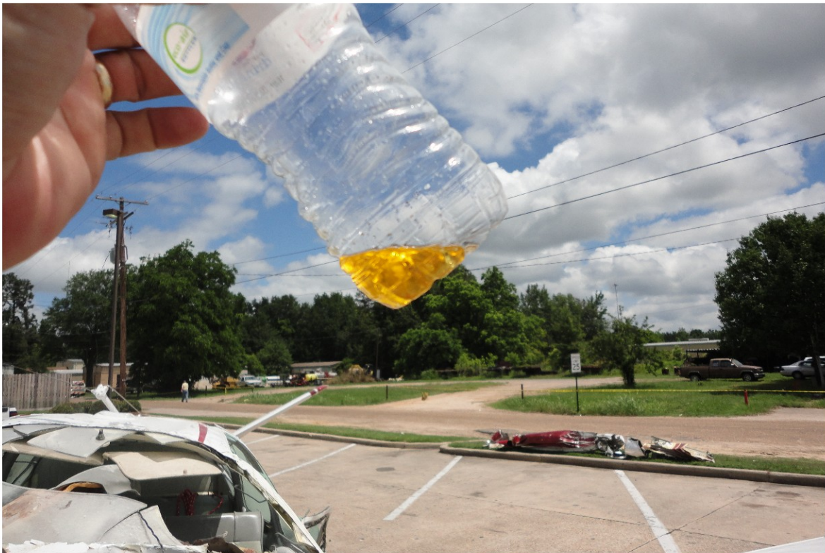
Fuel found in the fuel line headed to the engine. The fuel is discolored with an orange tint. This fuel was sent for analysis and the report is included in the public docket.
