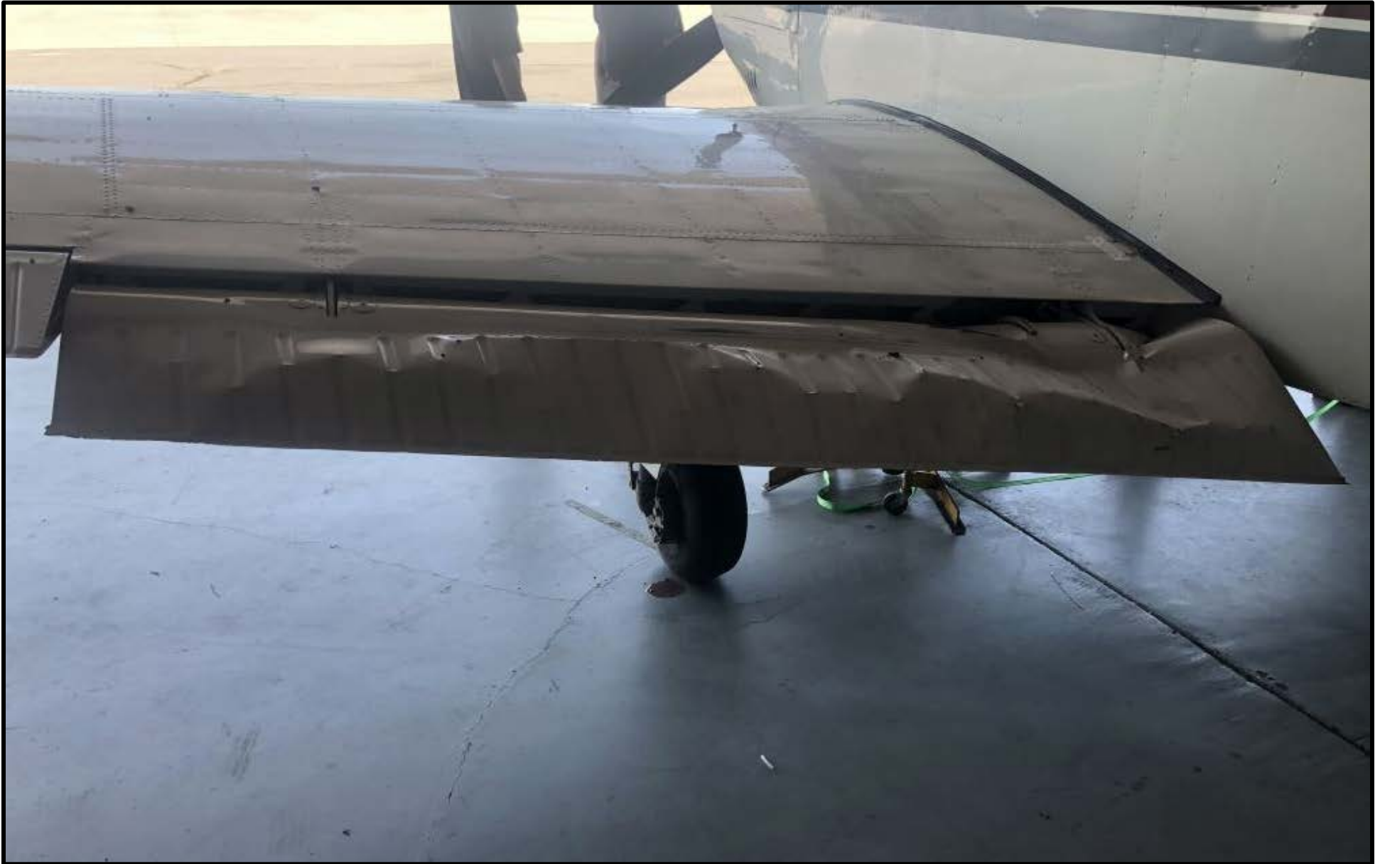
Figure 1: Airplane Damage - Aileron
