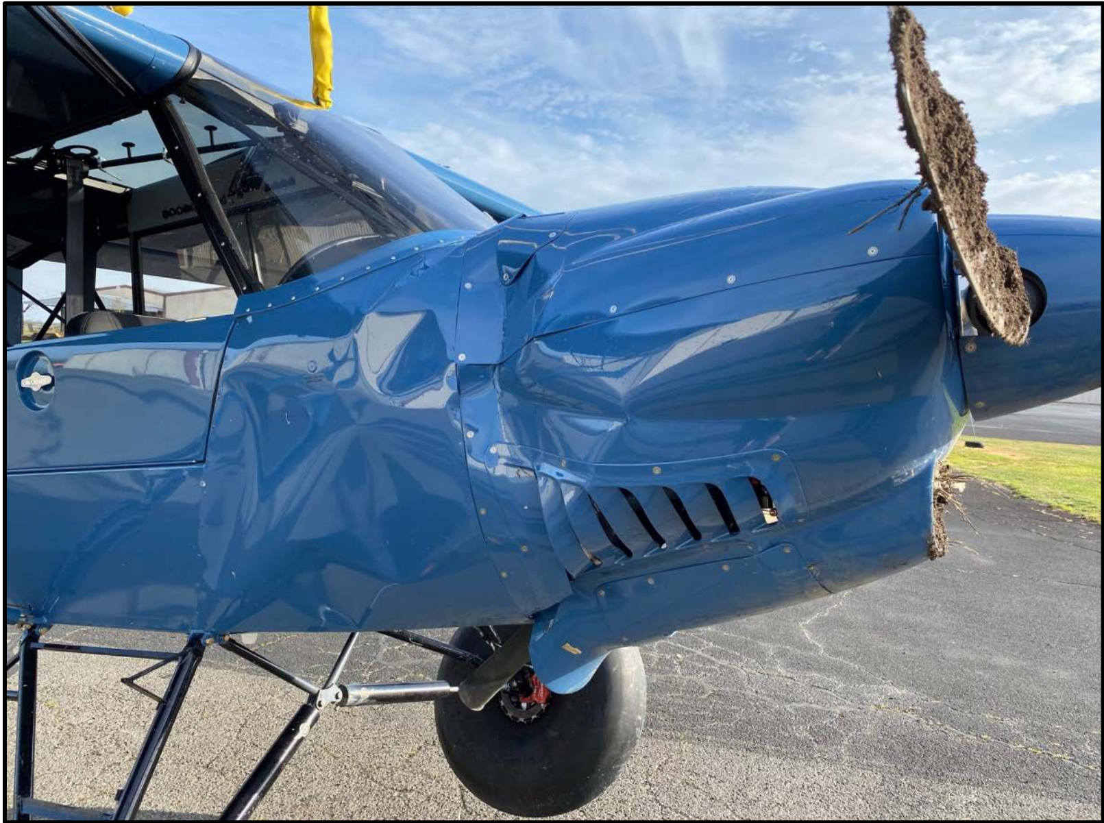
Figure 1: Airplane Damage: Nose
