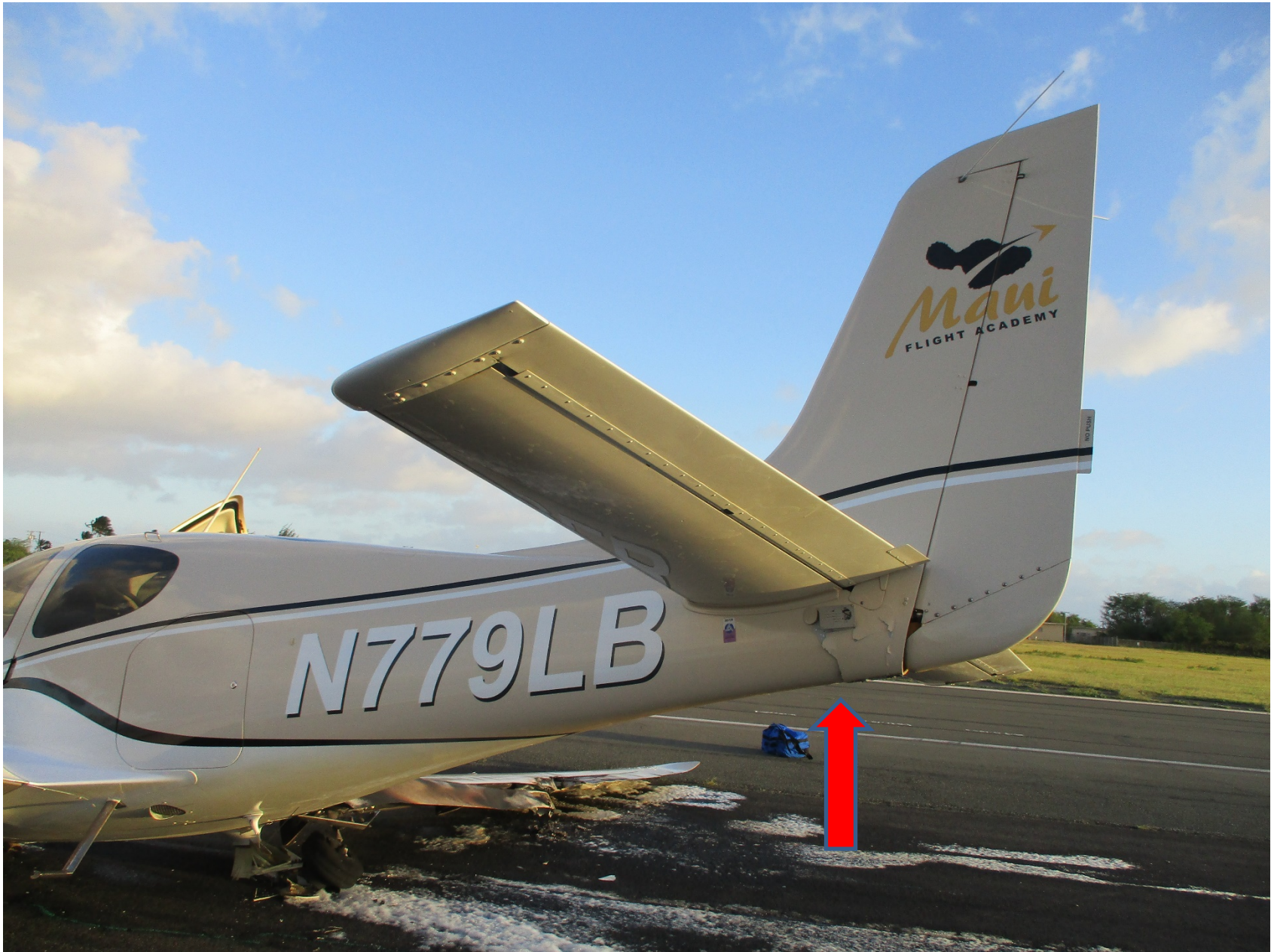
Photo 2 – Substantial damage to the empennage (Photograph compliments of the FAA)
