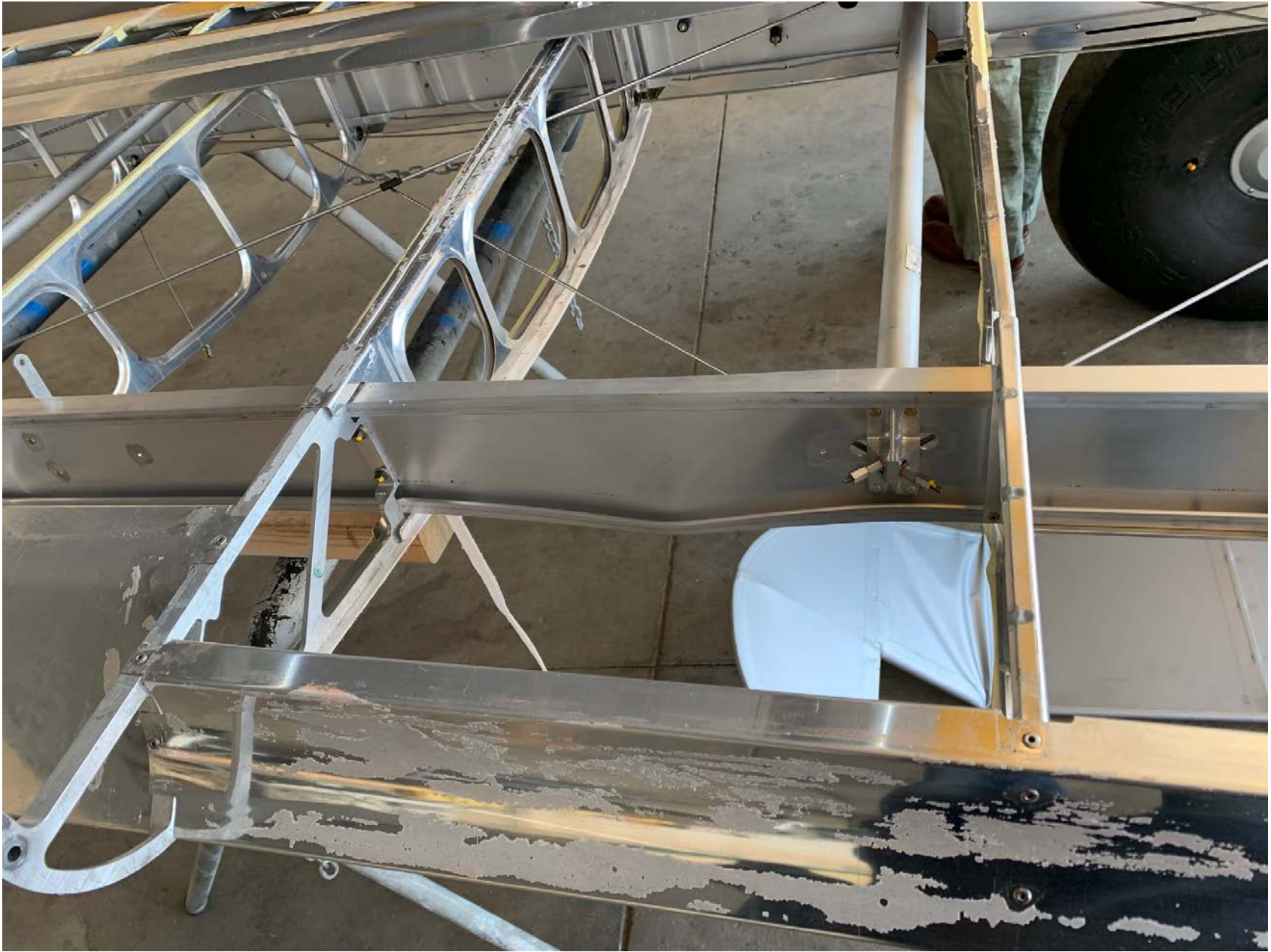
Photo 2 – Accident airplane’s damaged left wing spar.
