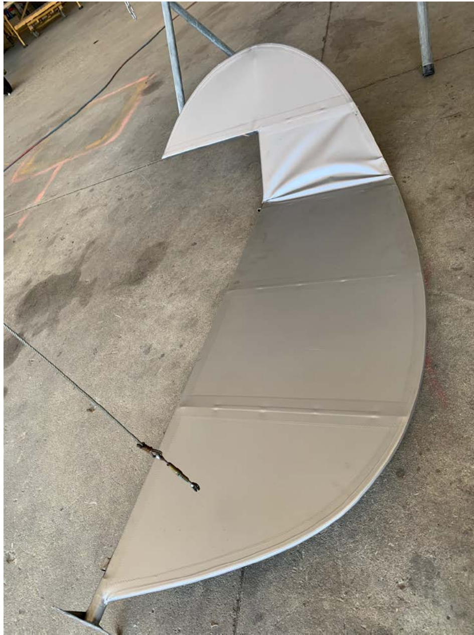
Photo 3 – Accident airplane’s damaged left elevator.
