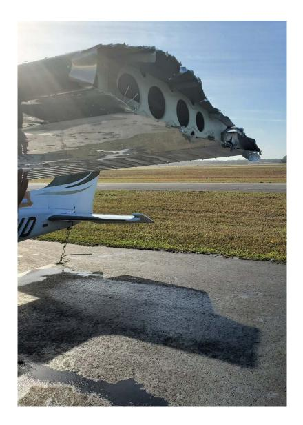
Photo 1 –View of Inboard Section of Severed Wing (Photo Courtesy of Phoenix East Aviation)
