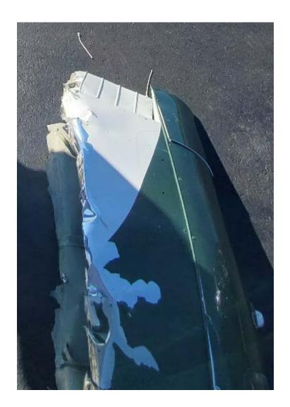
Photo 2 – View of Severed Wingtip (Photo Courtesy of Phoenix East Aviation)
