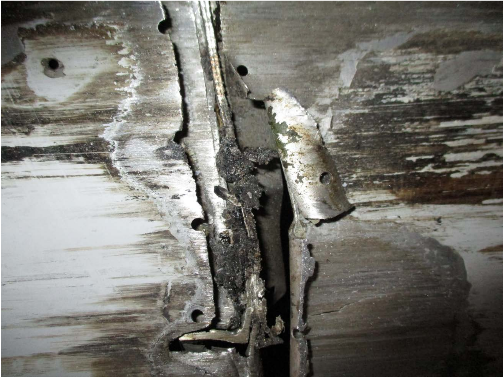
Photo 3 – Aft Spar Abrasion Damage (FAA Photo)
