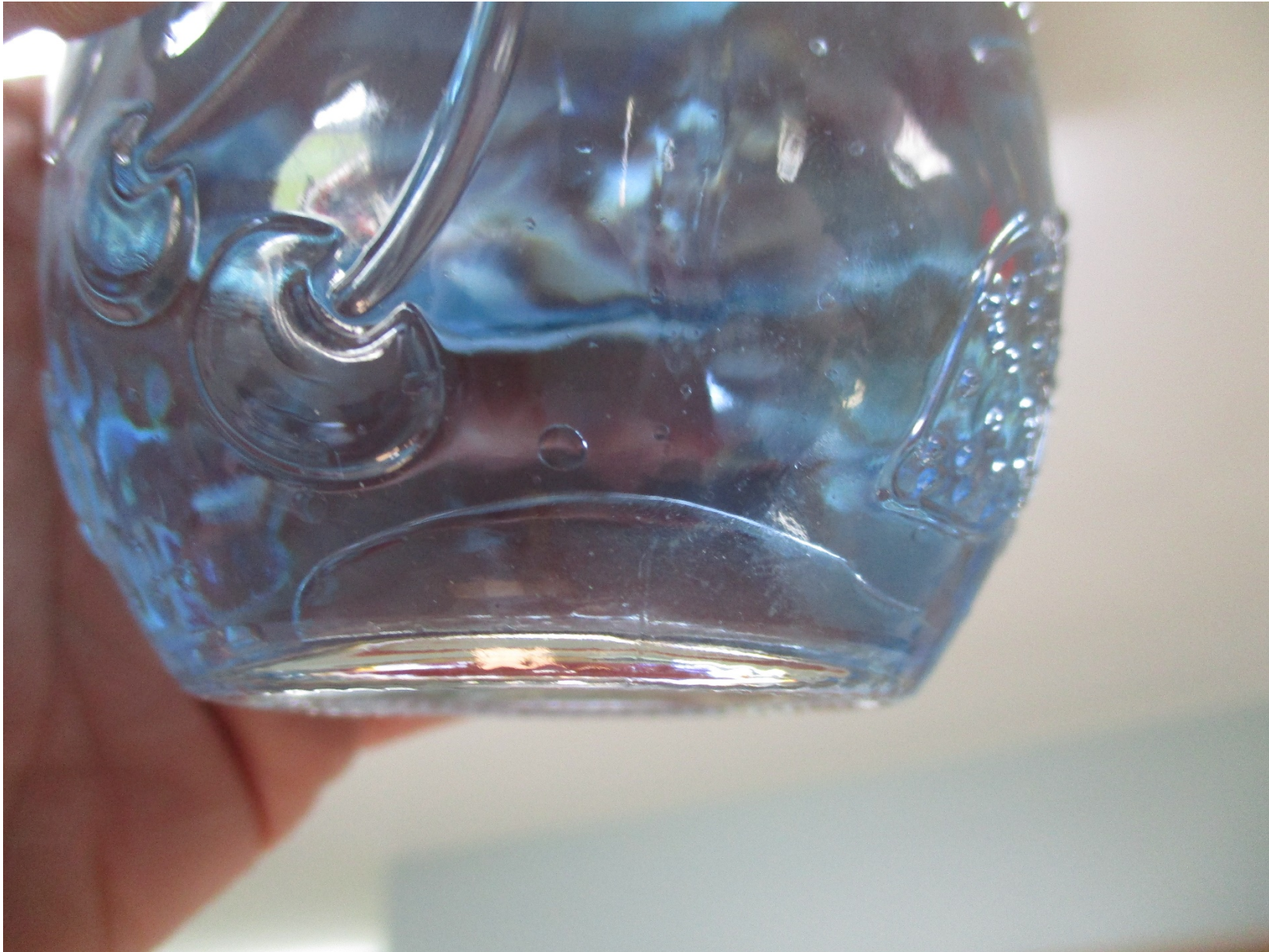
Photo 4 – Left Auxiliary Tank Fuel Sample (FAA Photo)
