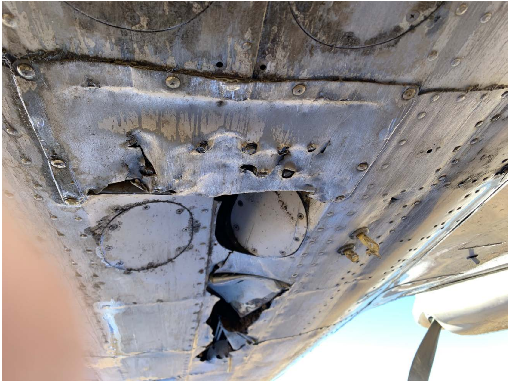
Photo 2 – Forward looking picture of accident airplane’s damaged belly.
