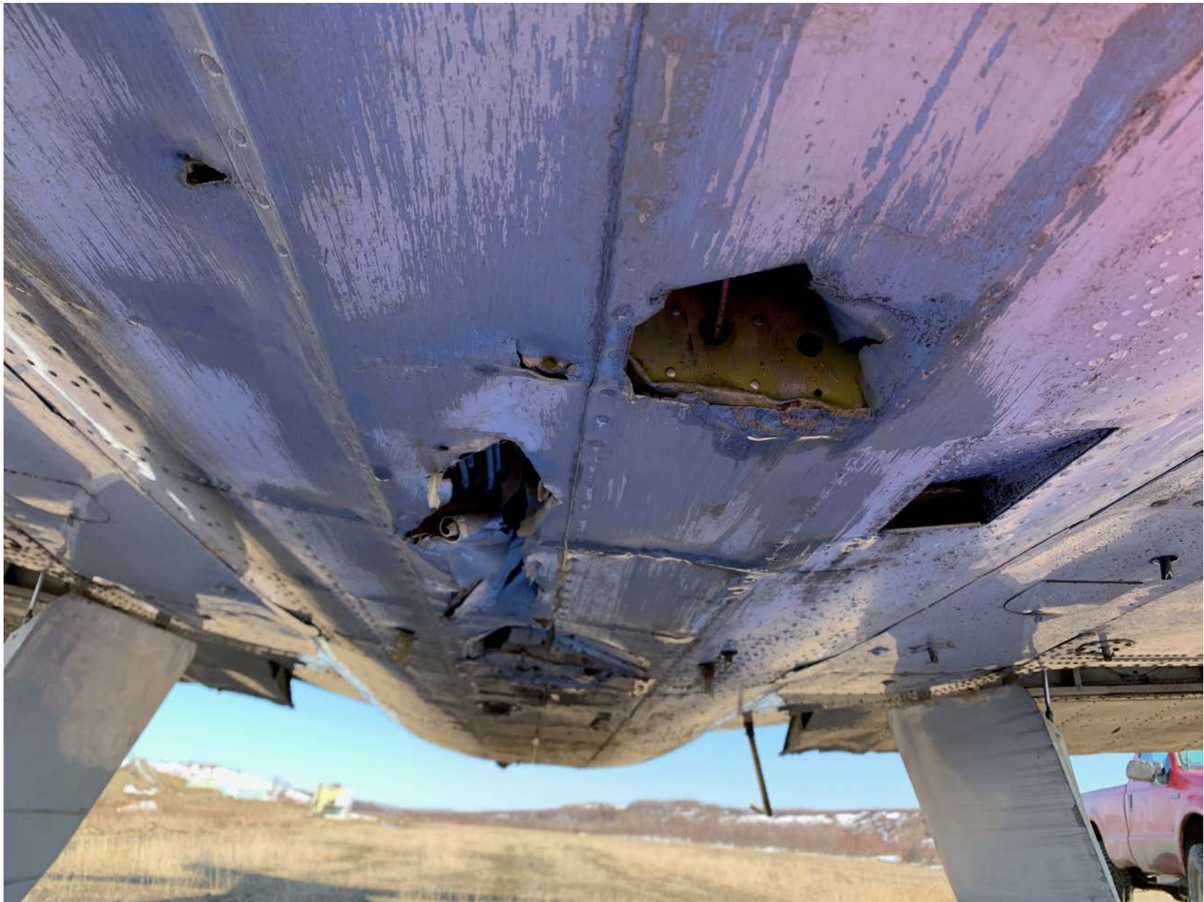
Photo 3 – Aft looking picture of accident airplane’s damaged belly.
