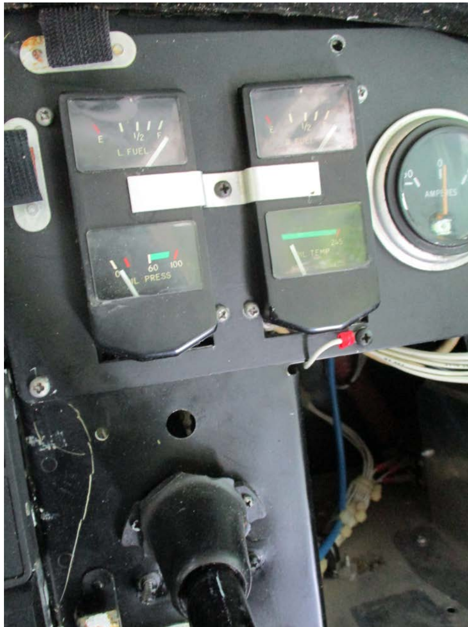
Photo 4 - FAA supplied view of the fuel tank gauges at the accident site. Both left and right fuel gauges have a full indication.
