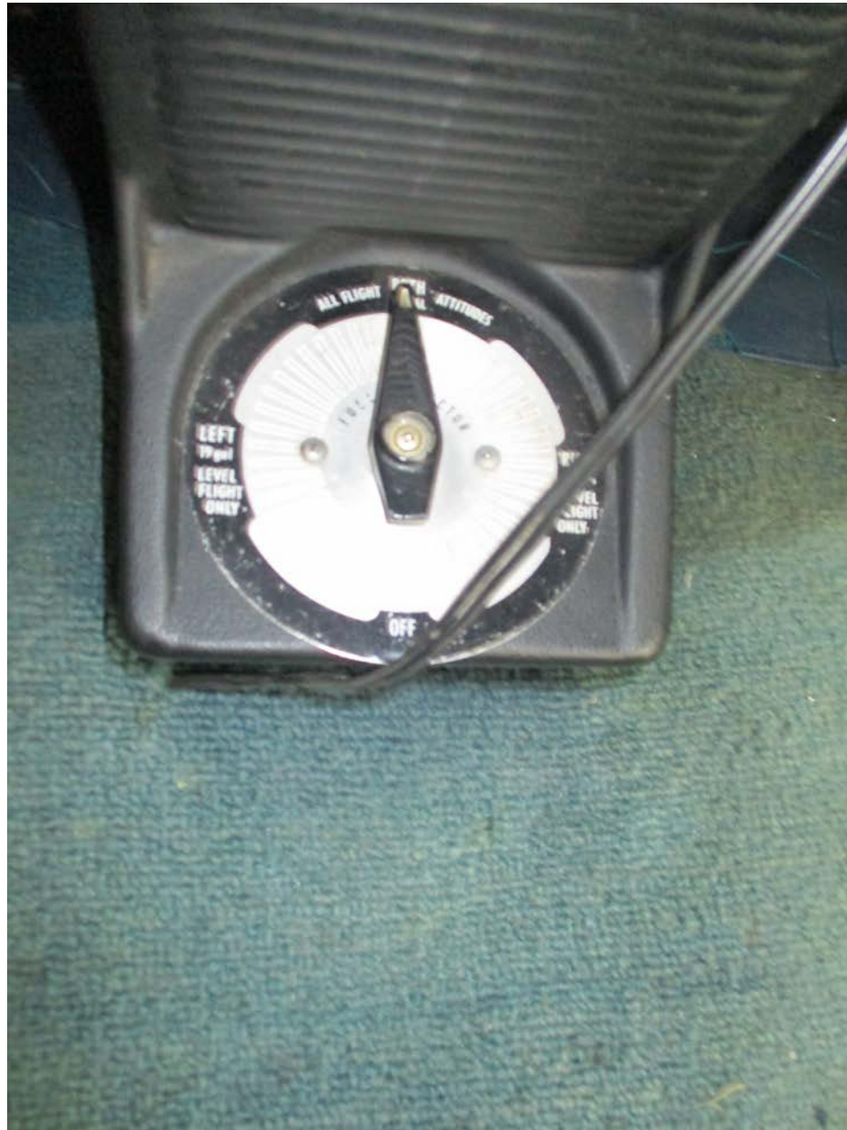
Photo 3 - FAA supplied view of the fuel tank selector. The selector is positioned to select both left and right tanks.
