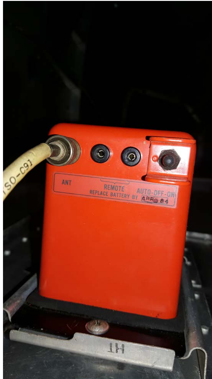
Photo 5 - FAA supplied view of the emergency locator transmitter at the accident site. The transmitter's switch is in the off position.
