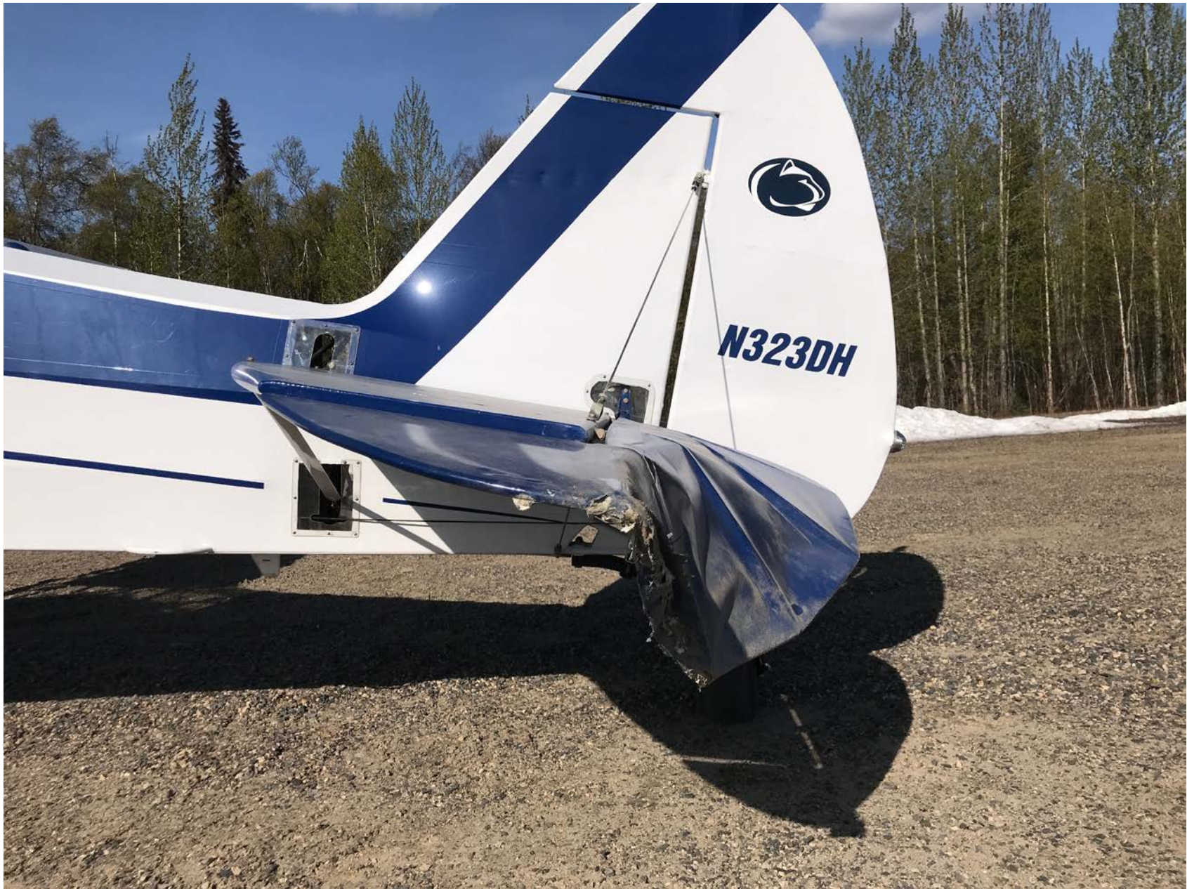
Photo 3 – Accident airplane’s damaged left elevator.
