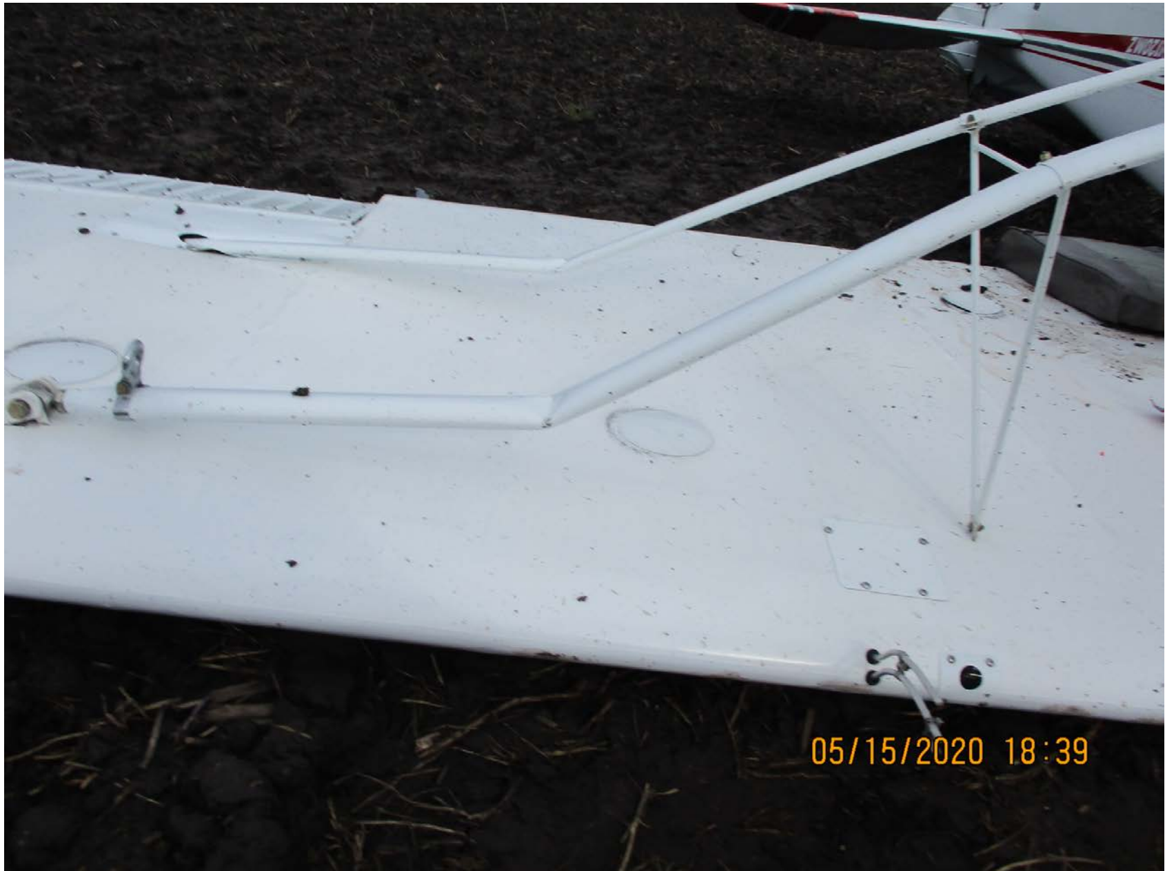
Photo 2 – Bent Left Wing Struts (FAA Photo)
