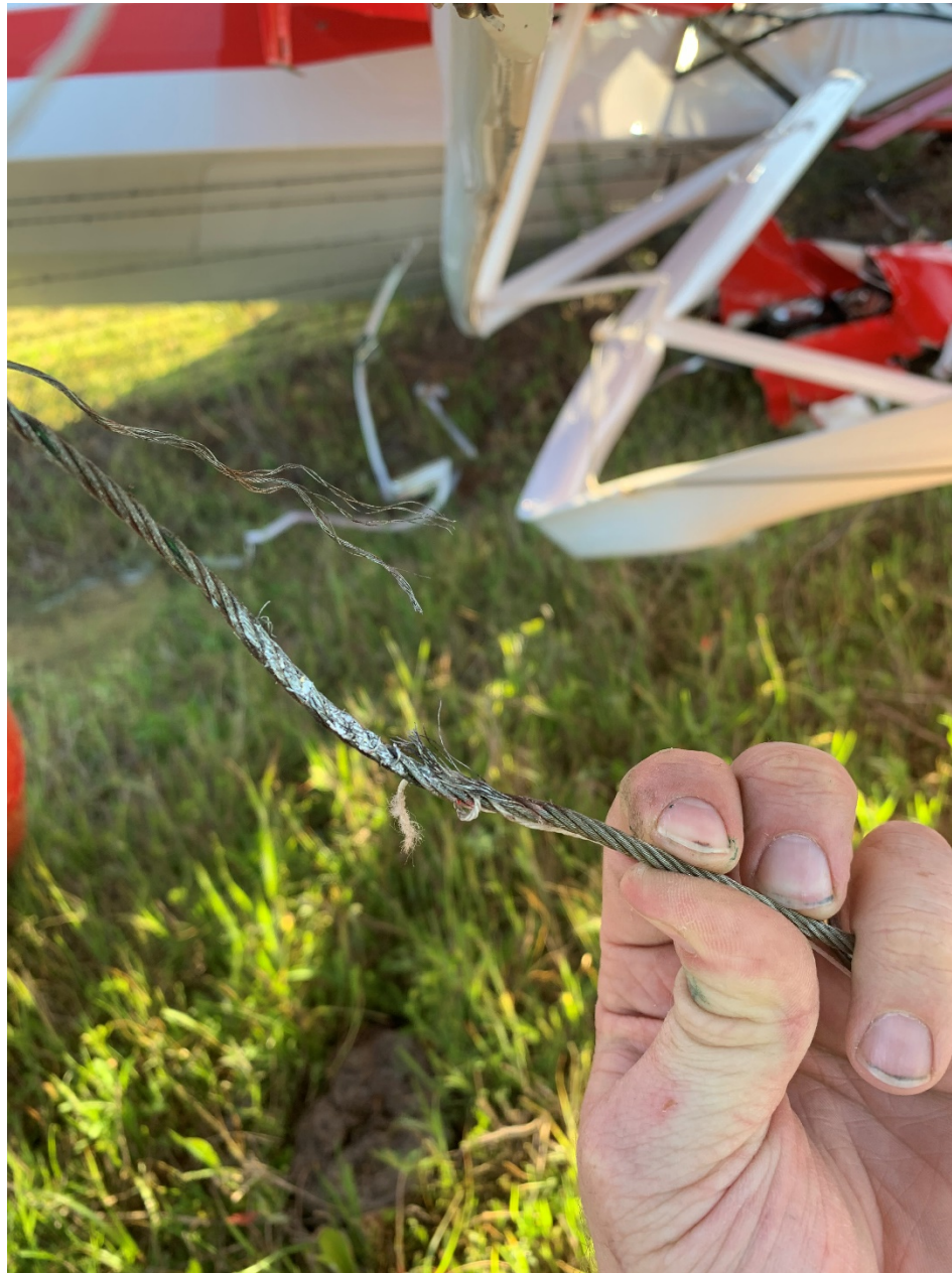
Photo 3 – Damage to aileron control cable
