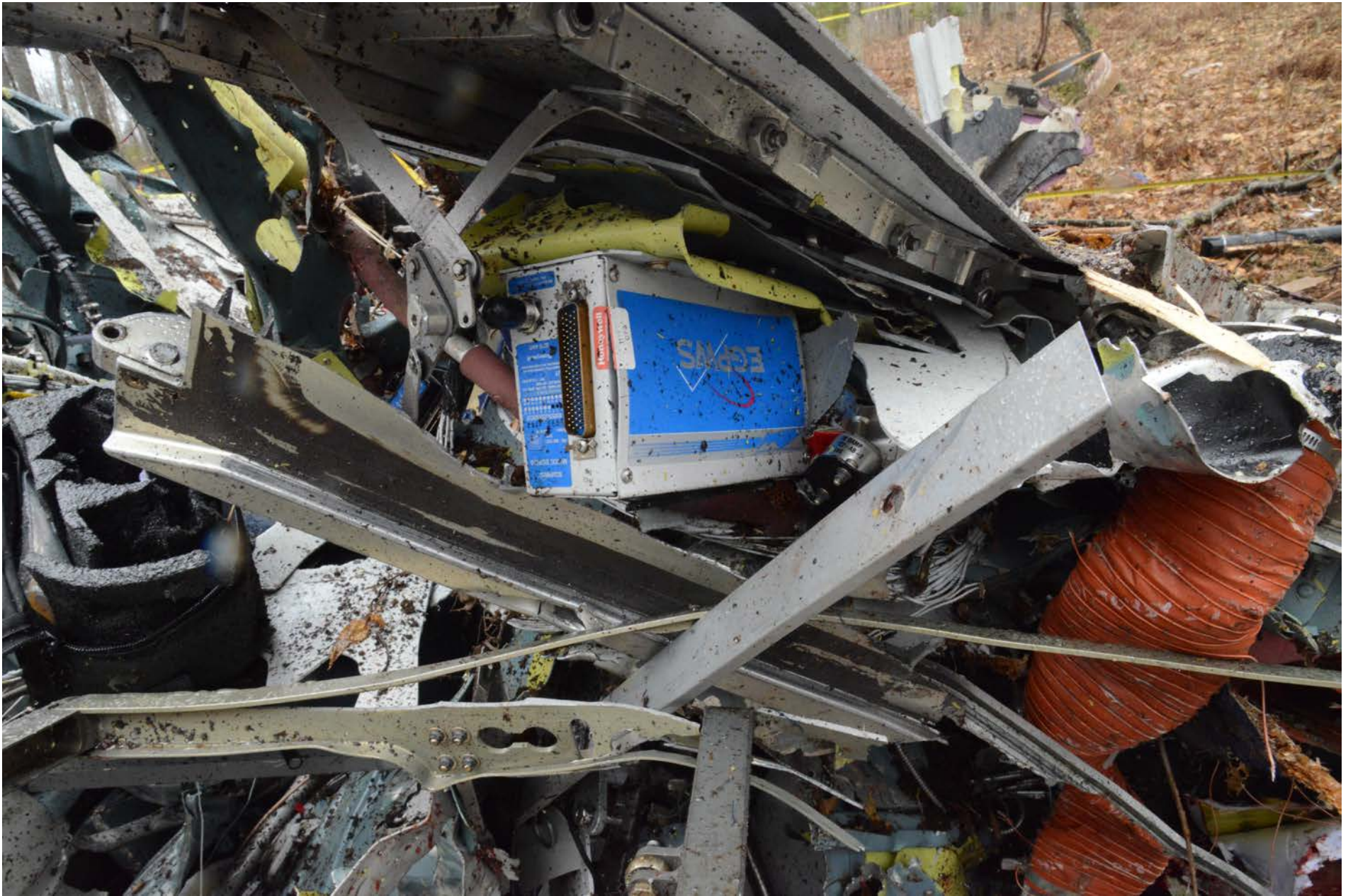
Photo 7 - View of the EGPWS unit.
