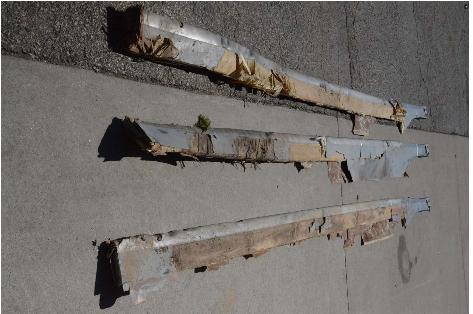
Photo 16 - View of removed main rotor blades.
