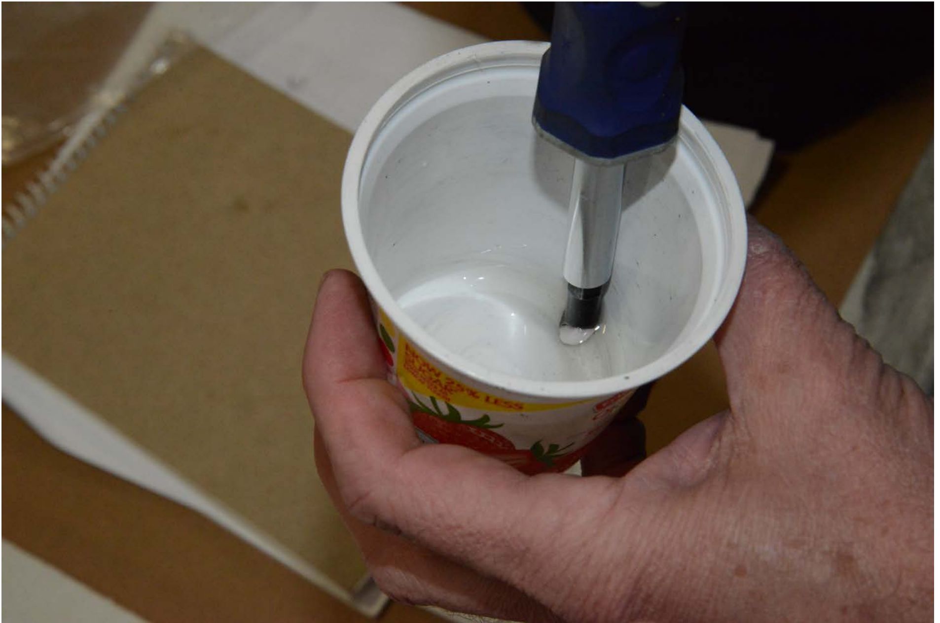
Photo 13 - View of recovered fuel being tested for water. The water testing paste did not indicate a presence of water.
