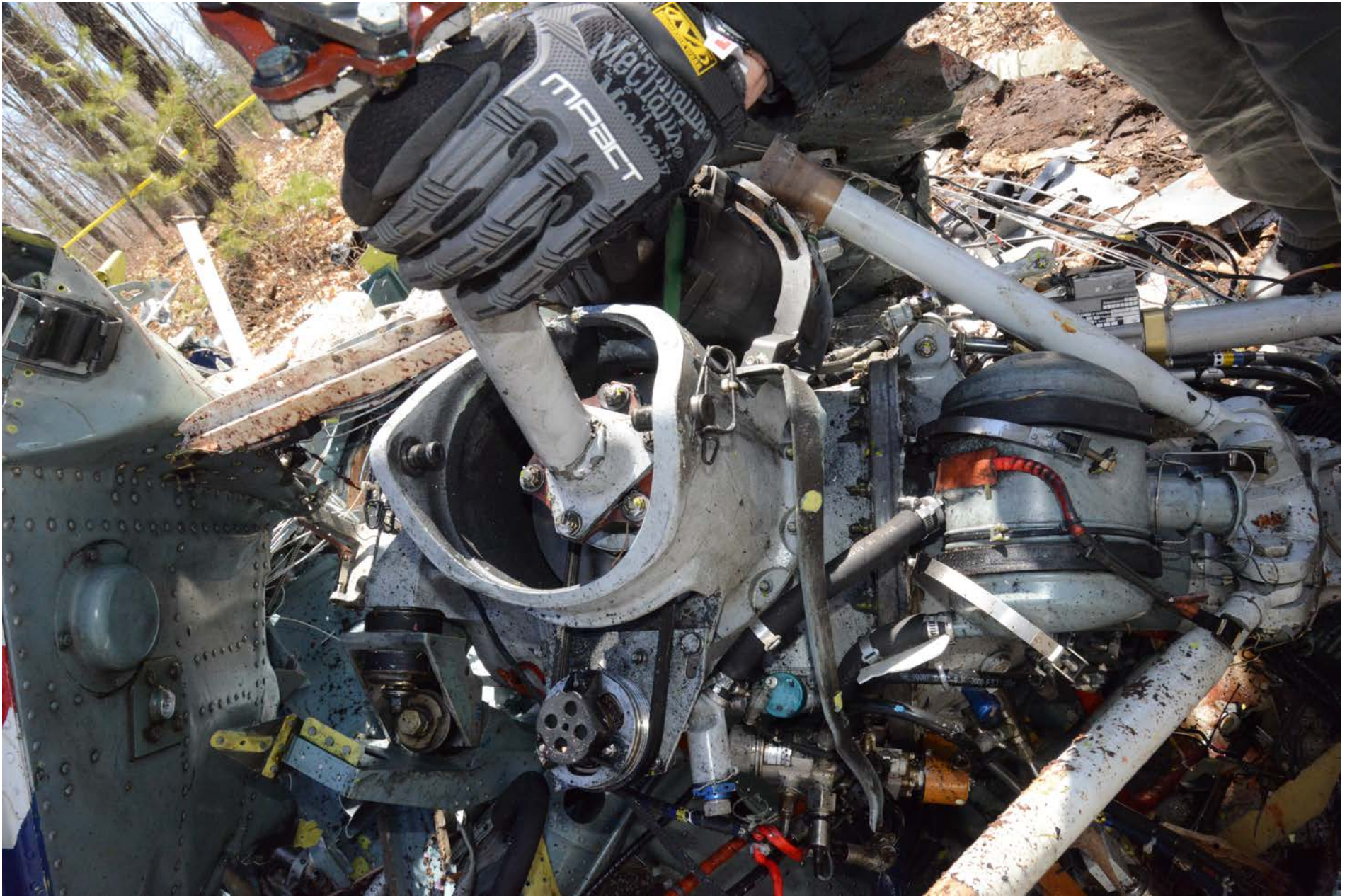
Photo 11 - View of a separation in the driveshaft.
