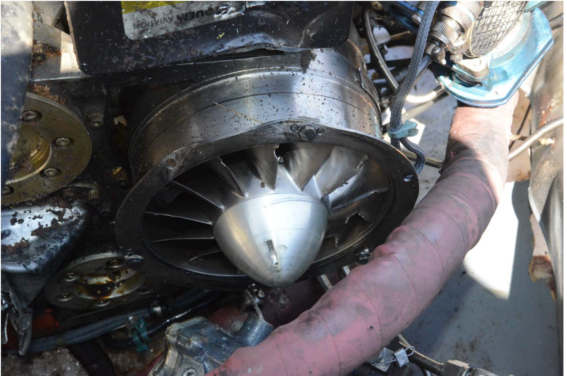
Photo 10 - View of the engine intake. Blades exhibit damage consistent with FOD ingestion.
