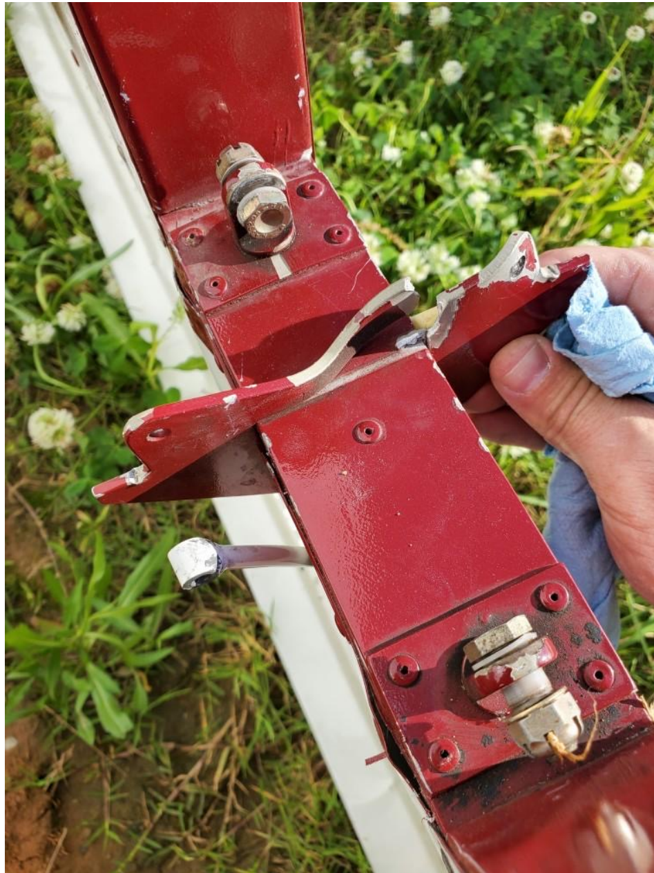
Photo 5 - Fractured stabilator control horn
