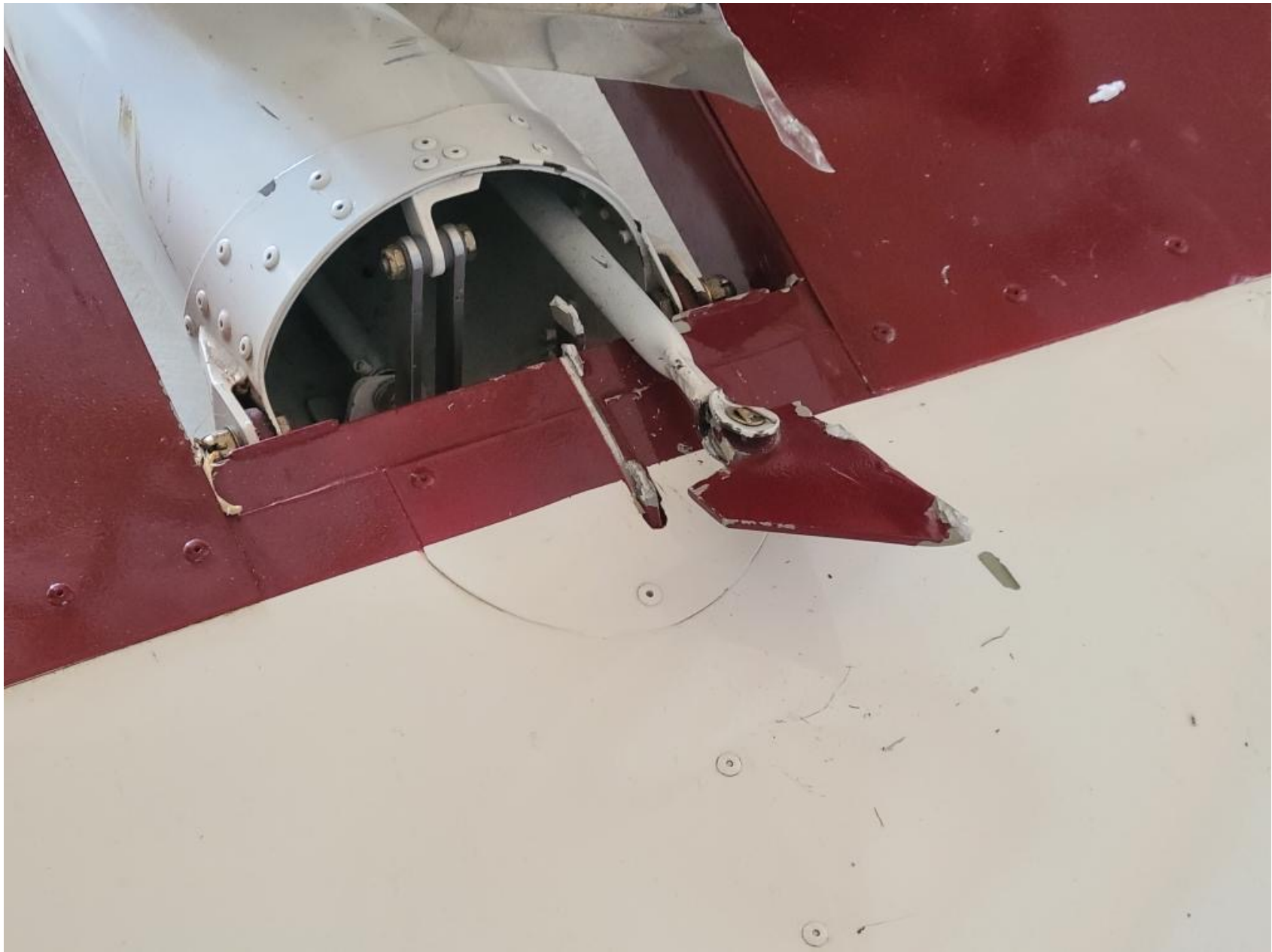
Photo 3 – Fractured stabilator control horn
