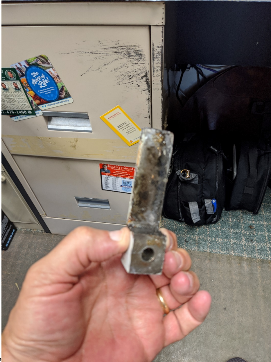
Photo 1: Fractured attach bracket
