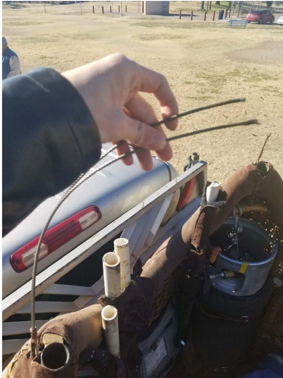
Photo 1 – View showing two broken Basket suspension Cables
