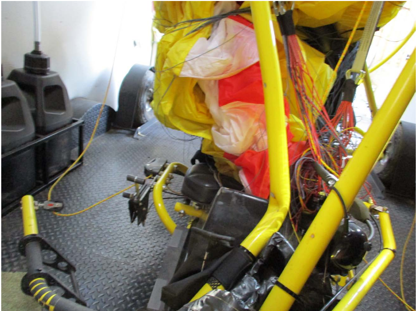
Photo 2 - Front View showing Frame Damage
