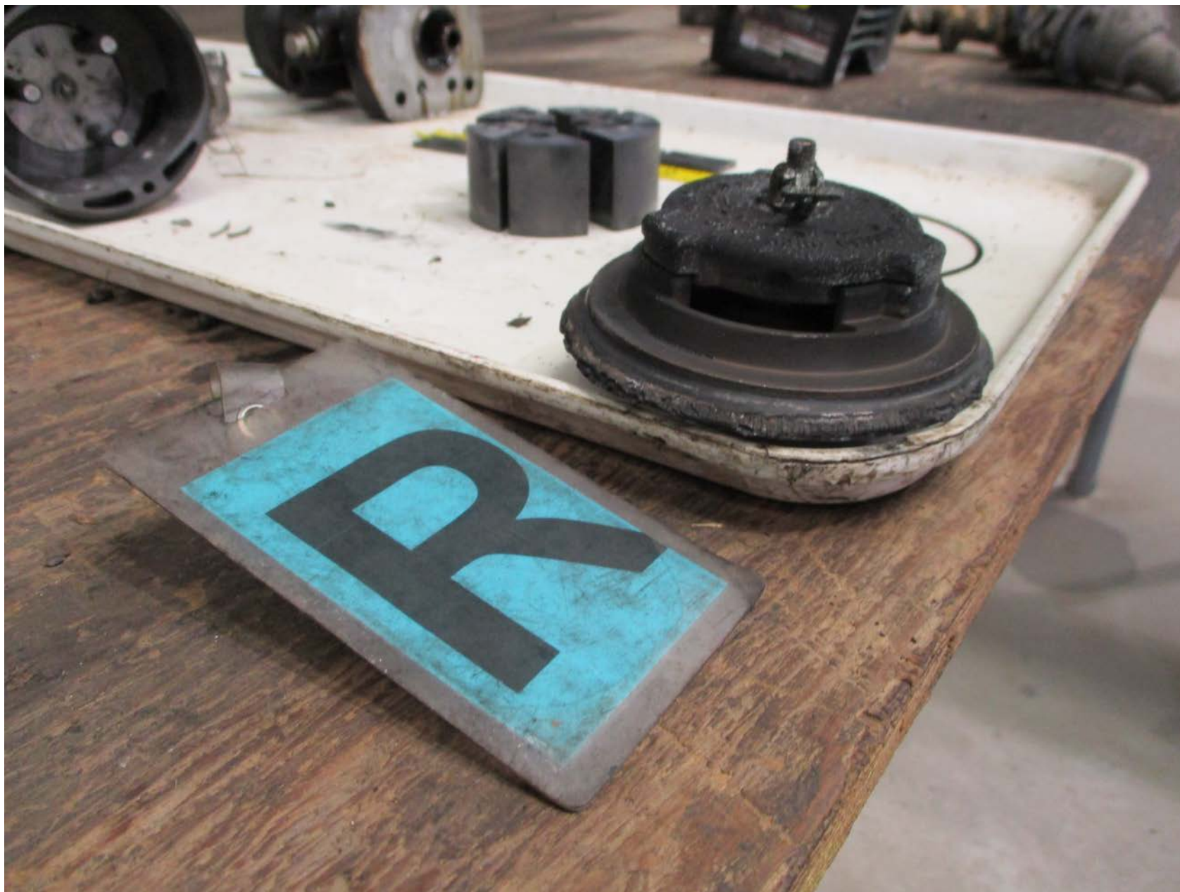
Photo 6 – Thermal damage to right fuel cap seal.
