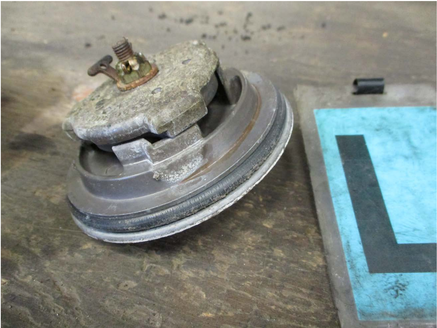
Photo 7 – Cracks around circumference of left fuel cap seal.
