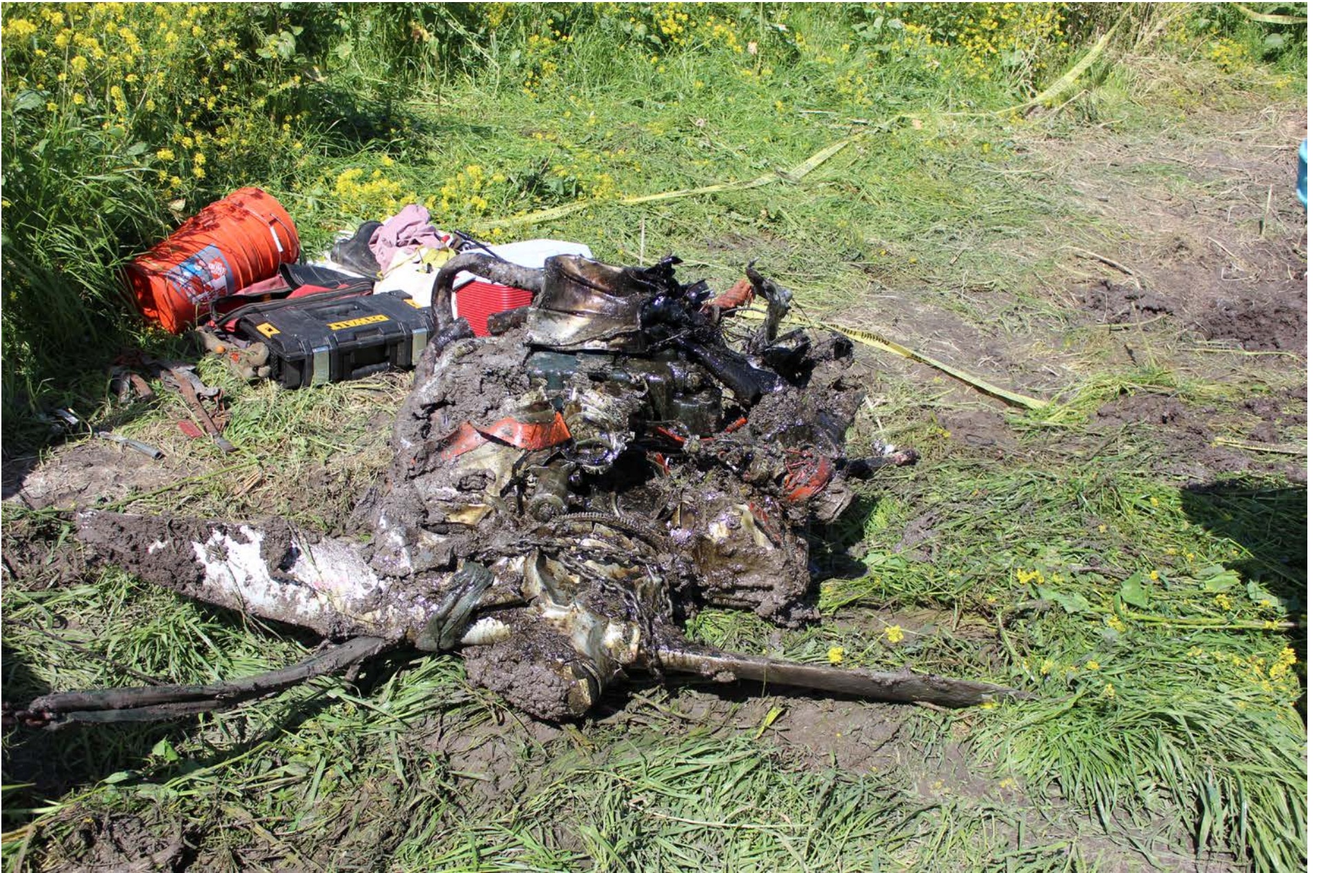
Photo 5 – Accident airplane's engine after removal from mud at accident site.
