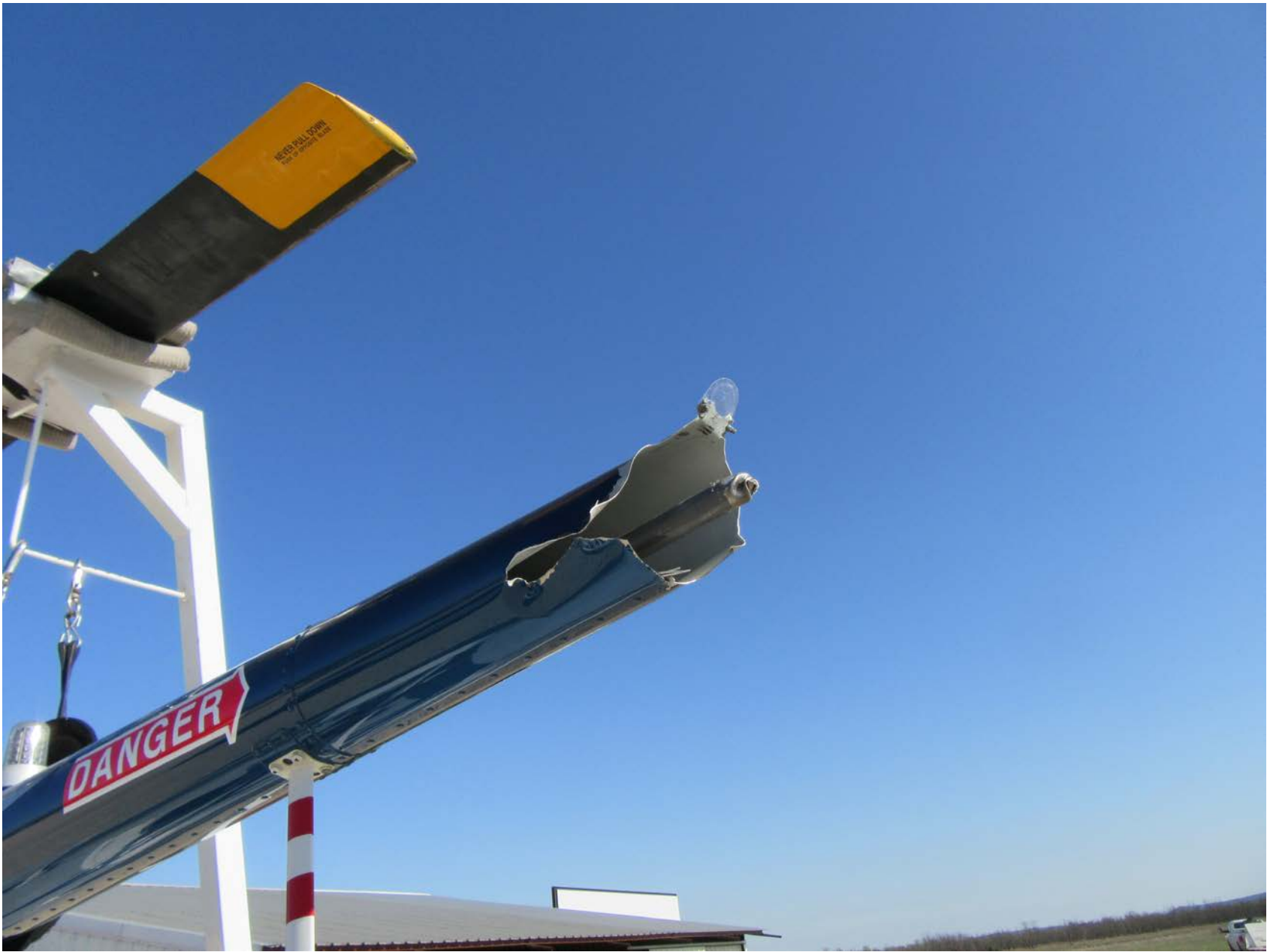
Photo 1 – Severed Tailboom (Photo courtesy of FAA)
