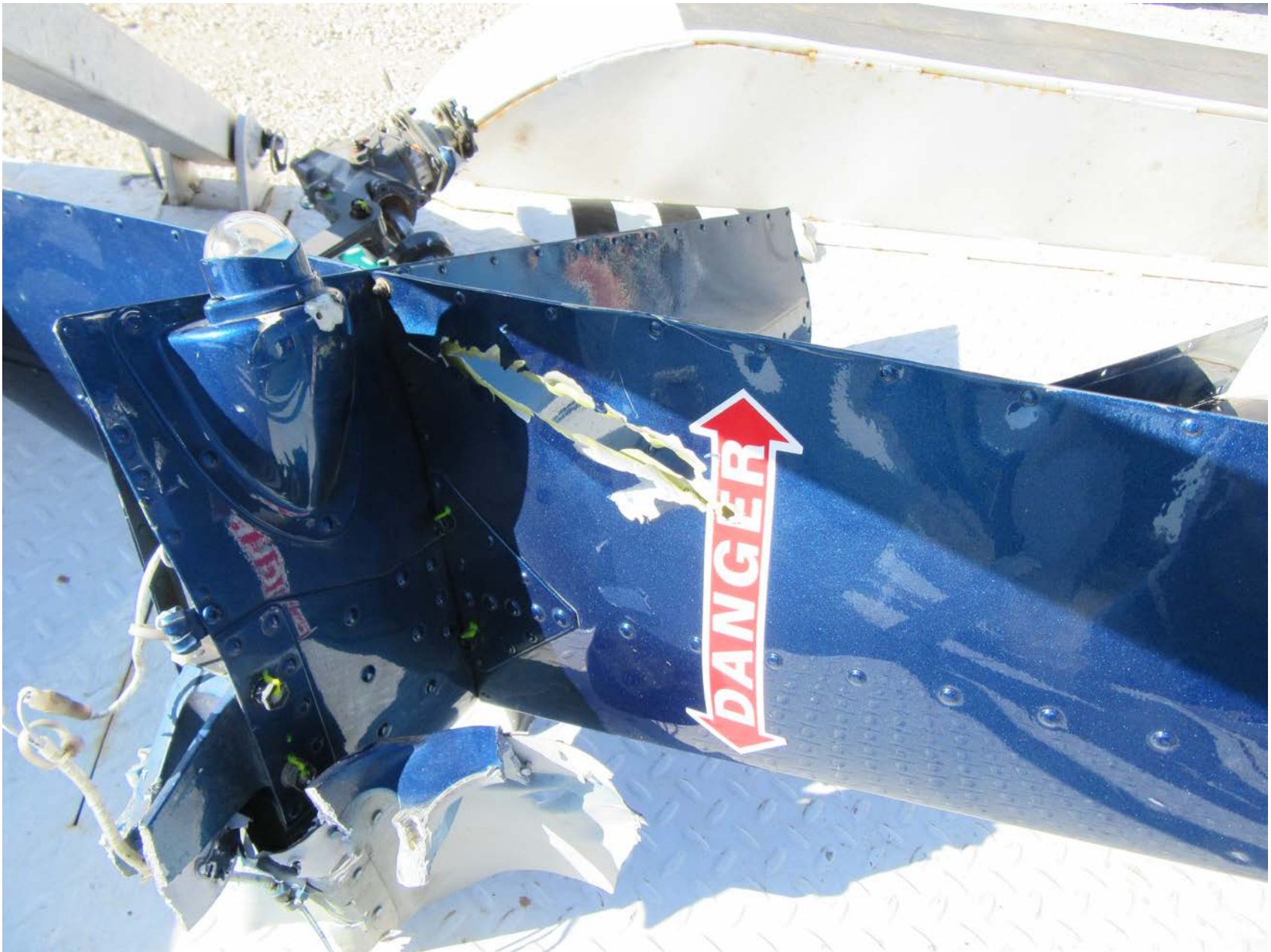
Photo 2 – Tailrotor Damage (Photo courtesy of FAA)
