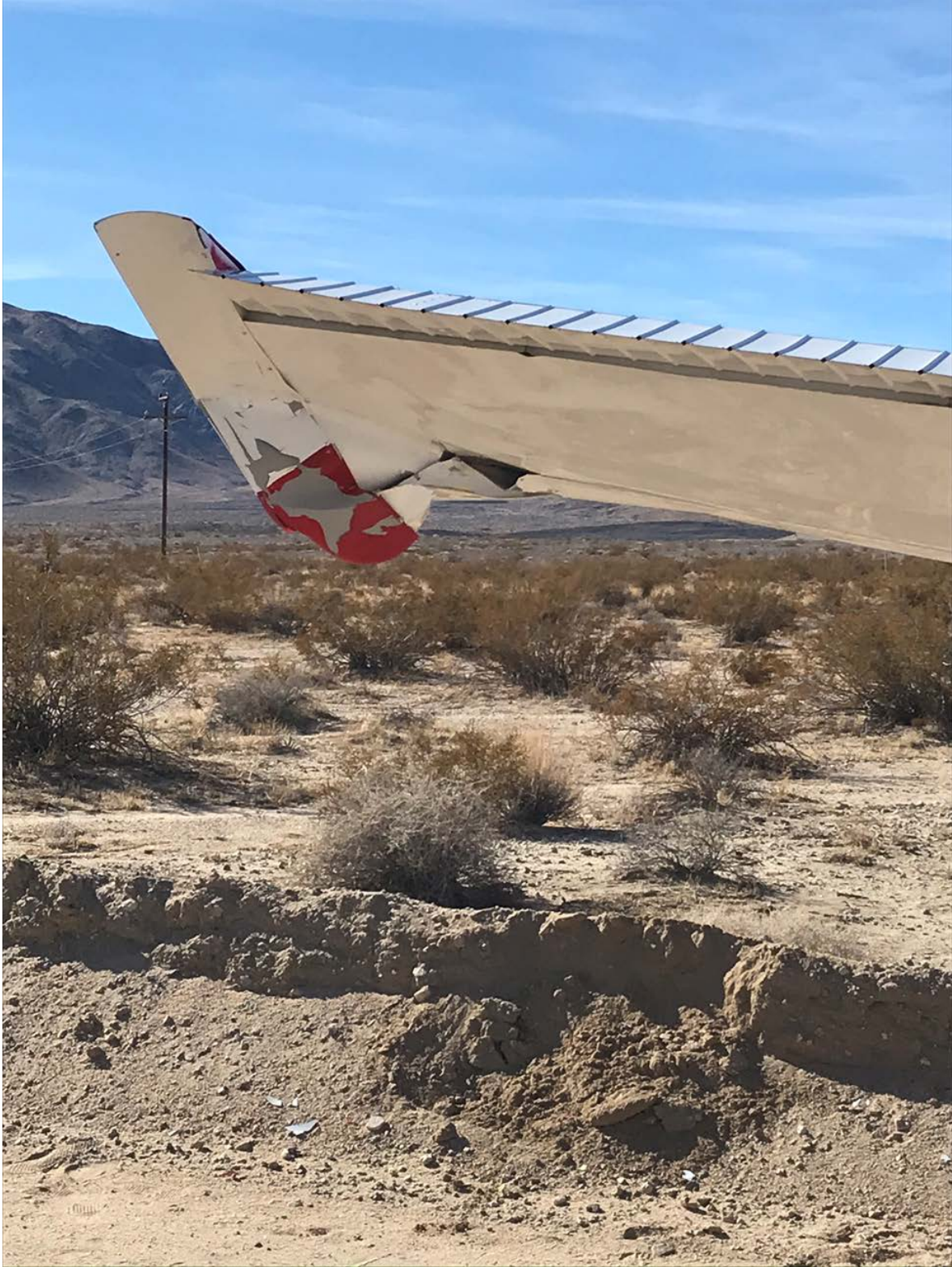
Photo 2: Damage to the wing outboard (GSowards Owner)
