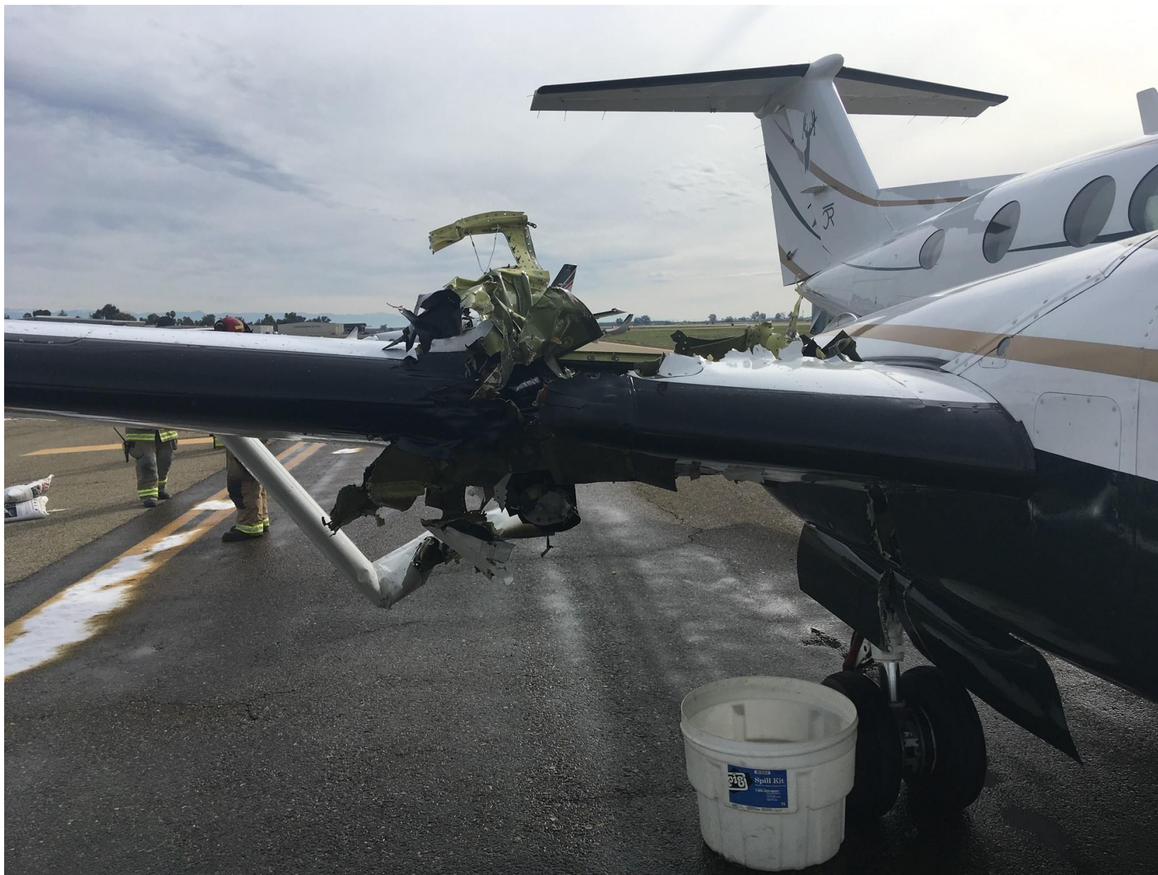
Photo 1 – N160RW showing Substantial Damage to the Right Wing
