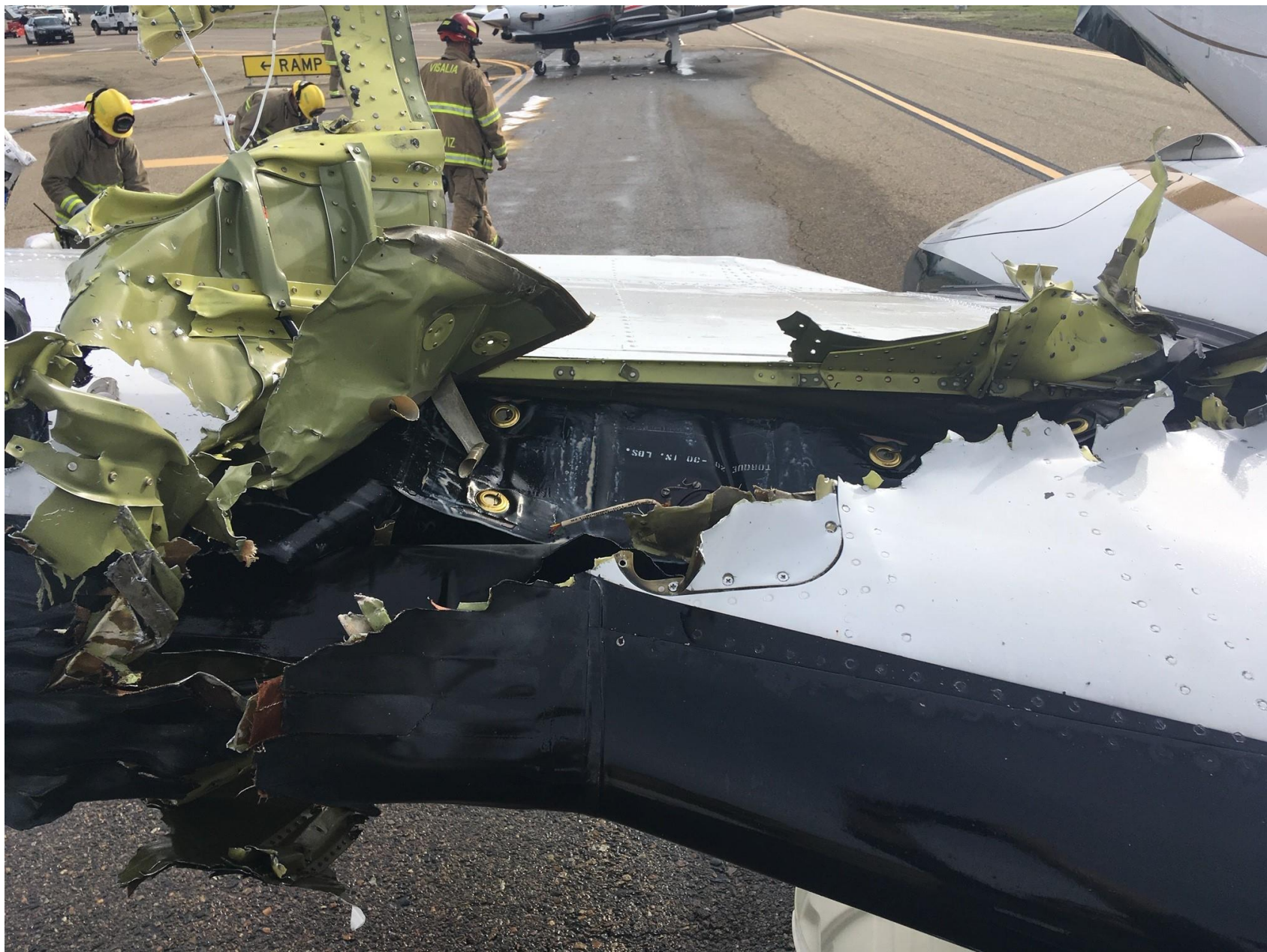
Photo 2 – N160RW showing Substantial Damage to the Right Wing
