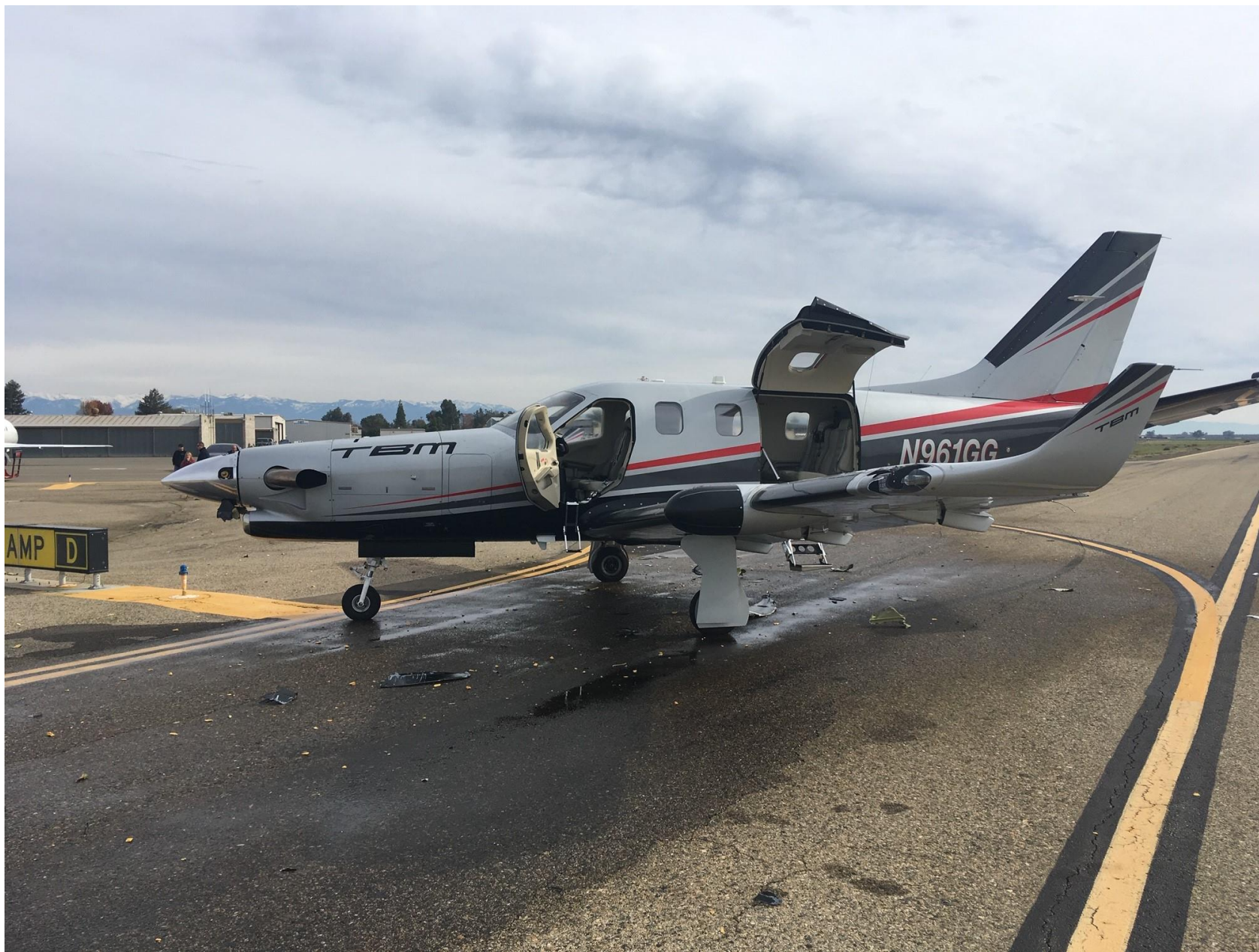
Photo 3 – N961GG Showing damage to the Propeller
