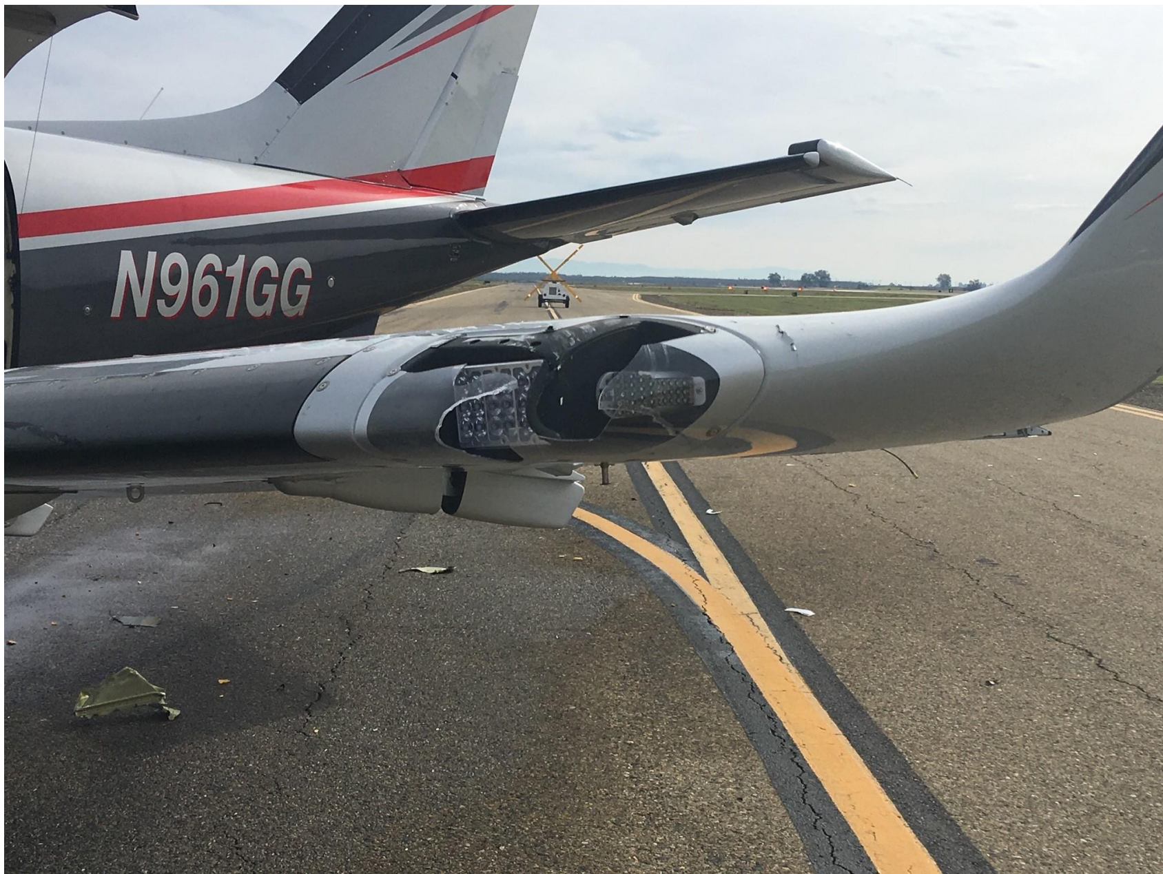
Photo 4 – N961GG showing damage to the Wing Tip
