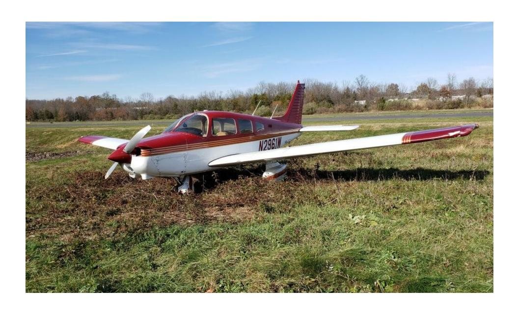
Photo 1-View of damage to the left wingtip and landing gear (Courtesy of FAA)
