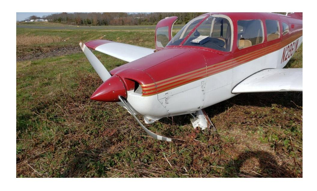
Photo 2 – View of damage to the nose landing gear, left wing leading edge and the propeller (Courtesy of FAA)
