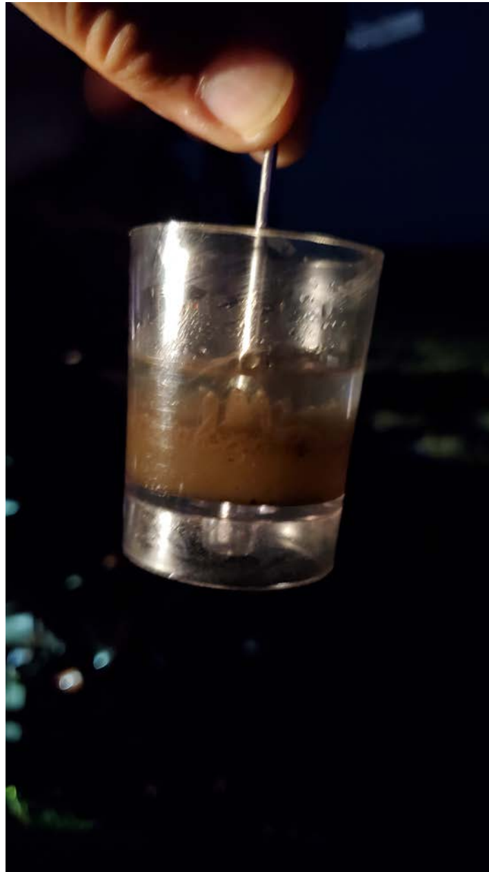
Photo 1 – Left Header Tank Sample (FAA Photo)
