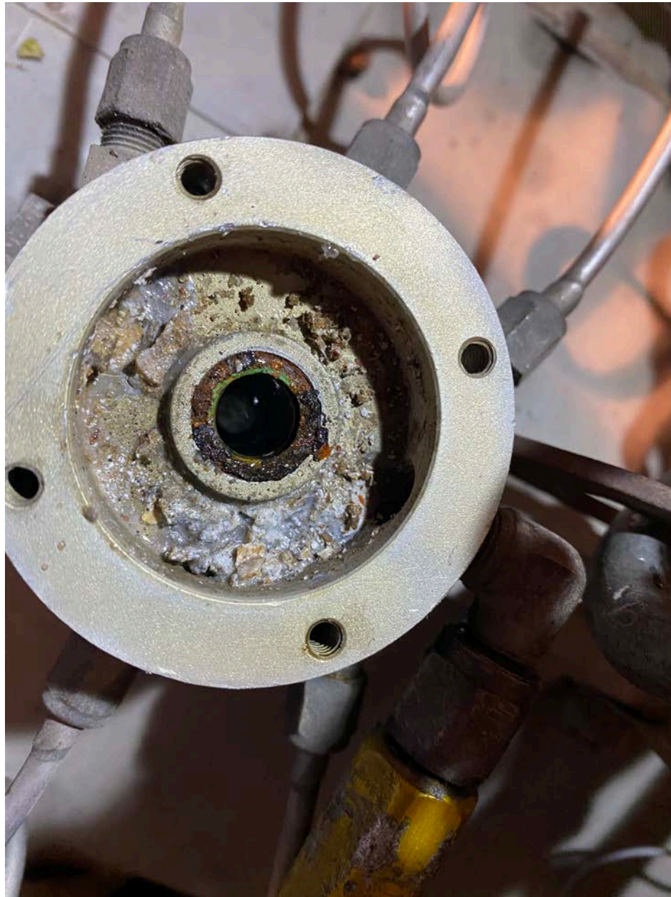
Photo 3 – Fuel Flow Divider (Southern Star Aviation Photo)
