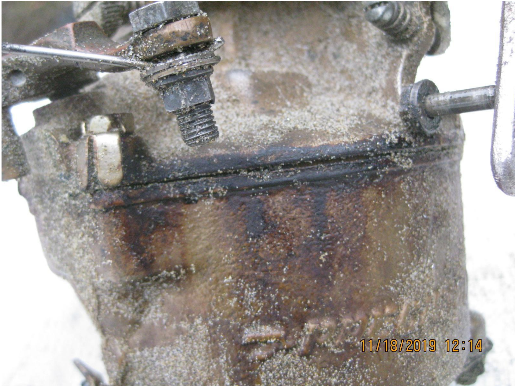
Photo 4 – Accident airplane’s carburetor with staining evident.
