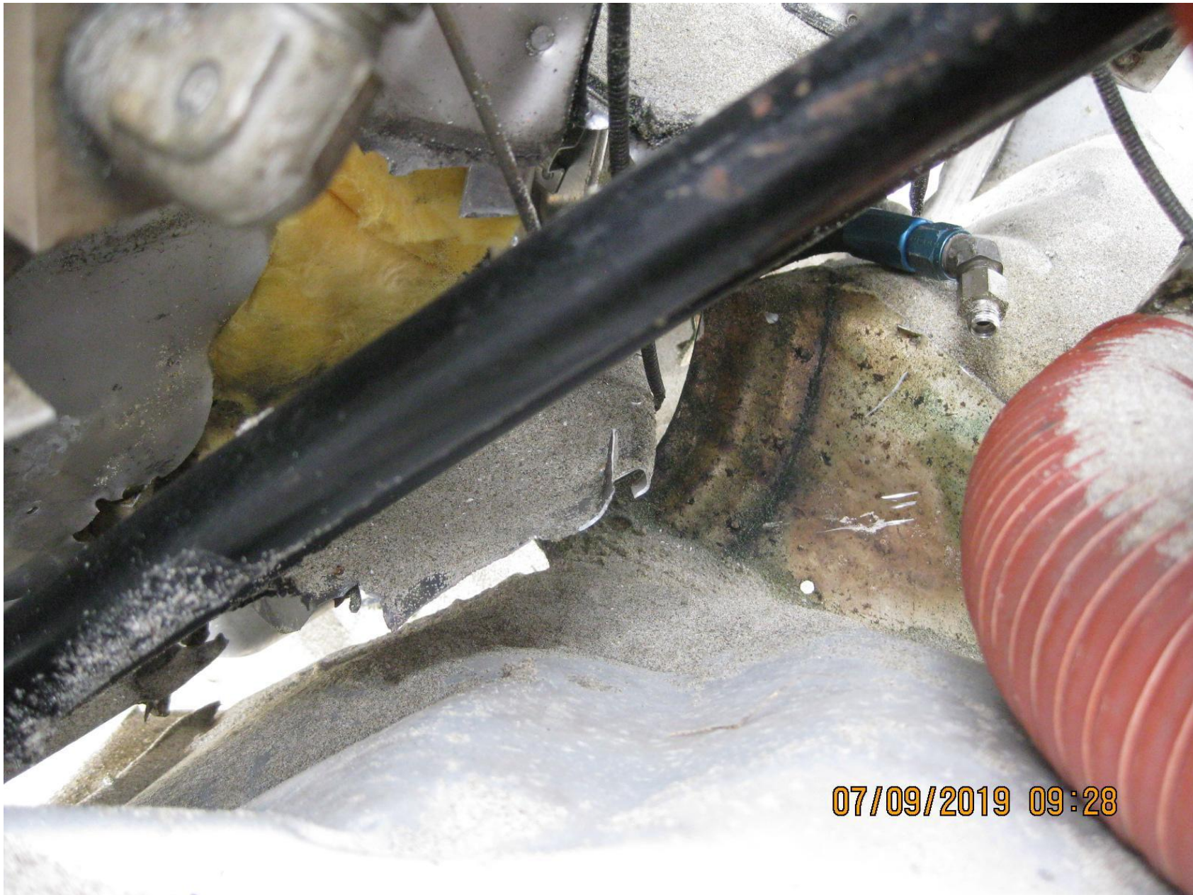
Photo 3 – Separated main fuel line of accident airplane.
