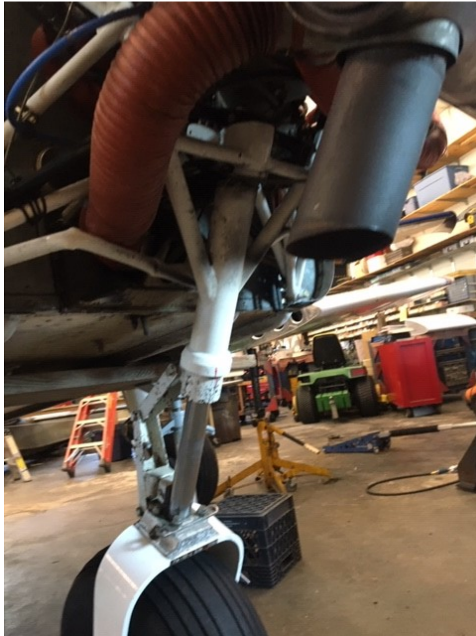
Photo 2 – Accident airplane’s damaged engine mount.
