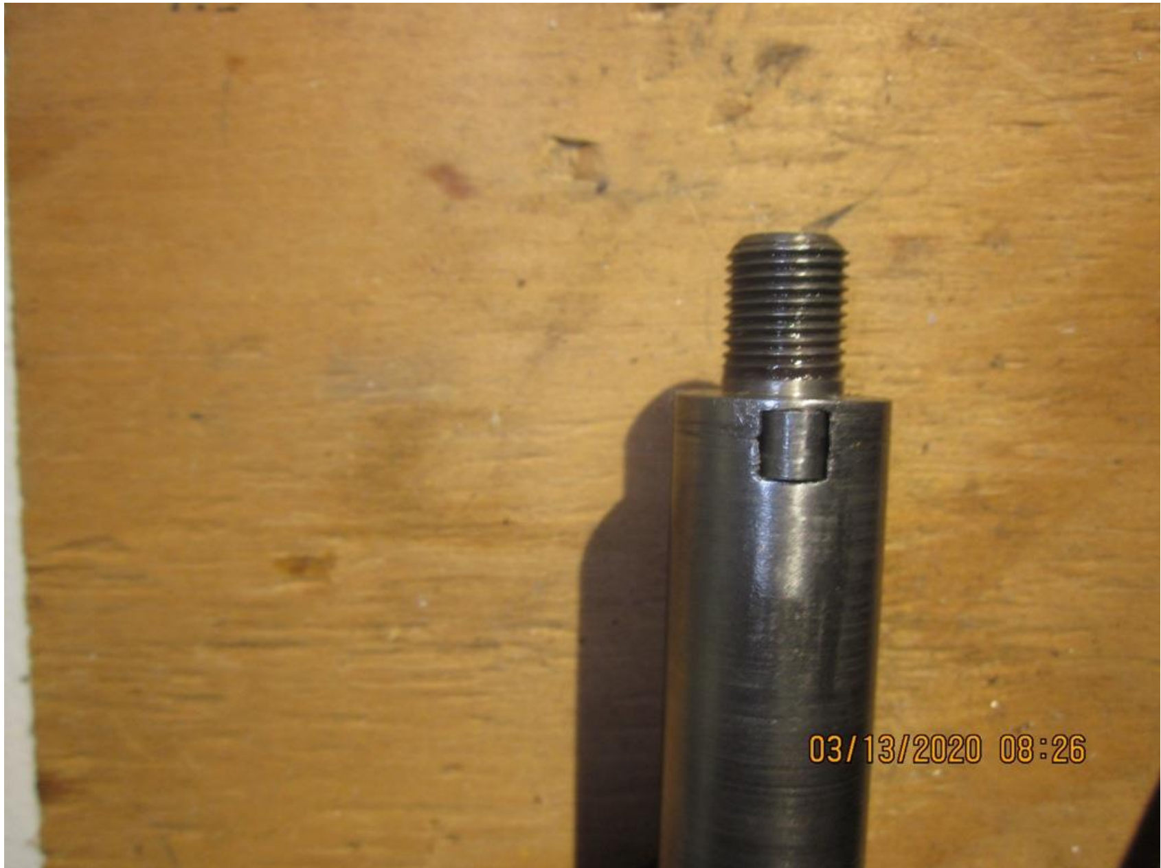
Photo 5 – Tailwheel Fork (Key Slide Stuck Fully Retracted)
