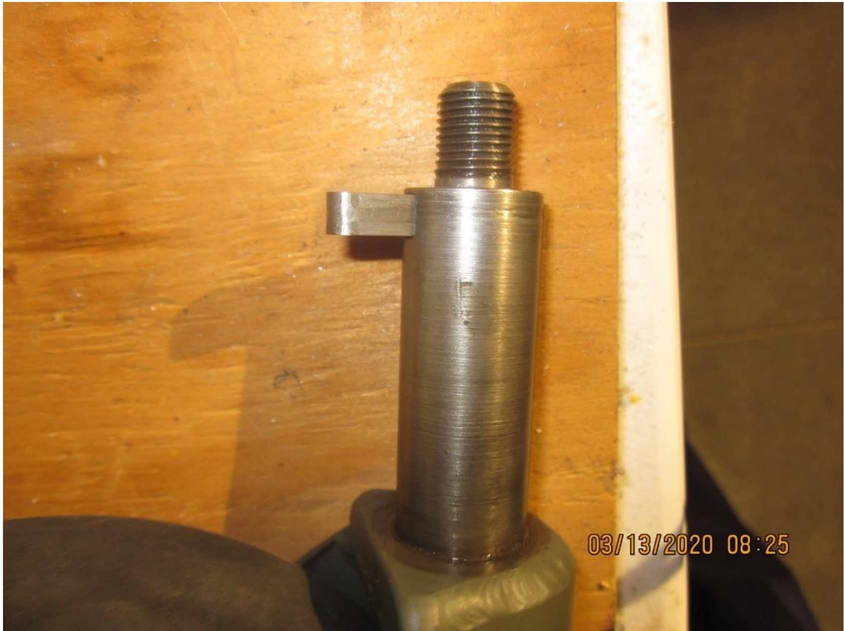
Photo 4 – Tailwheel Fork (Key Slide Fully Extended)
