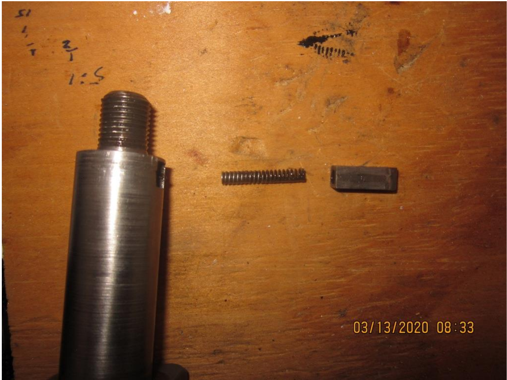
Photo 6 – Tailwheel Fork (Disassembled)
