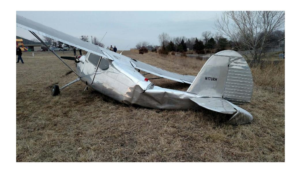
Photo 1 – FAA supplied photo of the left rear quarter of the airplane. The airplane exhibits fuselage damage forward of its empennage.
