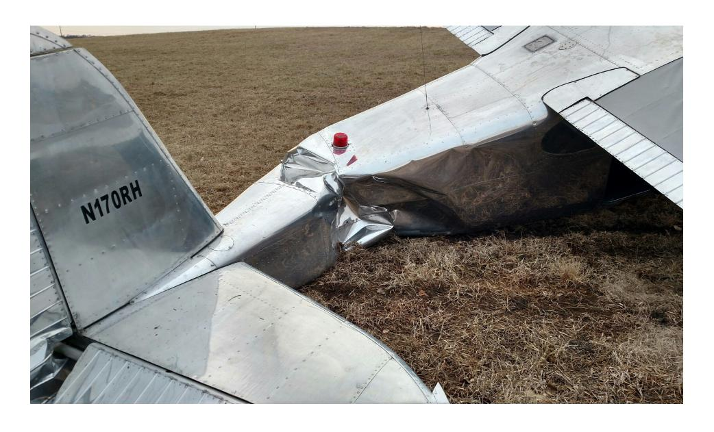
Photo 2 - FAA supplied close up photo of the right rear quarter of the airplane. The airplane exhibits fuselage damage forward of its empennage.
