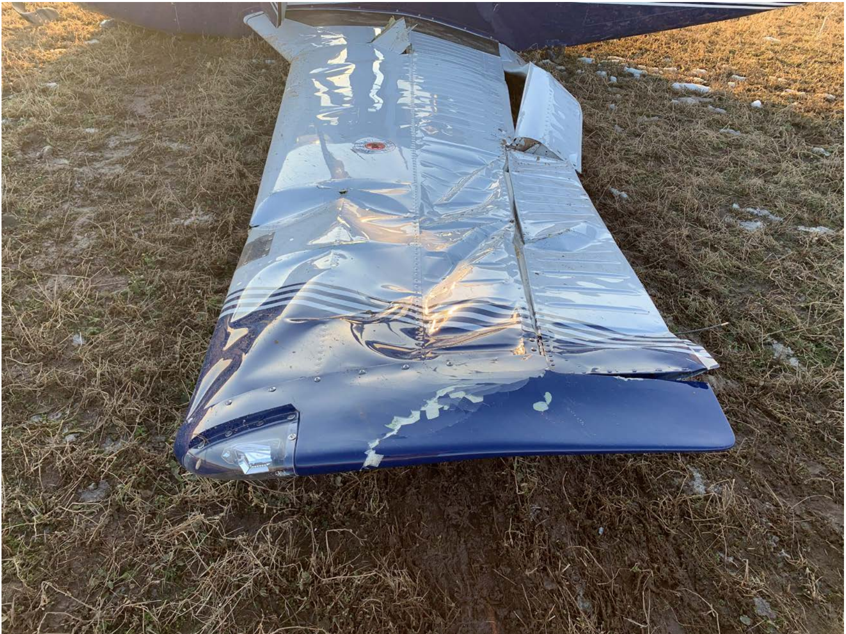
Photo 2 - Damaged and wrinkled left wing
