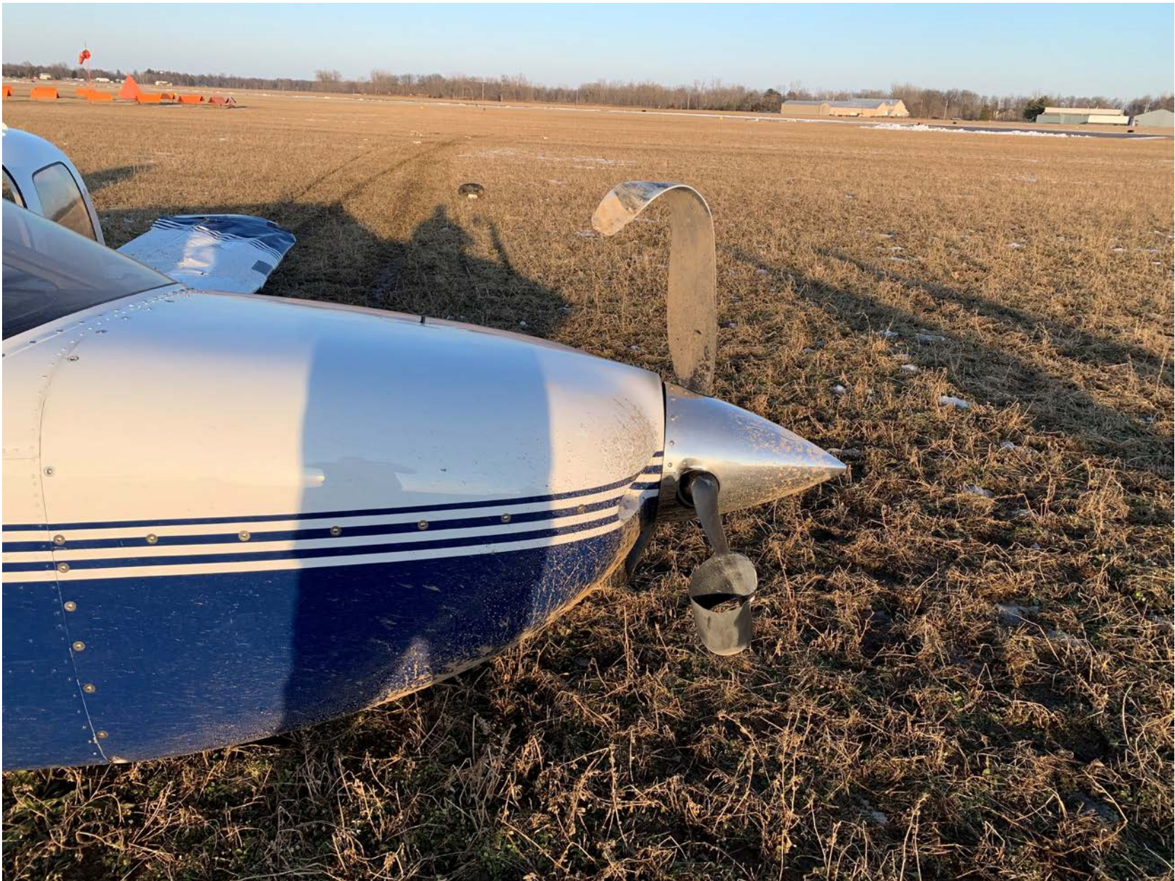
Photo 3 – Damaged and curled propeller blades
