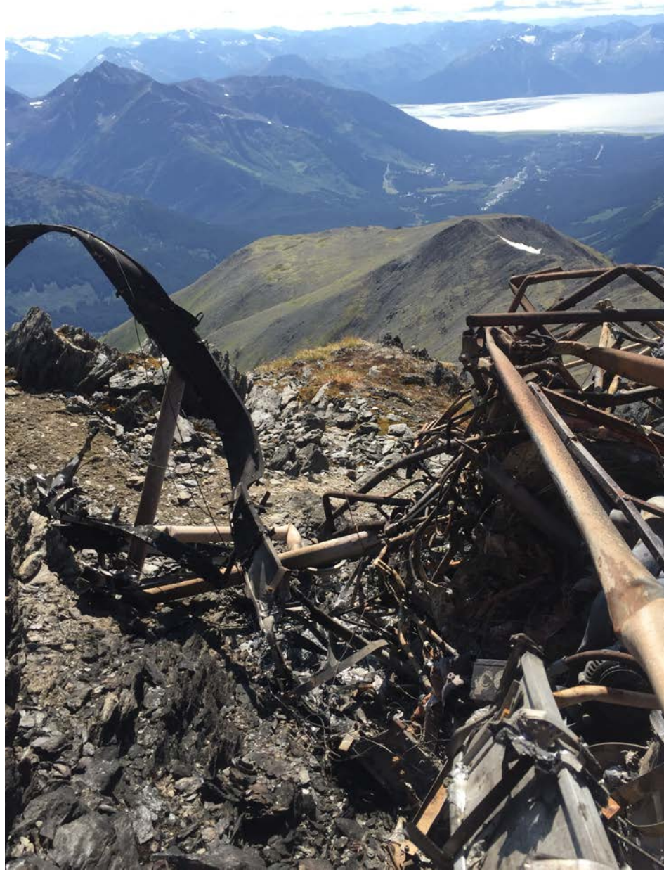
Photo 6 – Thermally damaged accident airplane at accident site looking south towards Girdwood, Alaska.
