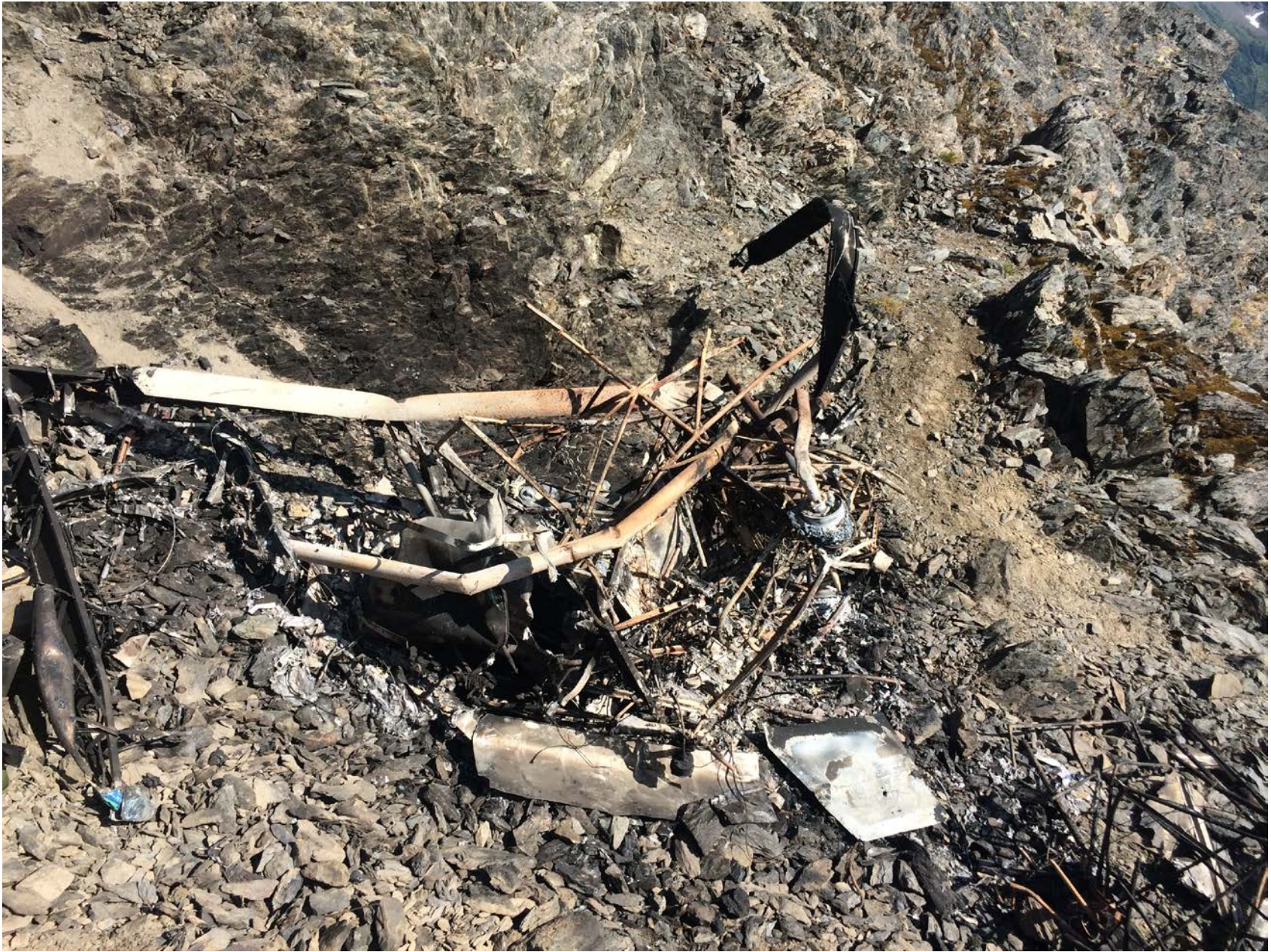
Photo 5 –Thermally damaged accident airplane at accident site.
