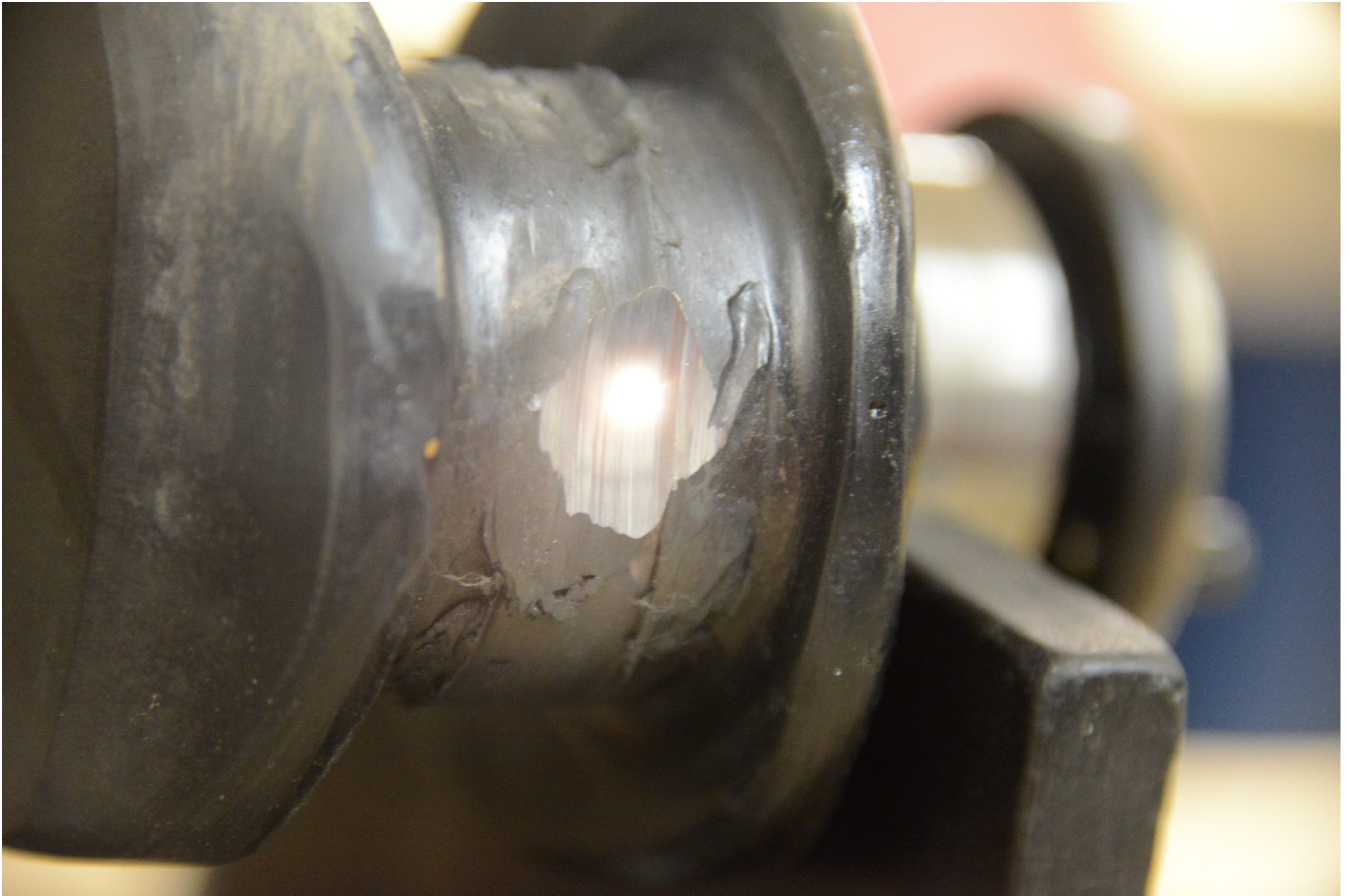
Photo 19 - View of the smeared metal removed over the oil passage on the No. 1 rod end journal. The view shows that the oil passage was not obstructed under the smeared metal..
