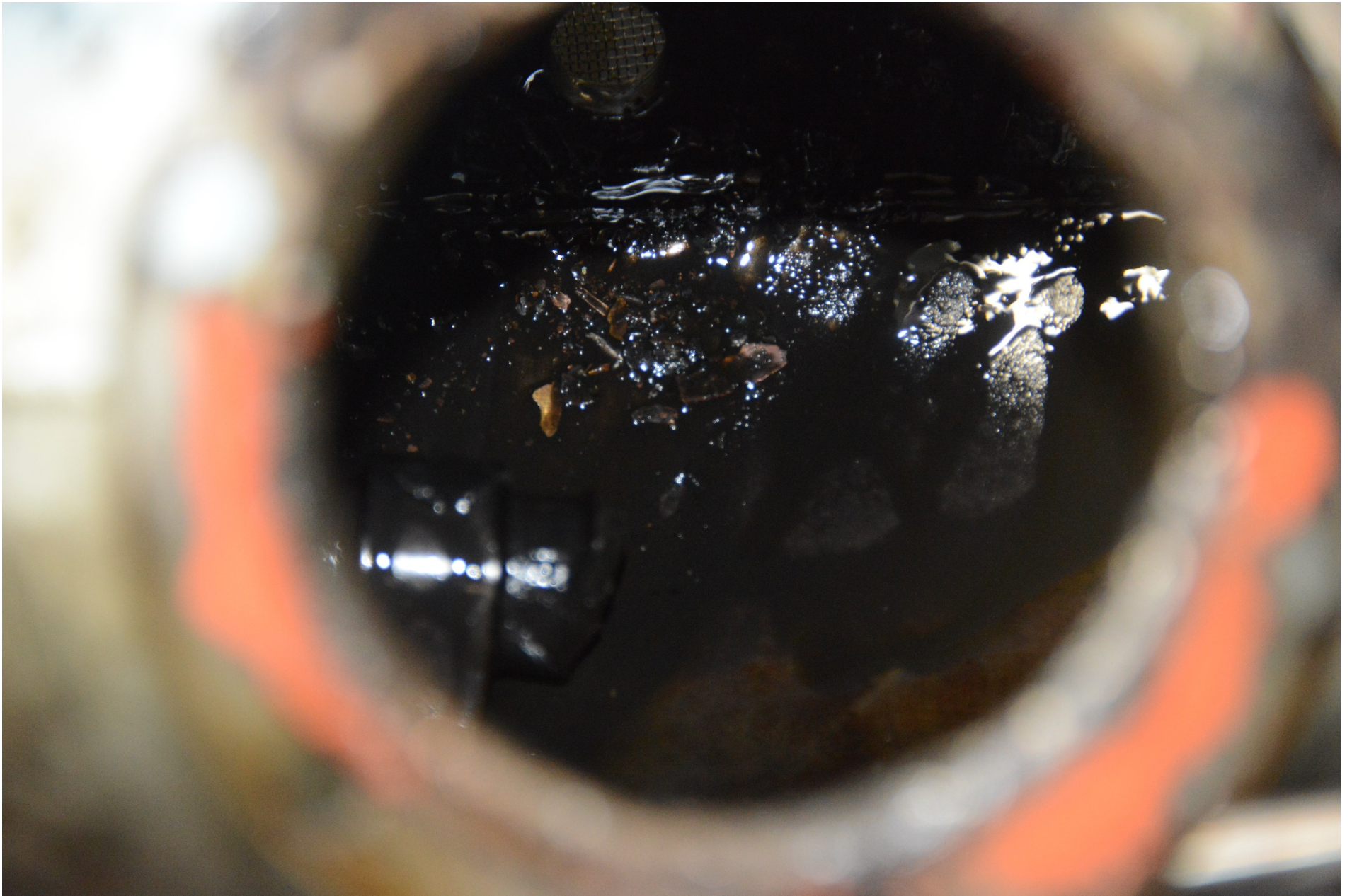
Photo 5 - View inside the oil sump showing debris and a liberated section of camshaft.
