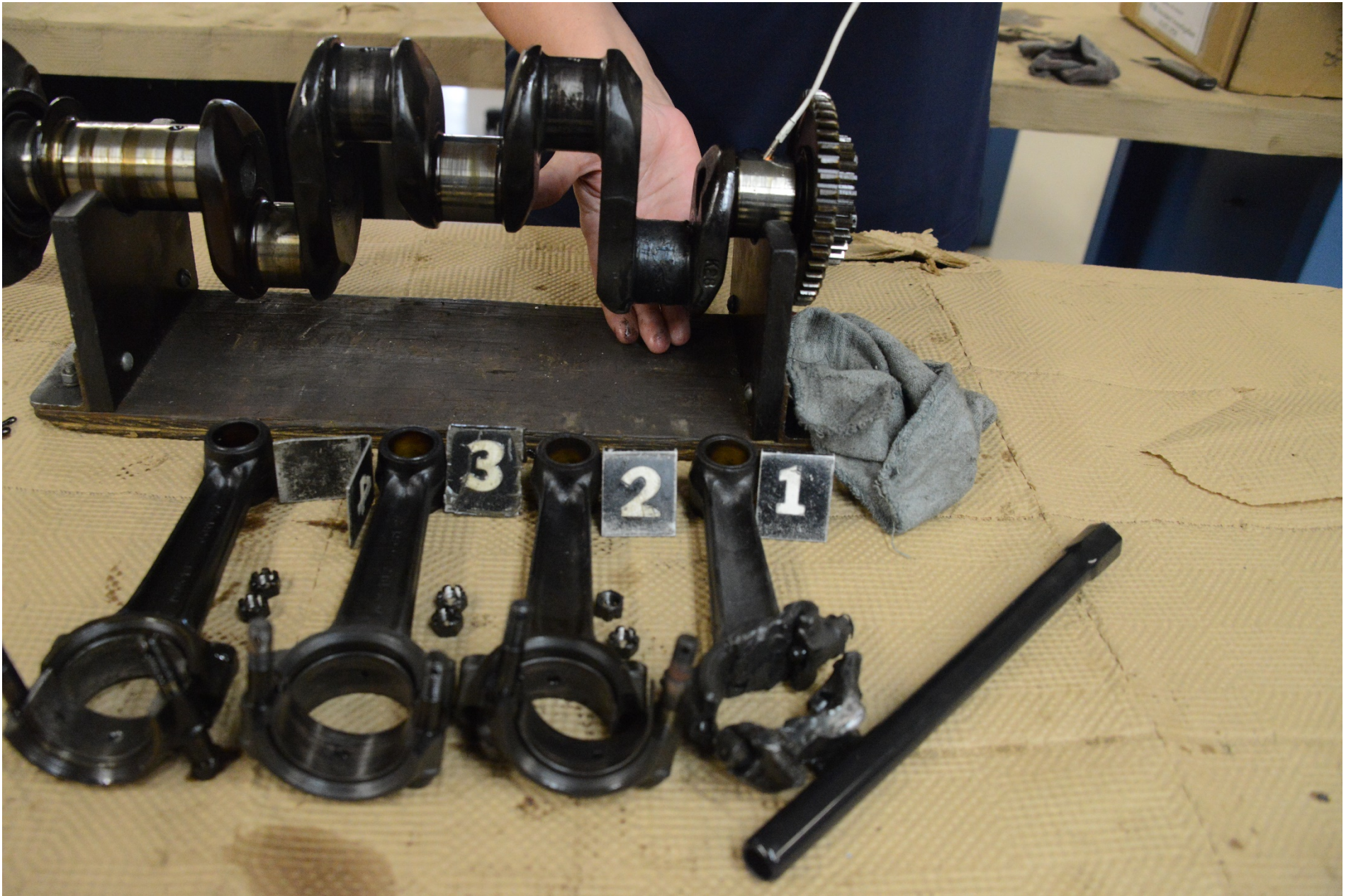
Photo 18 - View of the crankshaft with a light in the oil passage to the No. 1 rod journal. No light can be seen through the journal end of the oil passage.
