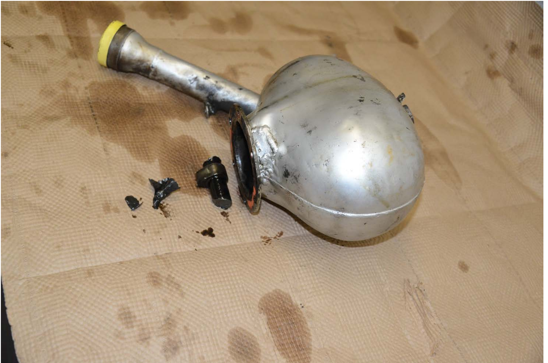
Photo 6 - View of the oil sump, debris. and a liberated section of camshaft.
