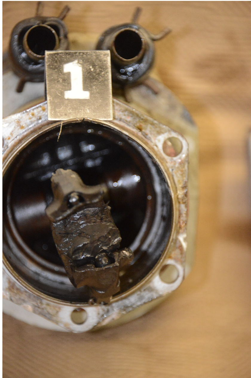
Photo 11 - Close-up view of the No. 1 Cylinder rod end.
