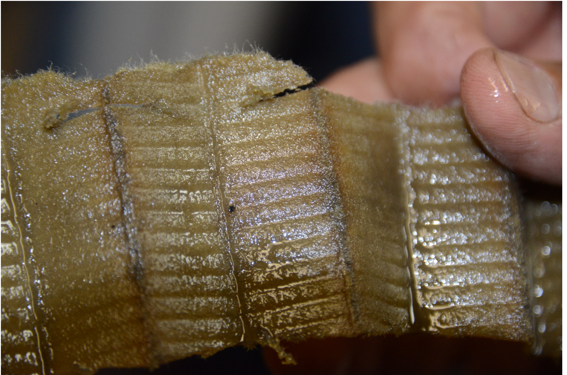
Photo 17 - Opened oil filter element exhibiting one dark colored piece of debris.
