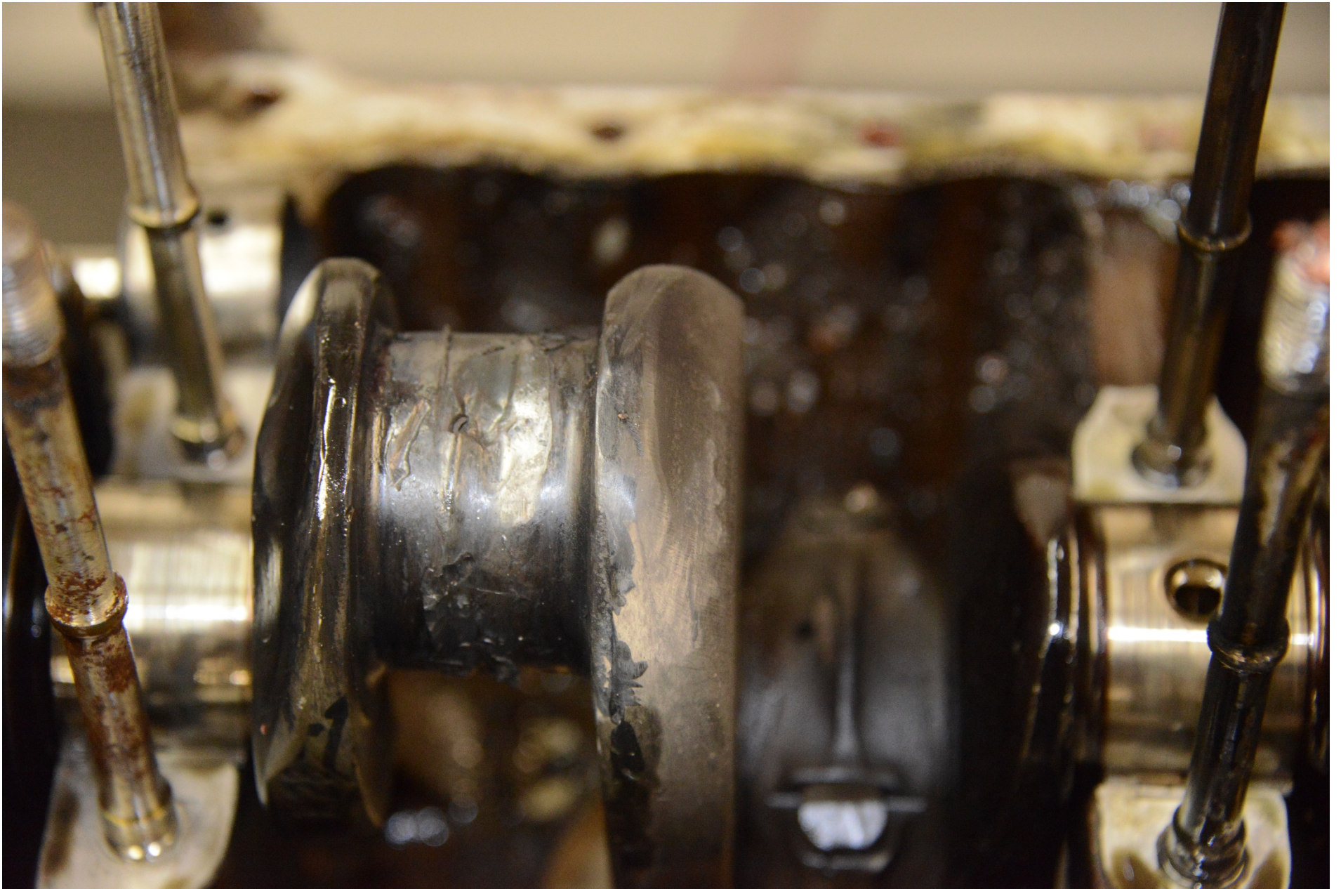
Photo 13 - Close-up view of the No. 1 connecting rod journal. The journal exhibits smeared metal appearance.
