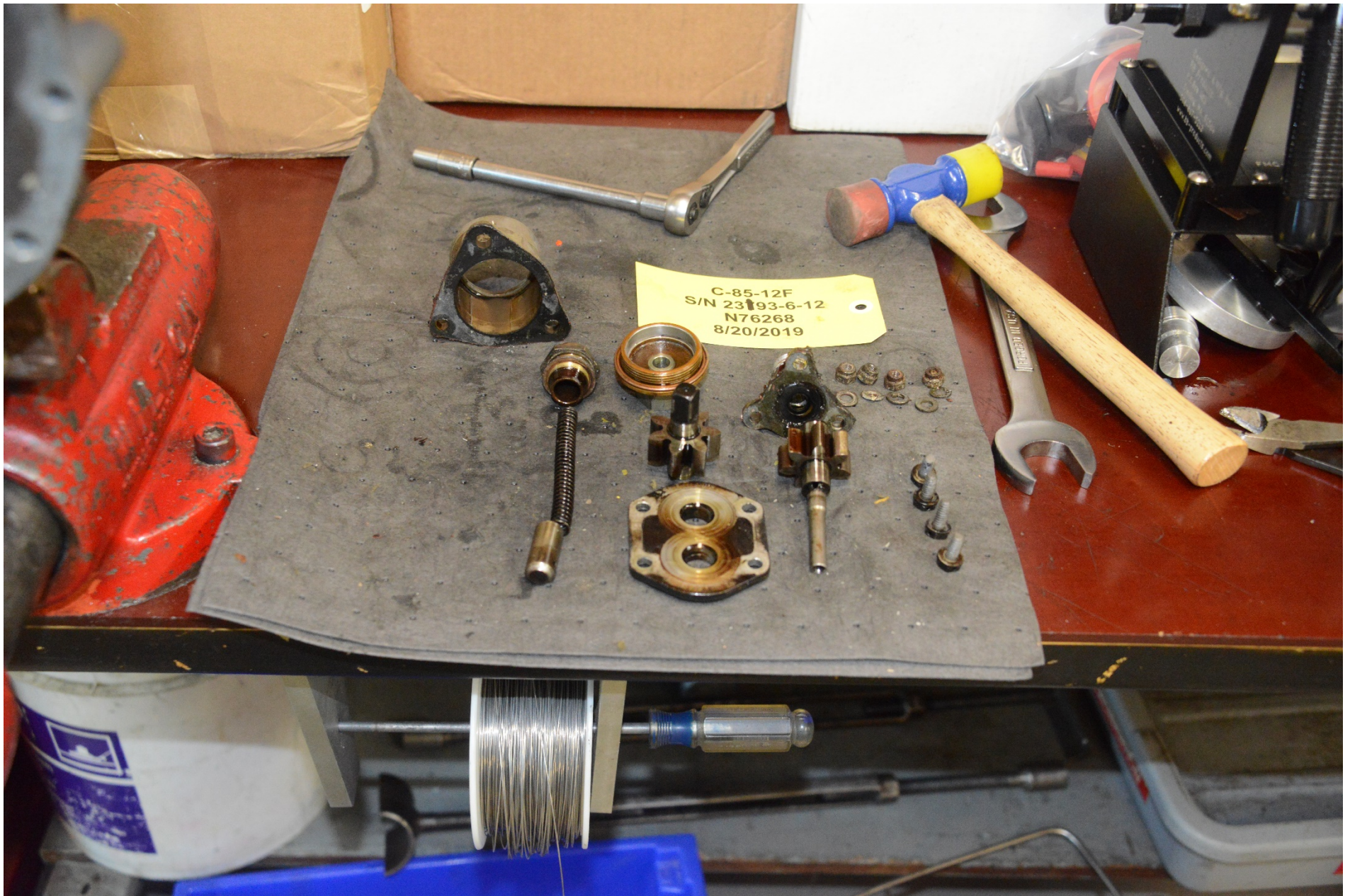
Photo 16 - View of the disassembled oil pump. The pump exhibits scoring consistent with hard particle passage.
