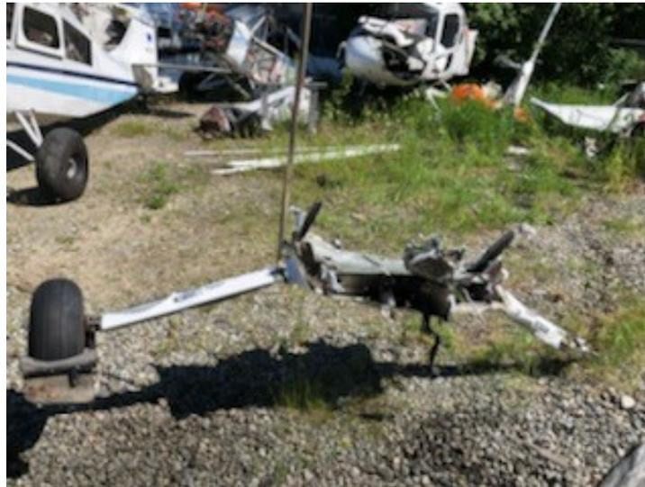
**Photo 4 – Gear box with main gear legs attached from N91038.**
