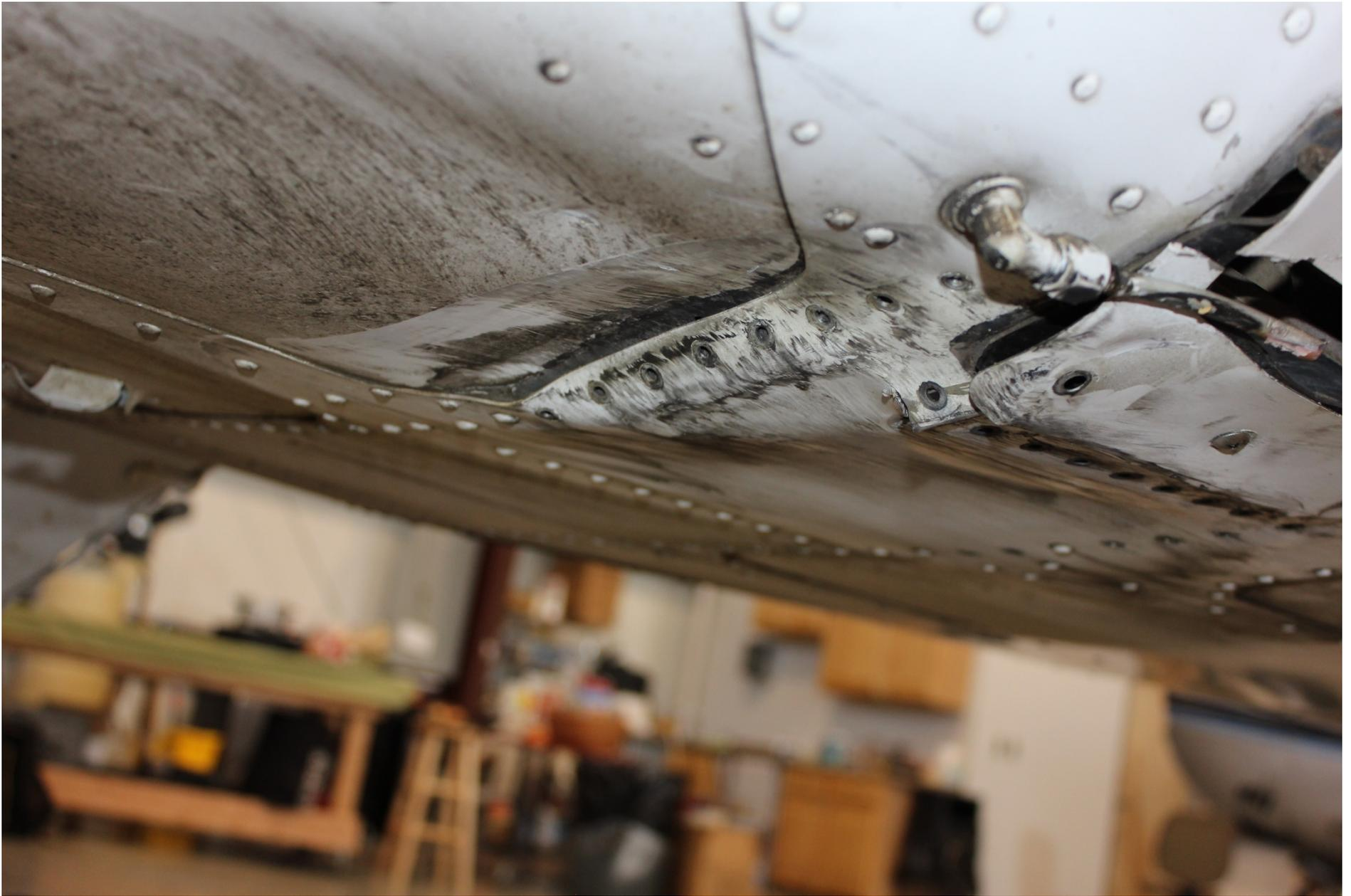
**Photo 10 – Damage to belly of N9423B.**
