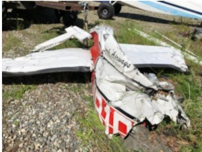
**Photo 3 – Separated empennage from N91038.**
