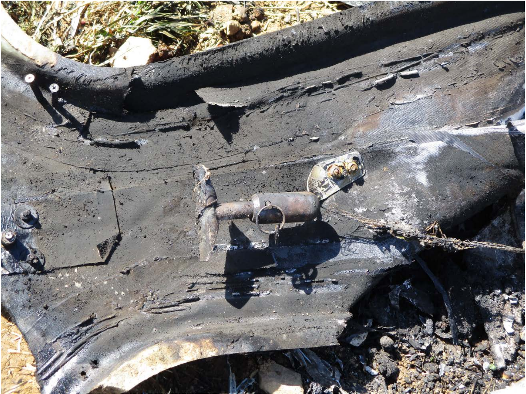
Photo 6 – C-APC T-handle with safety pin installed
