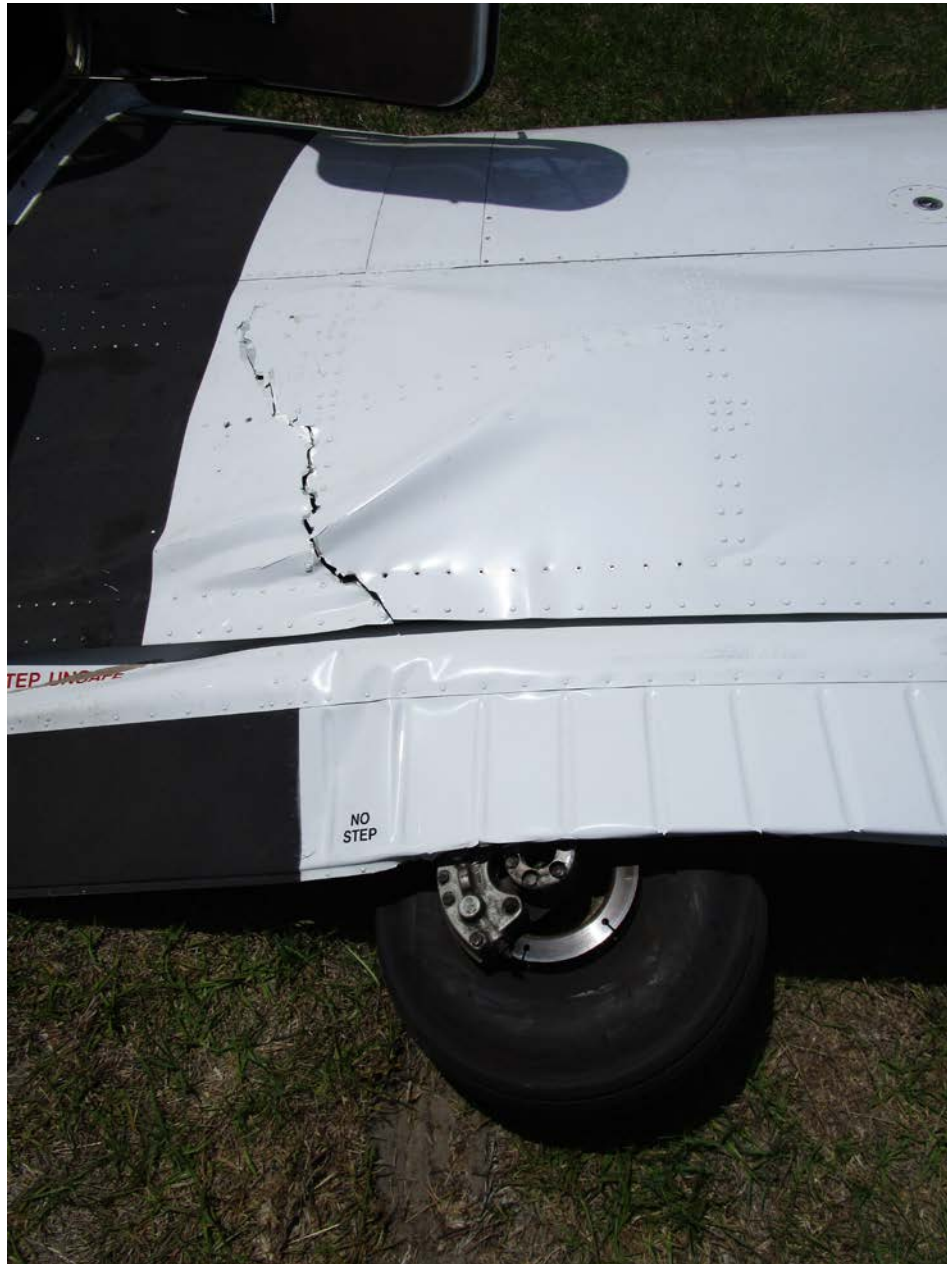
Photo 2 – View of damage to the right wing (Courtesy of Operator)
