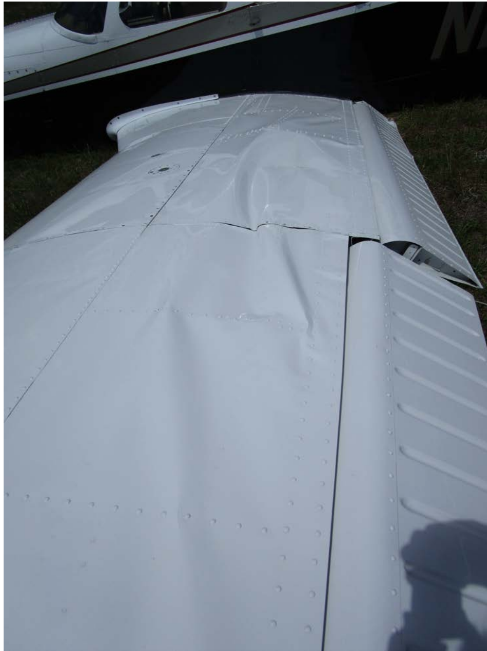
Photo 1 – View of damage to the left wing (Courtesy of Operator)
