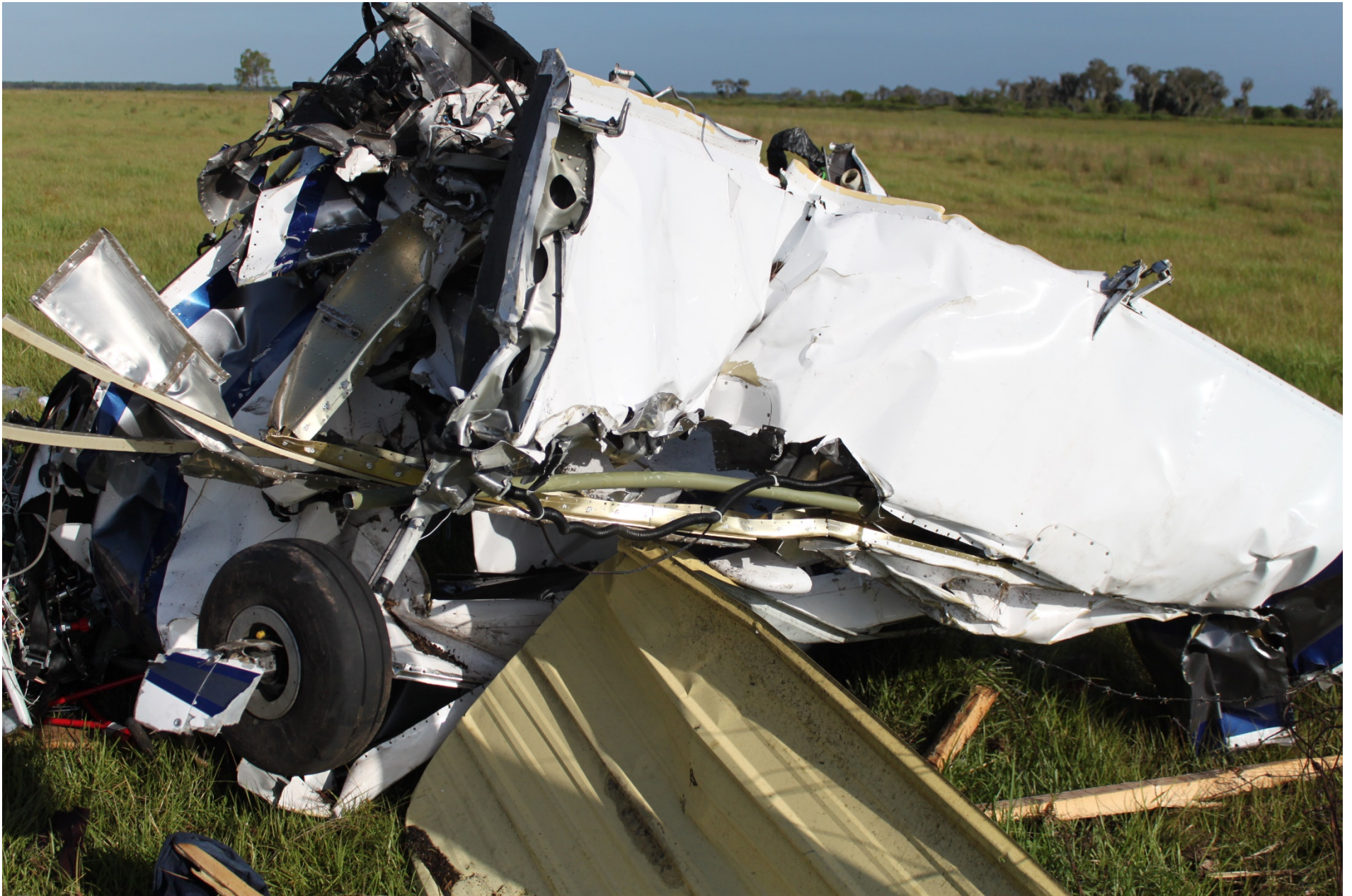
Photo 4 – View of fuselage and part of wing crushed.
