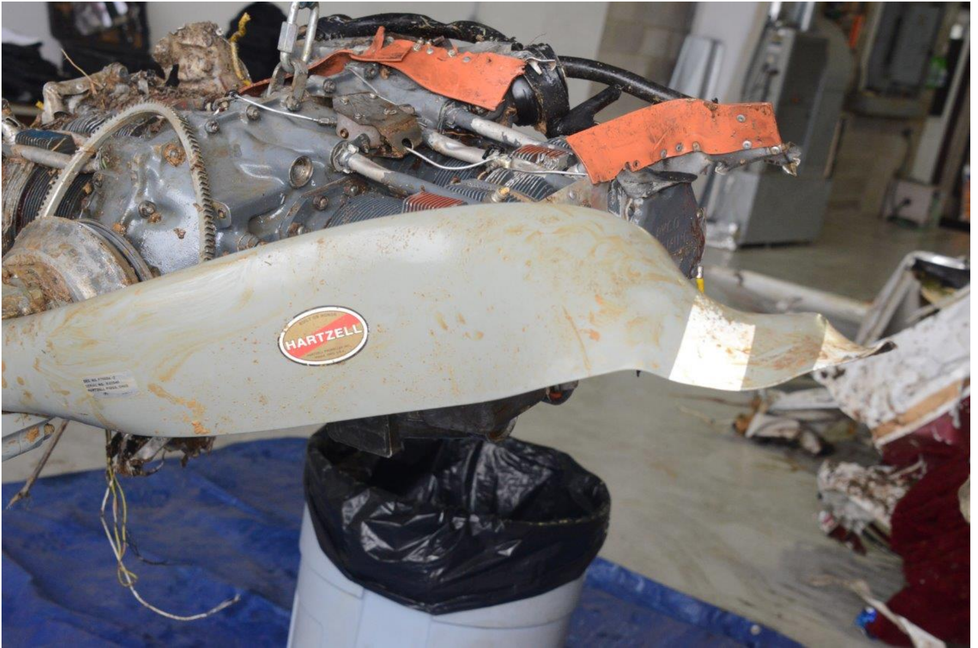
Photo 13 - View of a propeller blade marked no.1 with S shaped bending.
