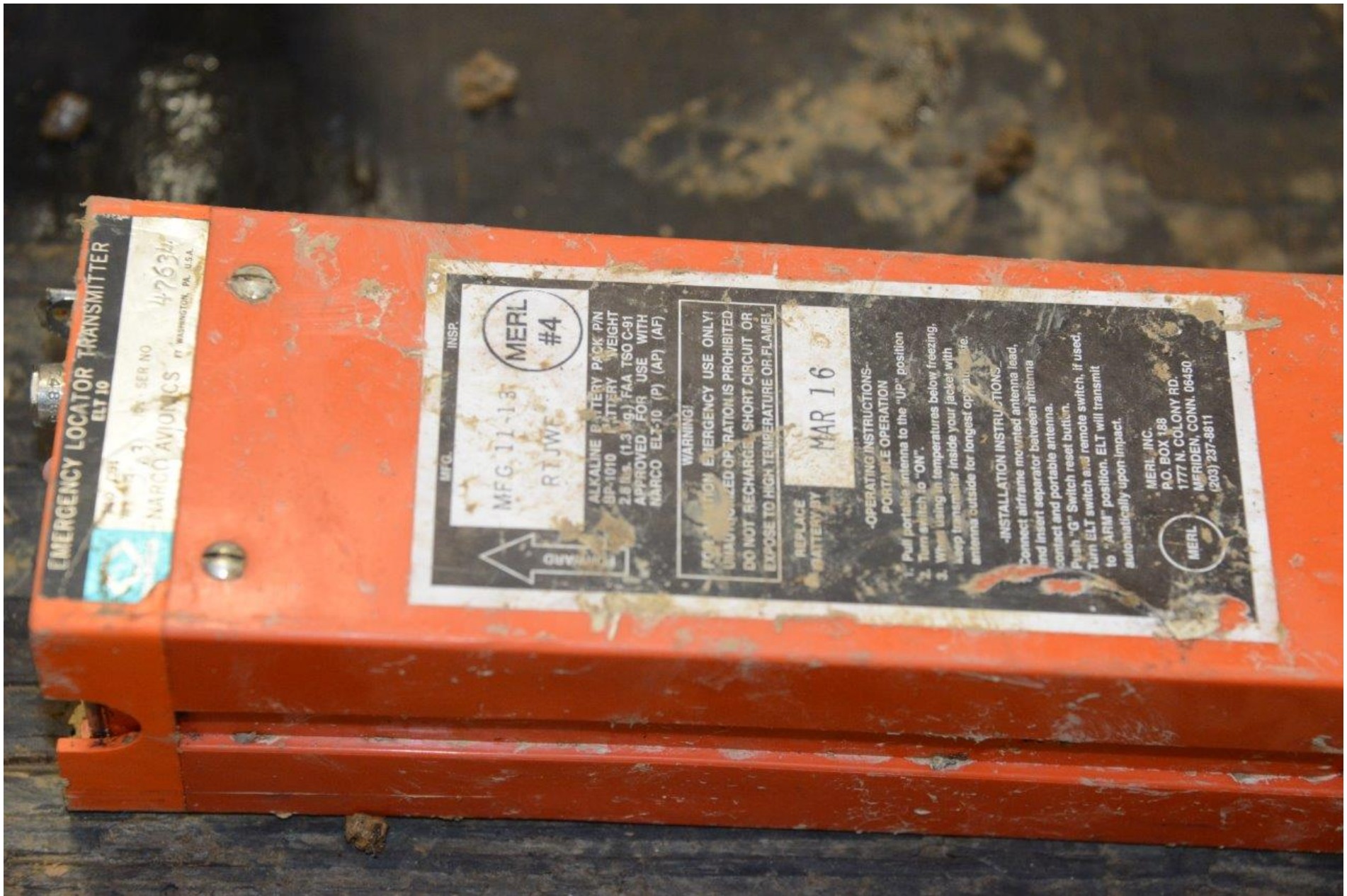
Photo 17 - View of the emergency locator transmitter.
