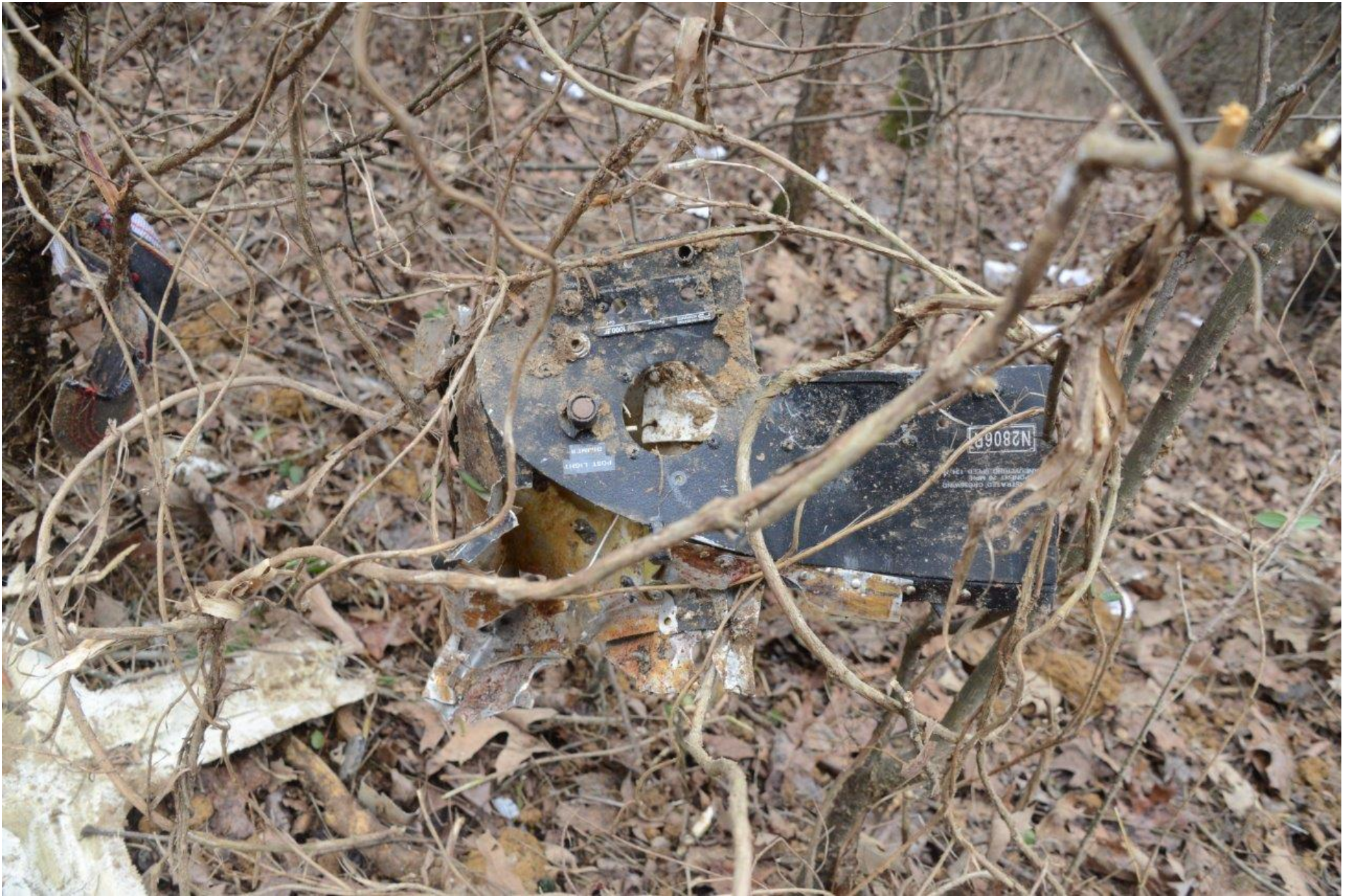
Photo 8 - View of a section of the instrument panel in the debris path.
