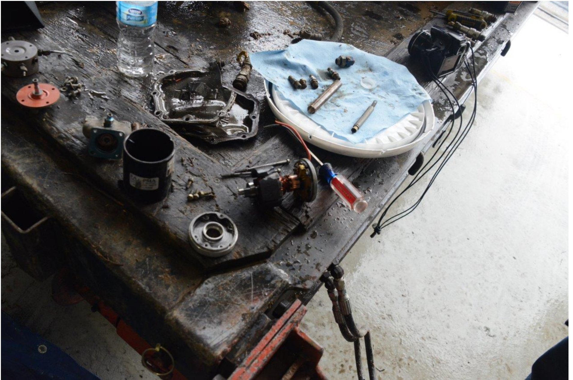
Photo 15 - View of fuel servo filter, disassembled electric fuel pump, and disassembled fuel divider.
