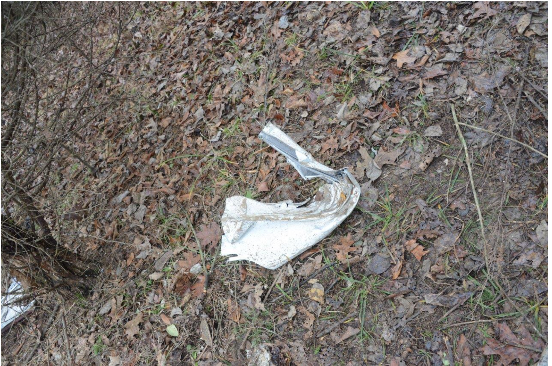
Photo 12 - View of a section of airplane skin with a semicircular deformation.
