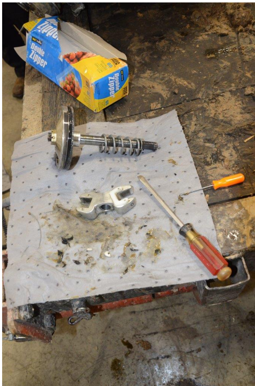
Photo 18 - View of the propeller piston, pitch change rod, spring, and pitch change fork.
