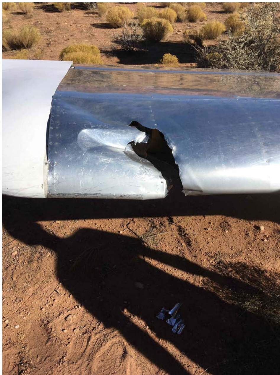
Photo 1 – View of damage to the right wing leading edge and ribs (Courtesy of FAA) □
