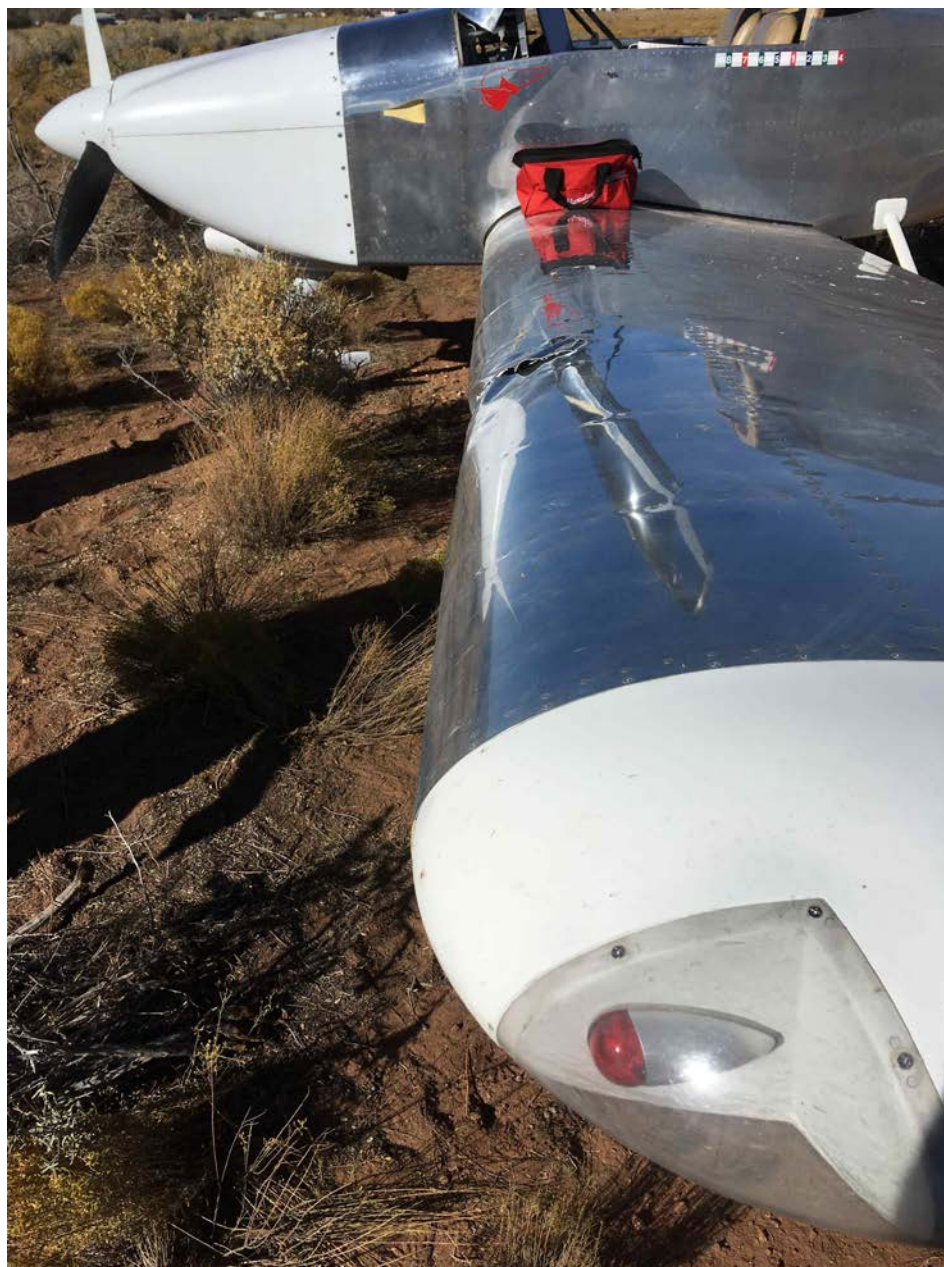
Photo 2 – View of damage to the left wing leading edge and ribs (Courtesy of FAA)
