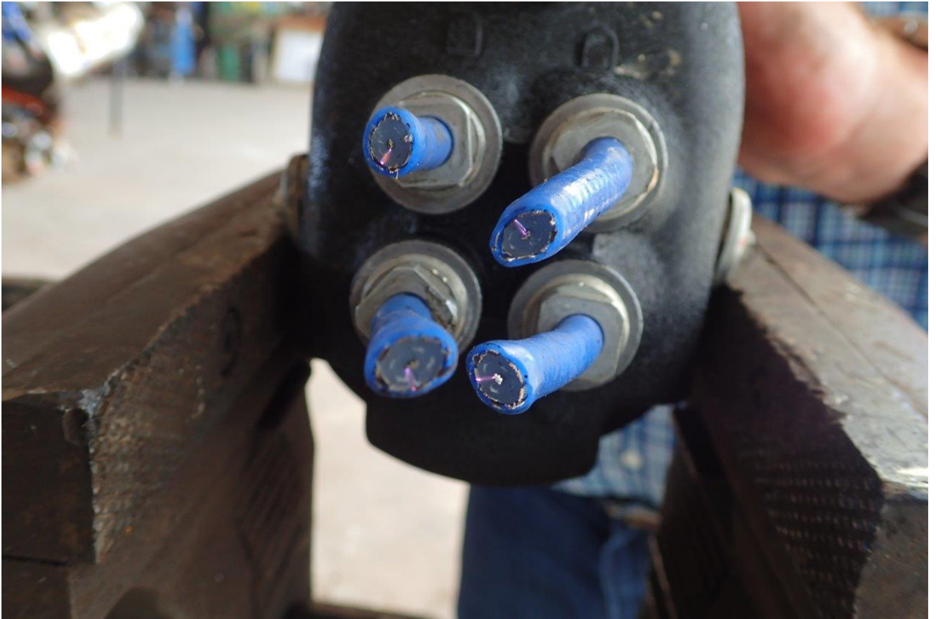
Photo 7 - View of a magneto exhibiting spark at all leads.
