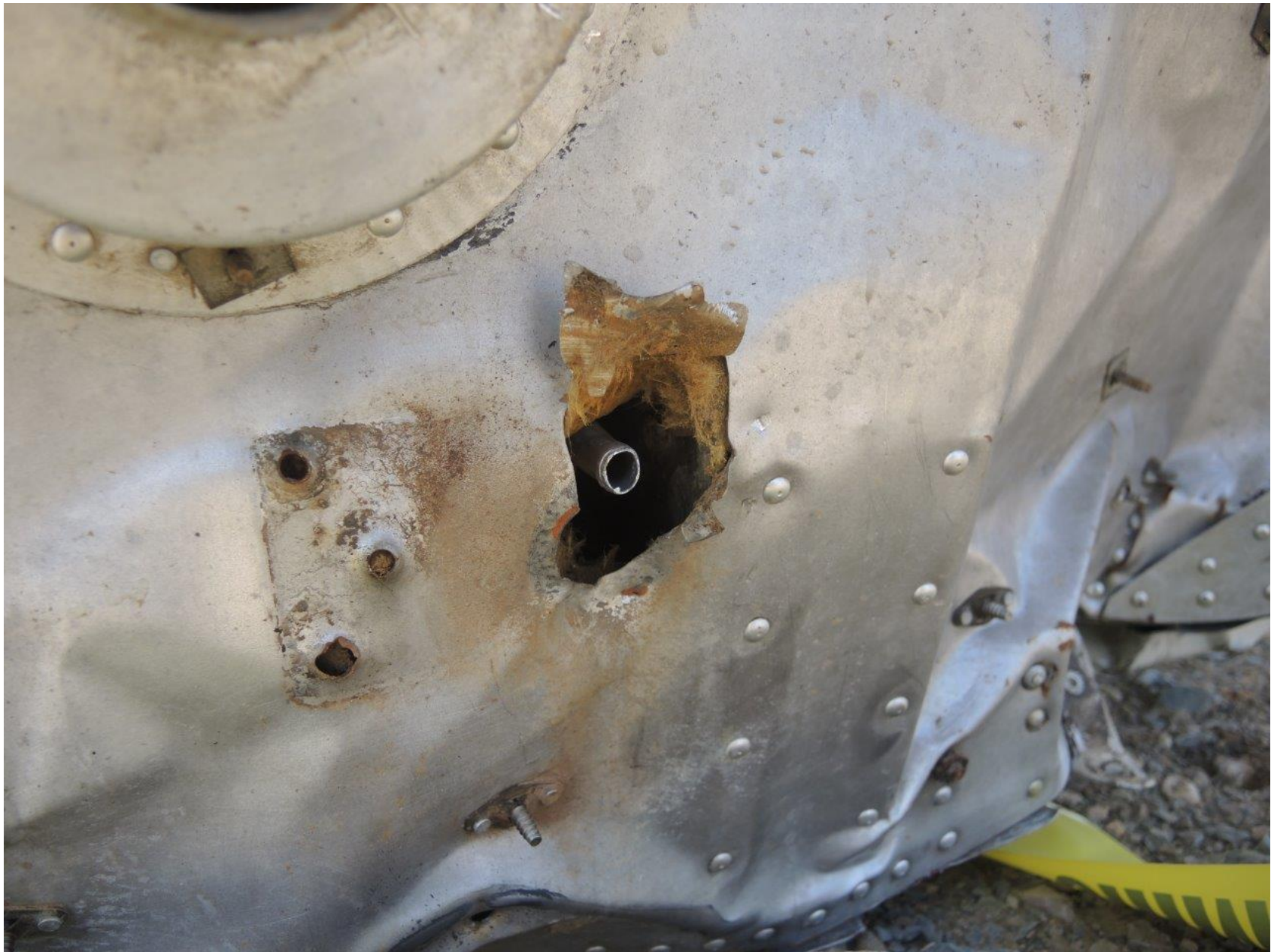
Photo 5 - View of the fuel line where pressurized air was applied.
