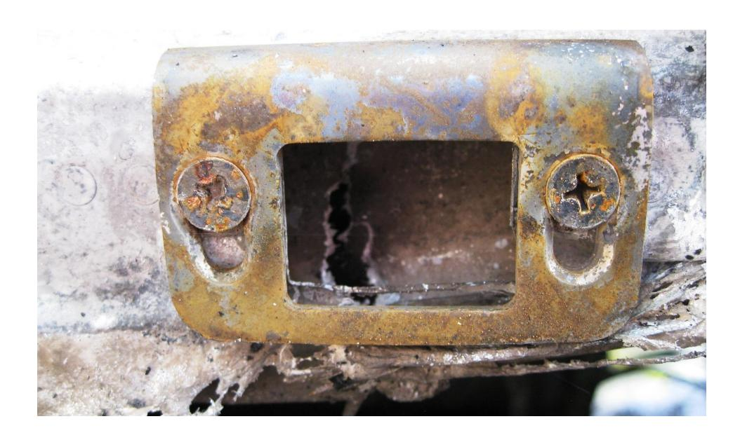
**Photo 11 - Forward Baggage Door Frame Latch Catch/Receptacle**
