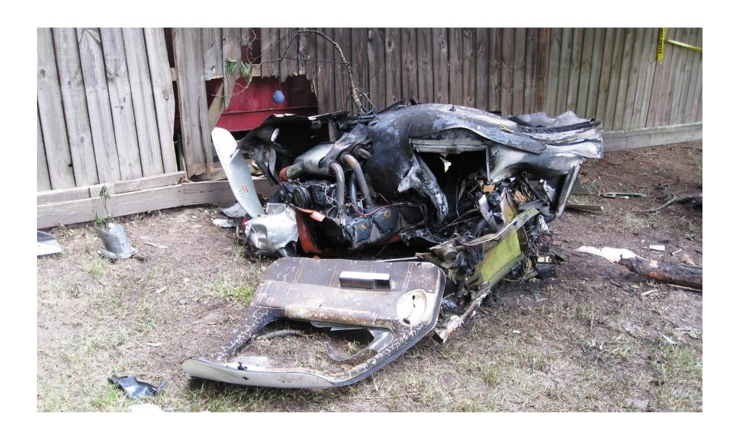
Photo 5 - Engine, Propeller, Forward Fuselage, and Main Cabin Door
