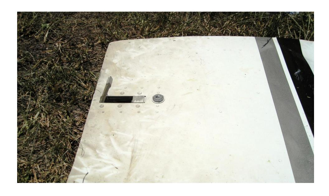
**Photo 9 - Forward Baggage Compartment Door Latch and Key-Lock (External)**
