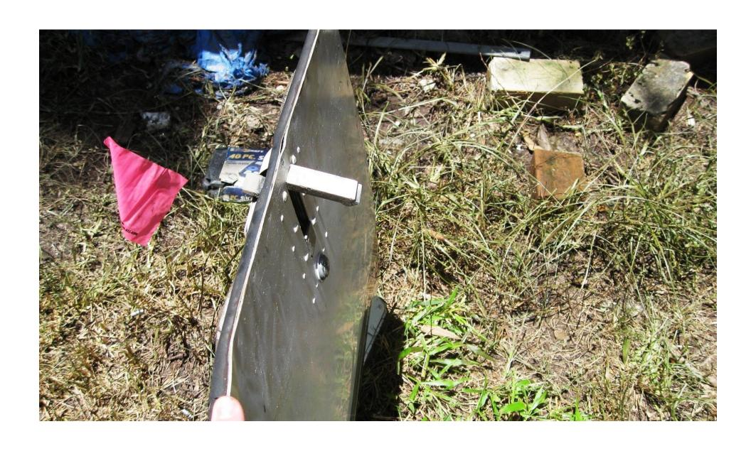
**Photo 8 - Forward Baggage Compartment Door Latch**
