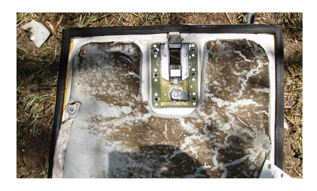
**Photo 10 - Forward Baggage Compartment Door Latch and Key-Lock Assembly (Internal)**
