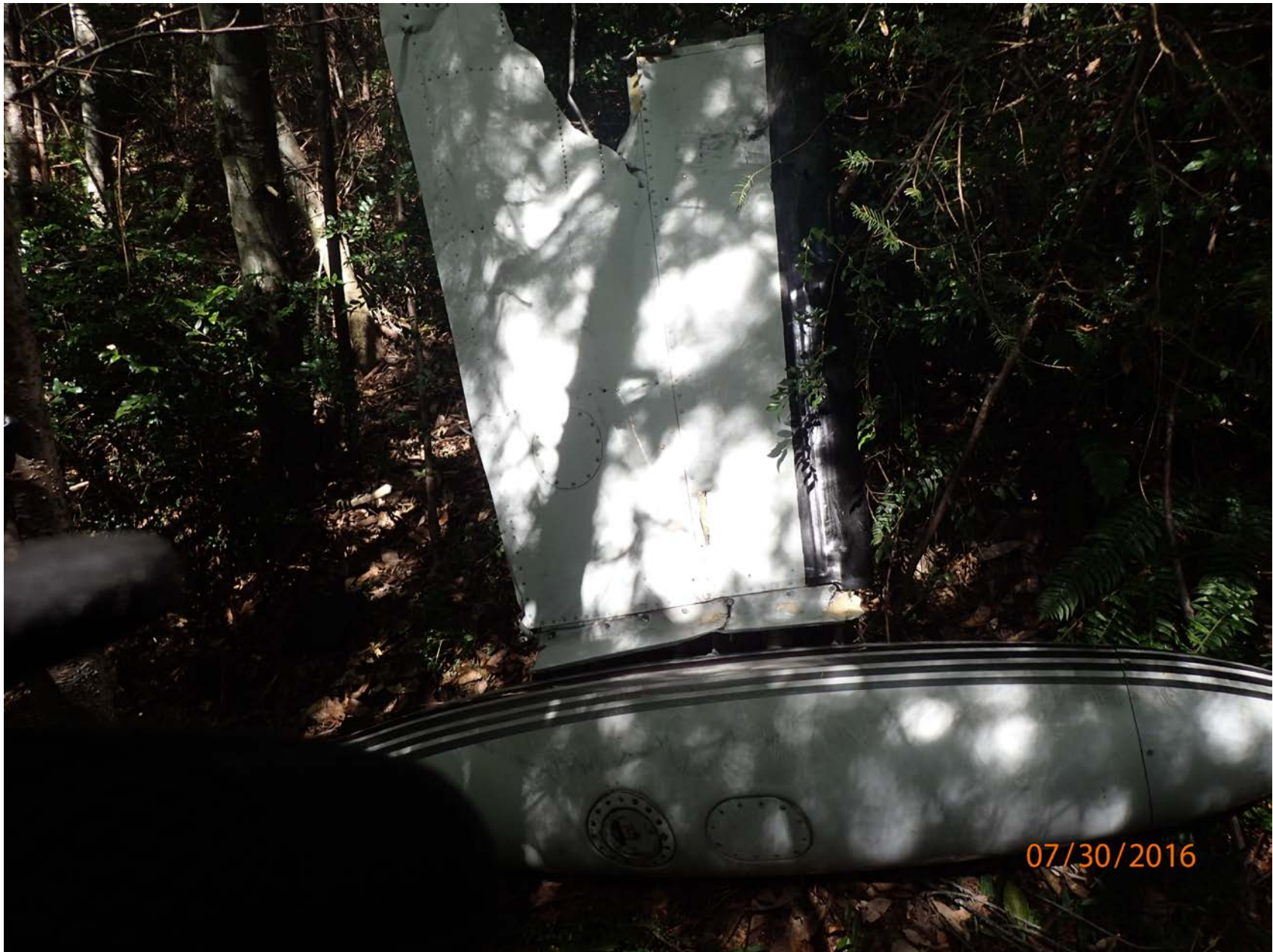
Photo 5 – Right outboard wing section at accident site.
