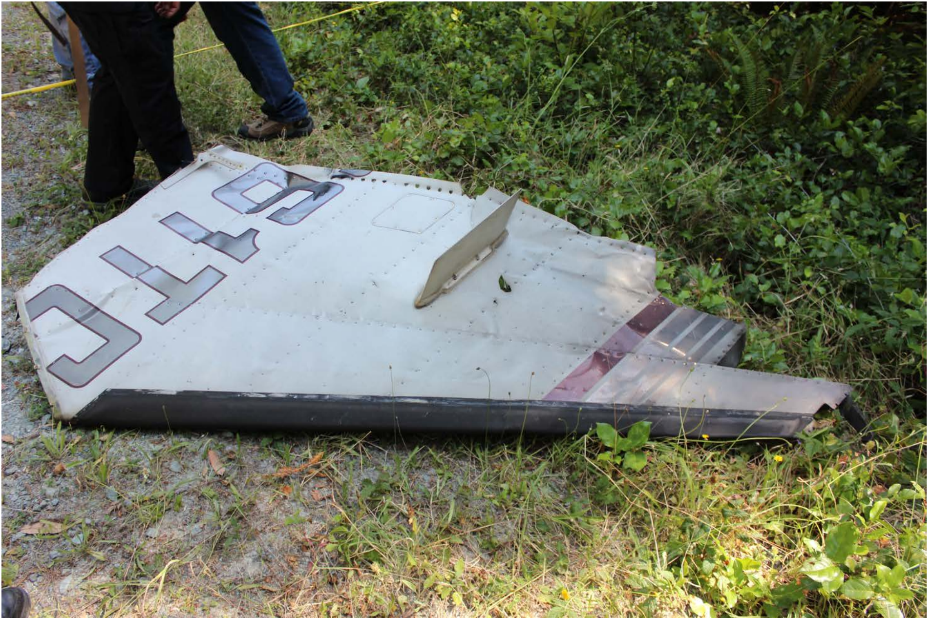
Photo 6 – Vertical stabilizer at accident site.
