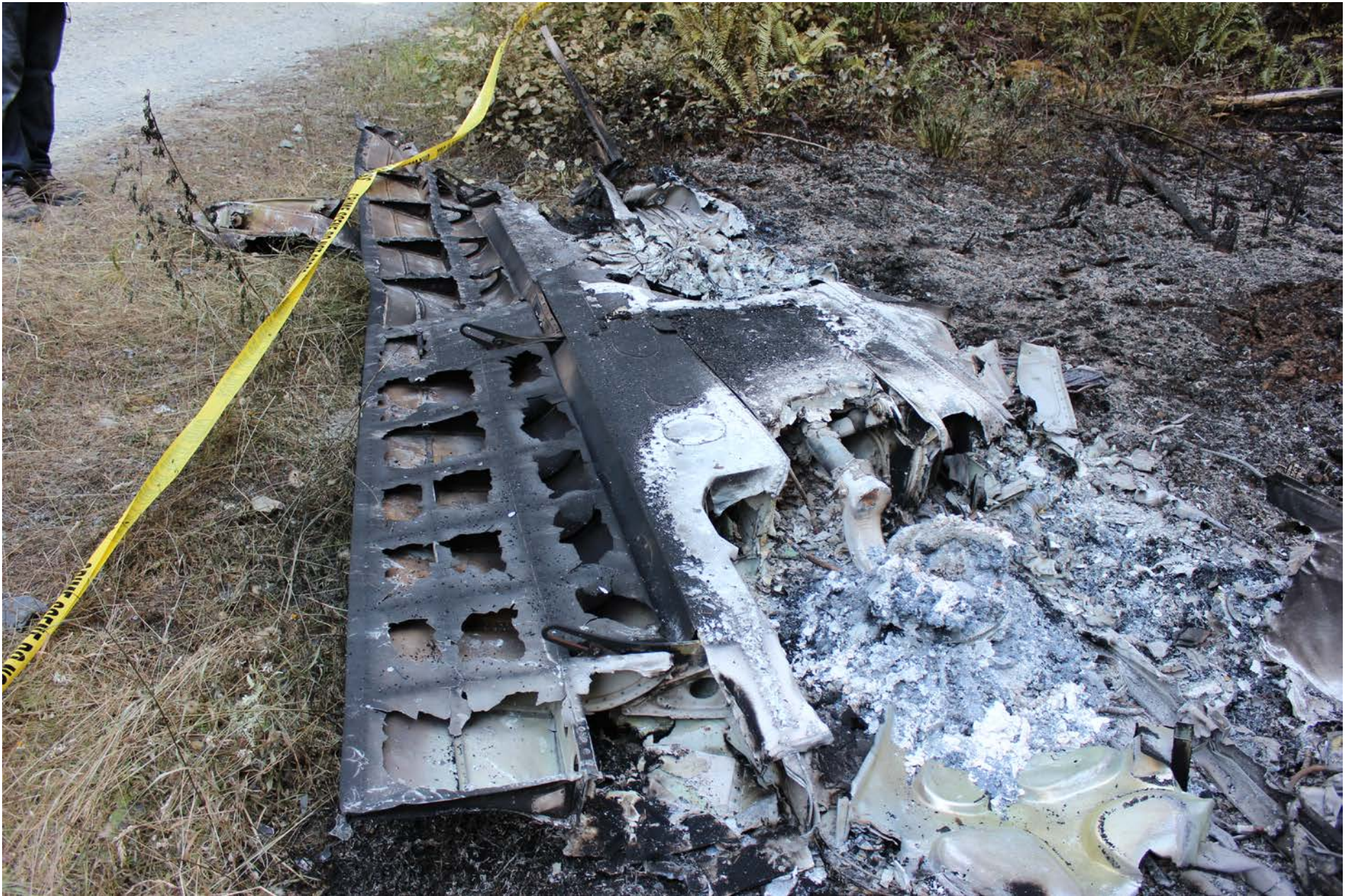
Photo 3 – Right inboard wing section at accident site.
