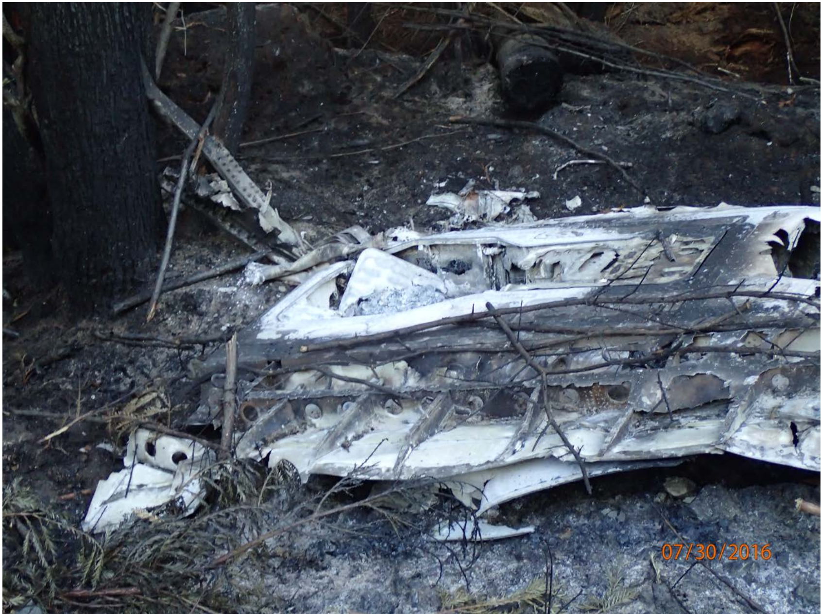
Photo 2 – Left inboard wing section at accident site.
