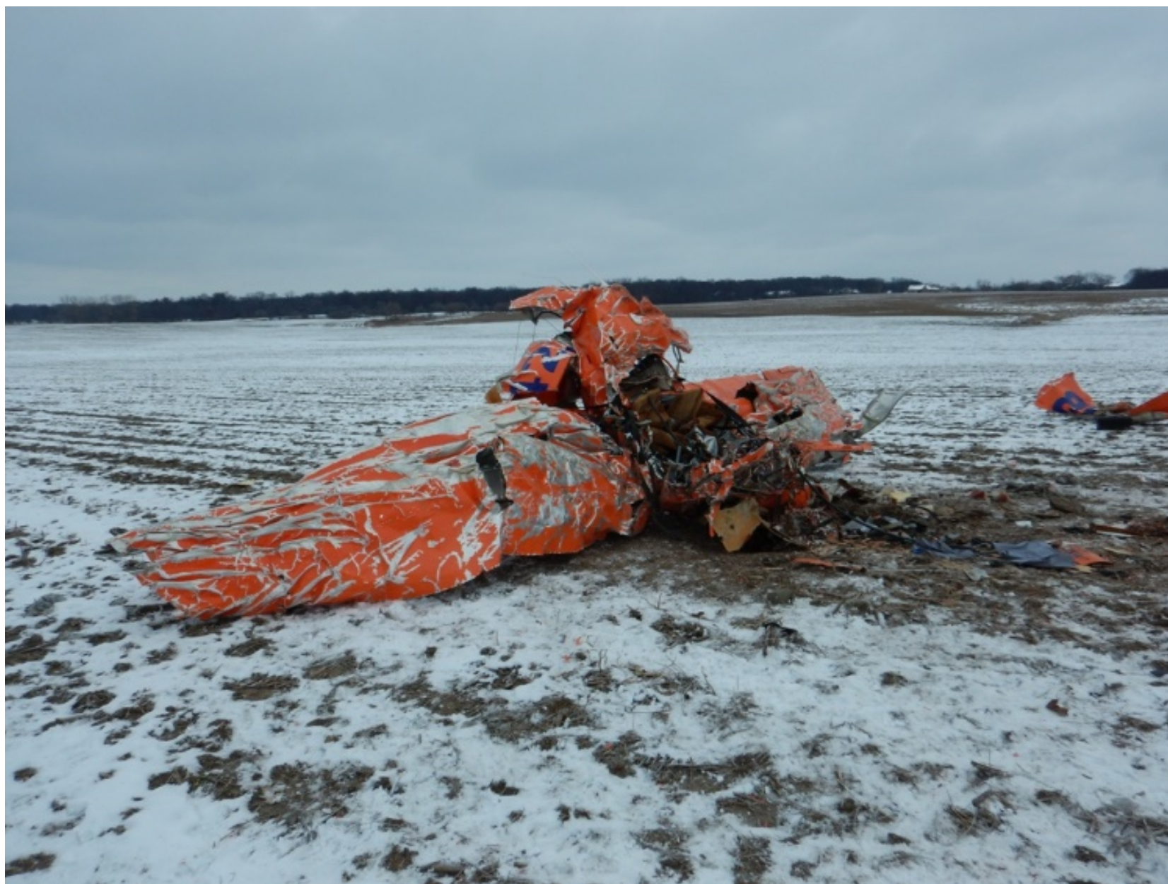
Photo 5 – Right wing after wreckage was up righted.
