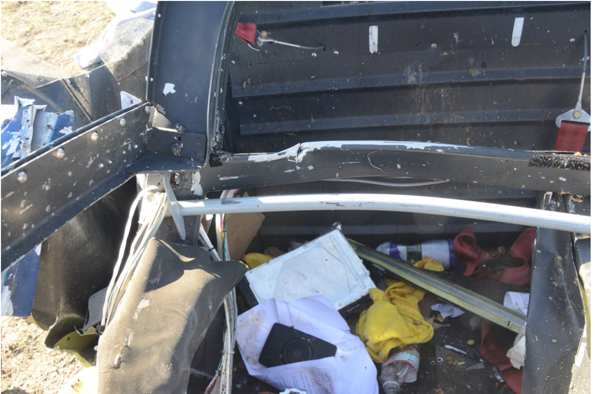
Photo 10 - View of a section of the canopy latch assembly.
