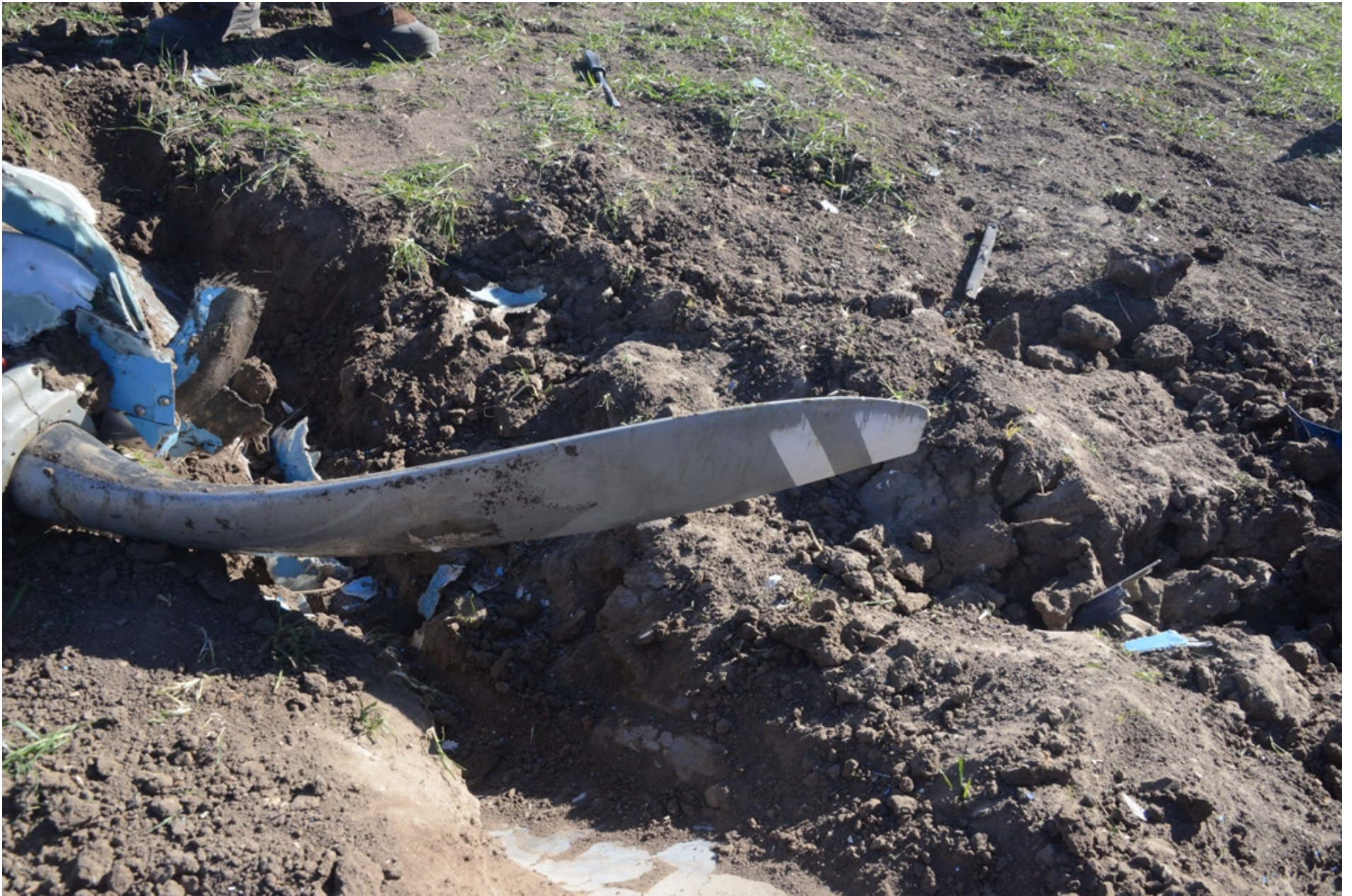
Photo 7 - View of abrasion on a propeller blade.
