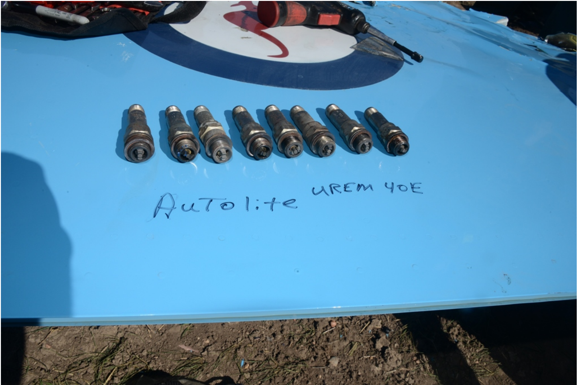
Photo 15 - View of removed sparkplugs.
