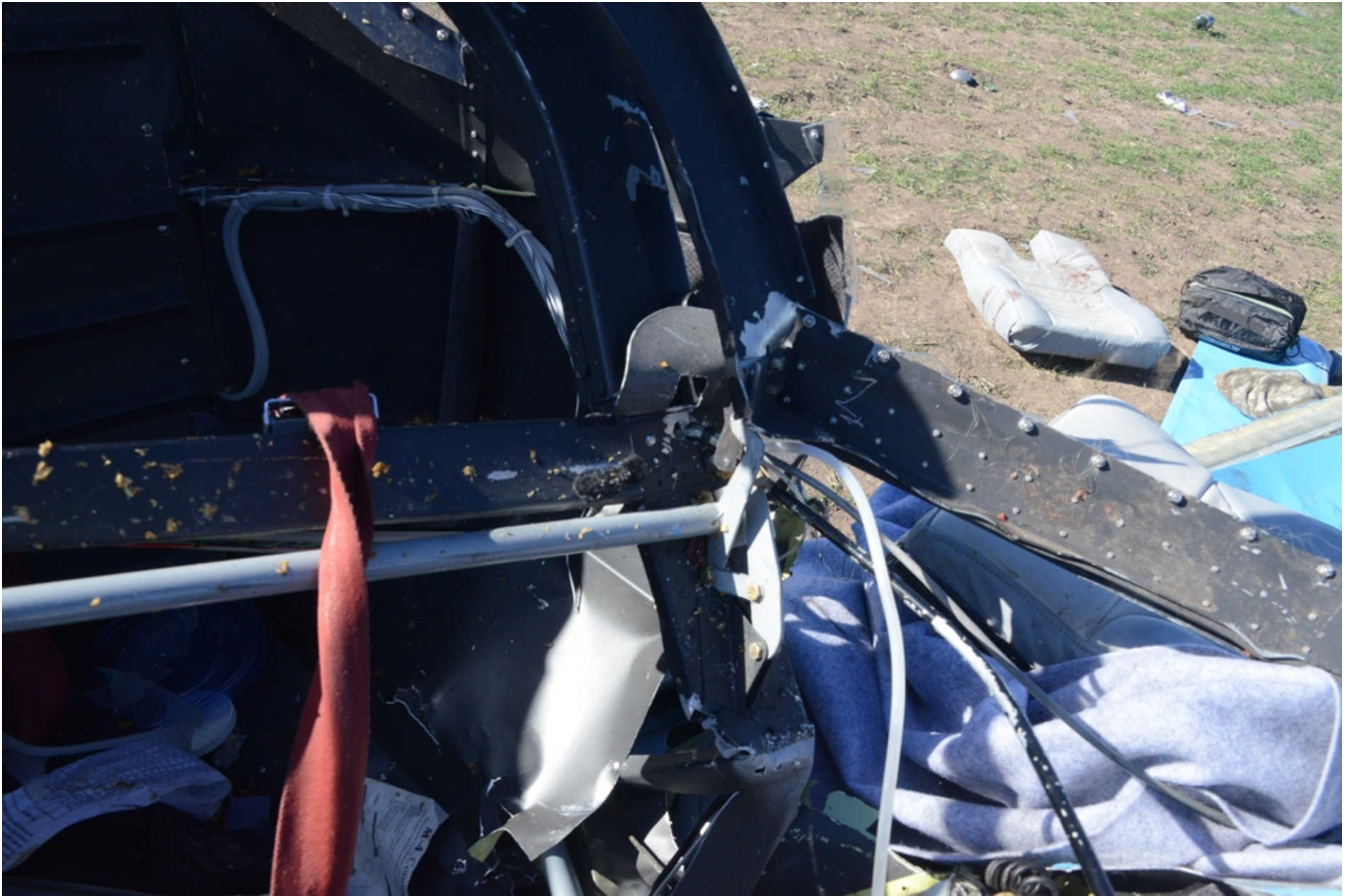
Photo 9 - View of a section of the canopy latch assembly.
