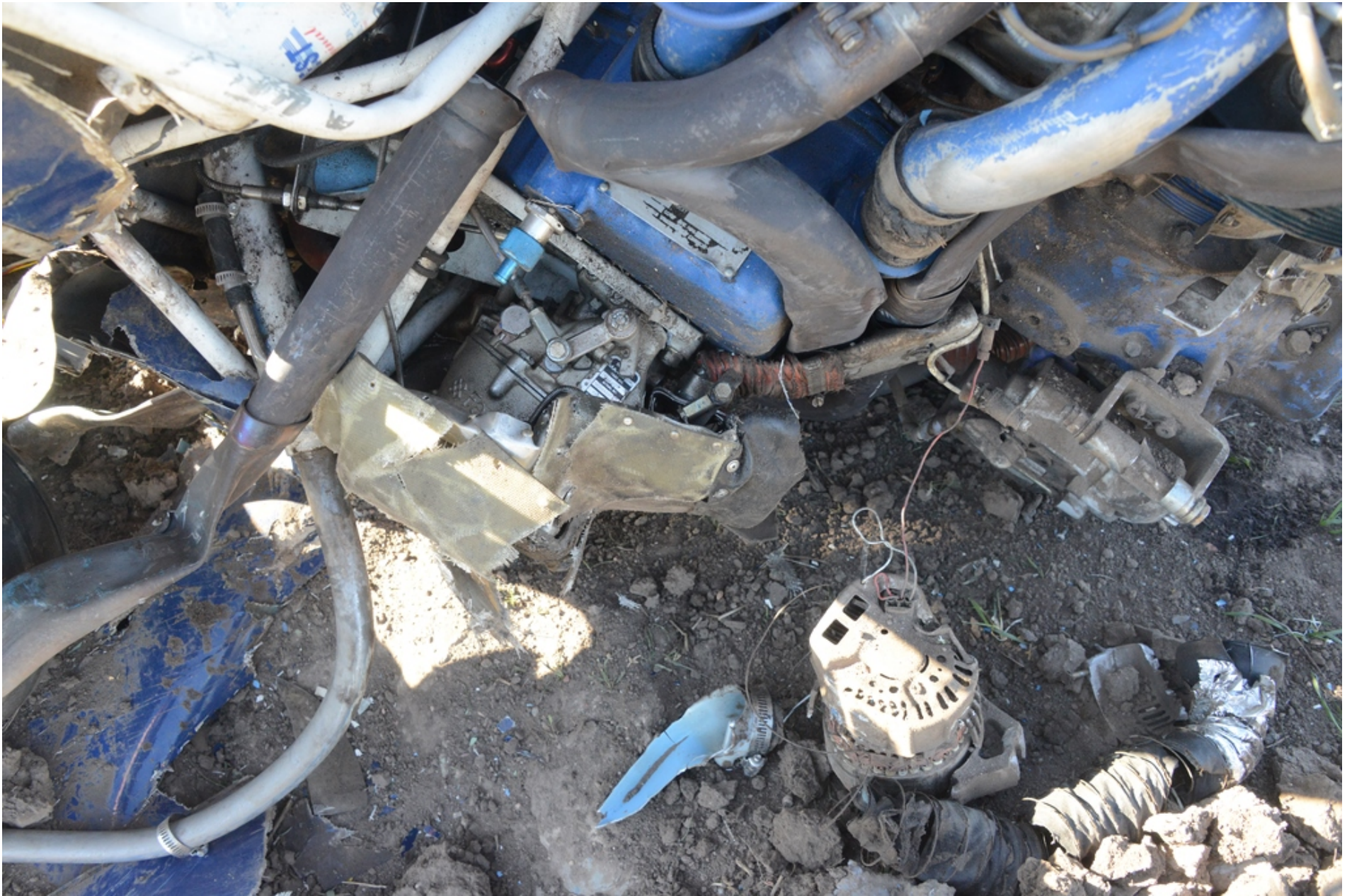
Photo 12 - View of the carburetor and lower portion of the engine.
