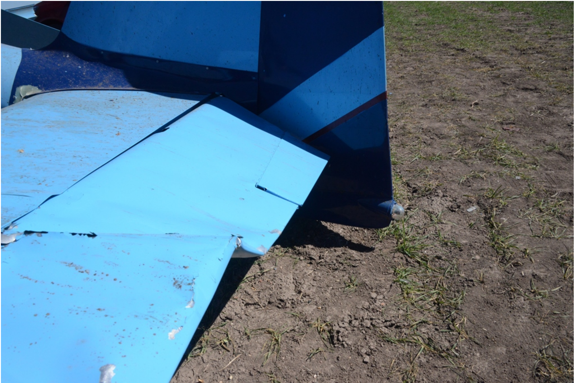
Photo 20 - View of an elevator with its trim tab near a neutral position.
