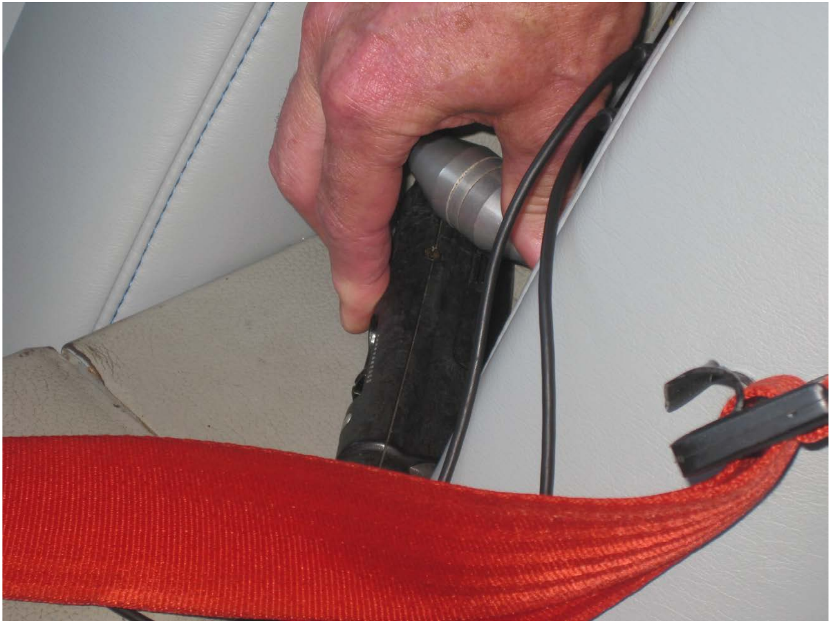
Photo 3 – View of student pilot’s headset control unit lodged under canopy security handle (Courtesy of FAA)
