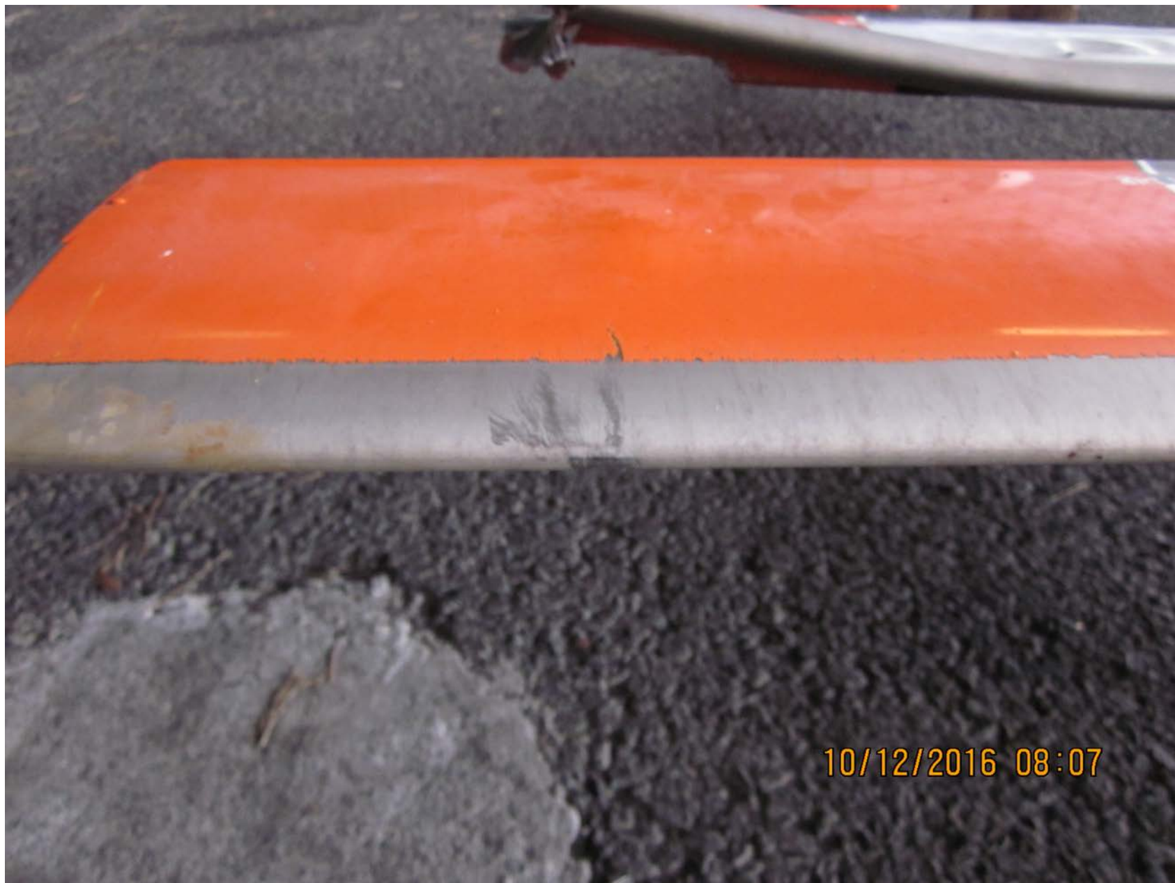
Photo 9 – Second damaged blade
