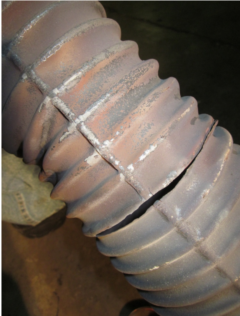
Photo 3 – Crack in Muffler – FAA Photo
