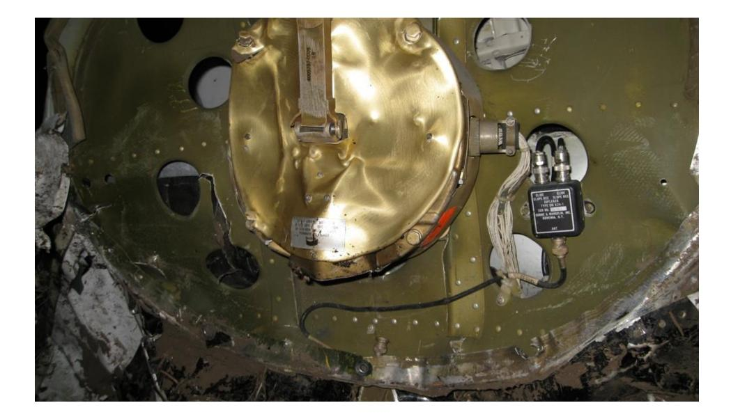
Photo 11 – Coaxial Glideslope Antenna Cable and Glideslope Signal Diplexer
