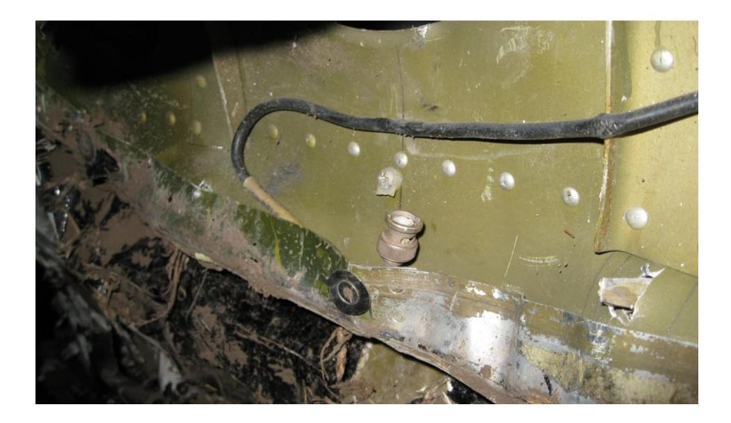
Photo 12 – Coaxial Glideslope Antenna Cable
