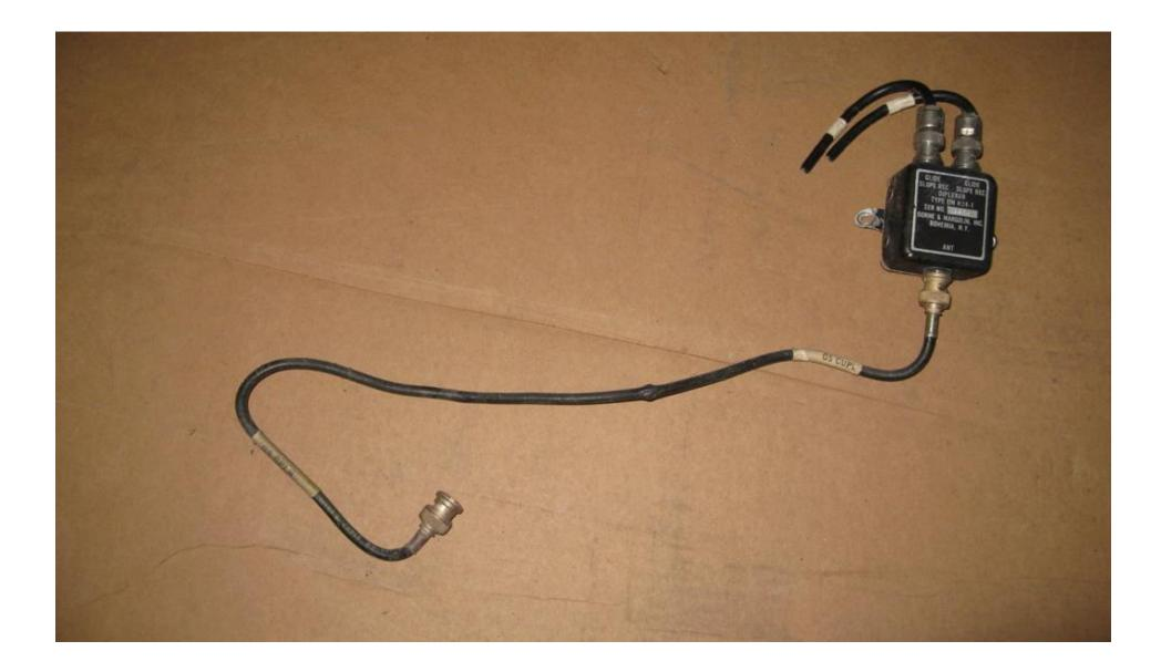
Photo 13 - Coaxial Glideslope Antenna Cable and Glideslope Diplexer
