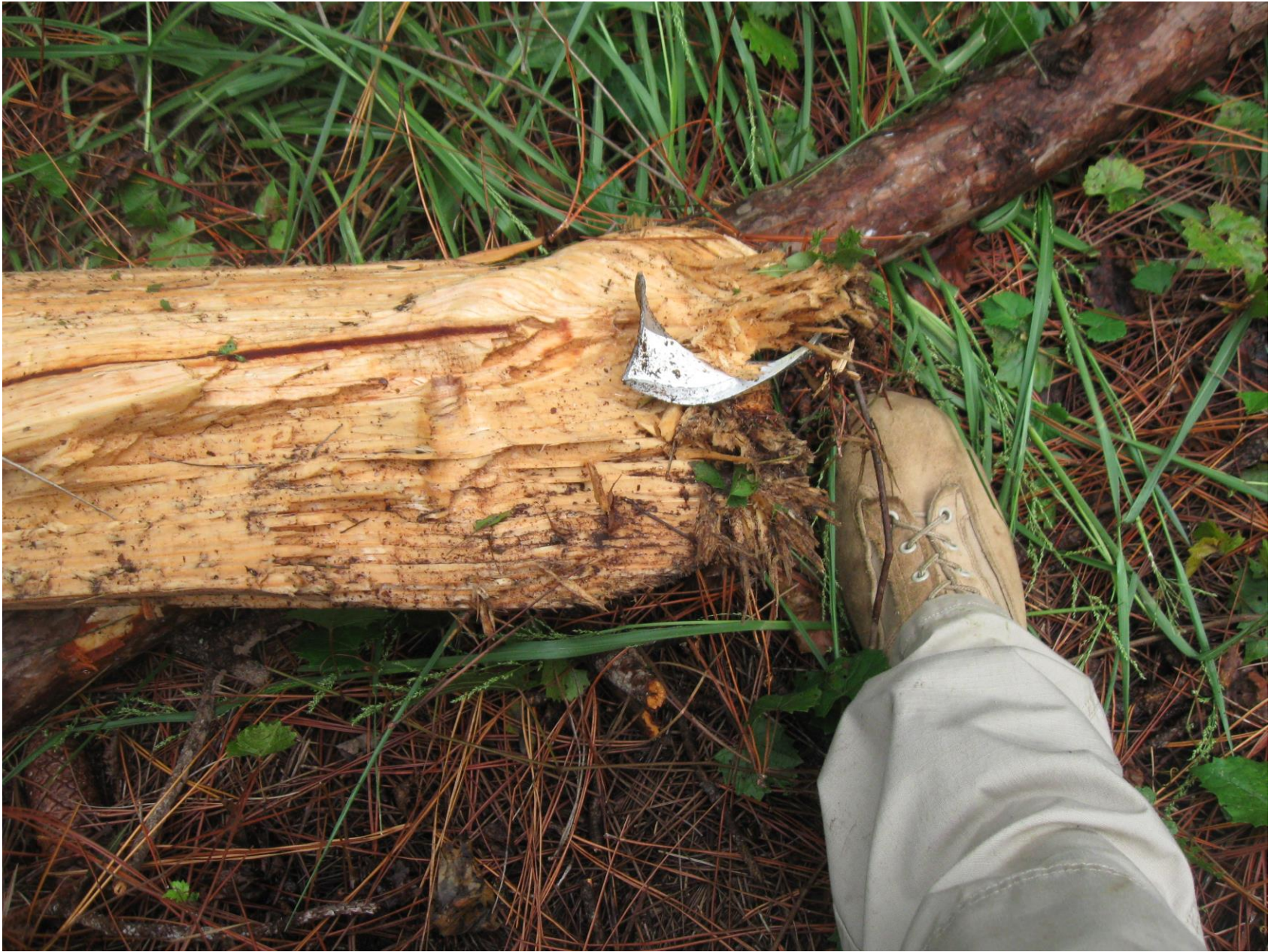
Photo 5 - View of Angular Cut Tree Trunk with Fractured Propeller Tip Embedded (Side View)
