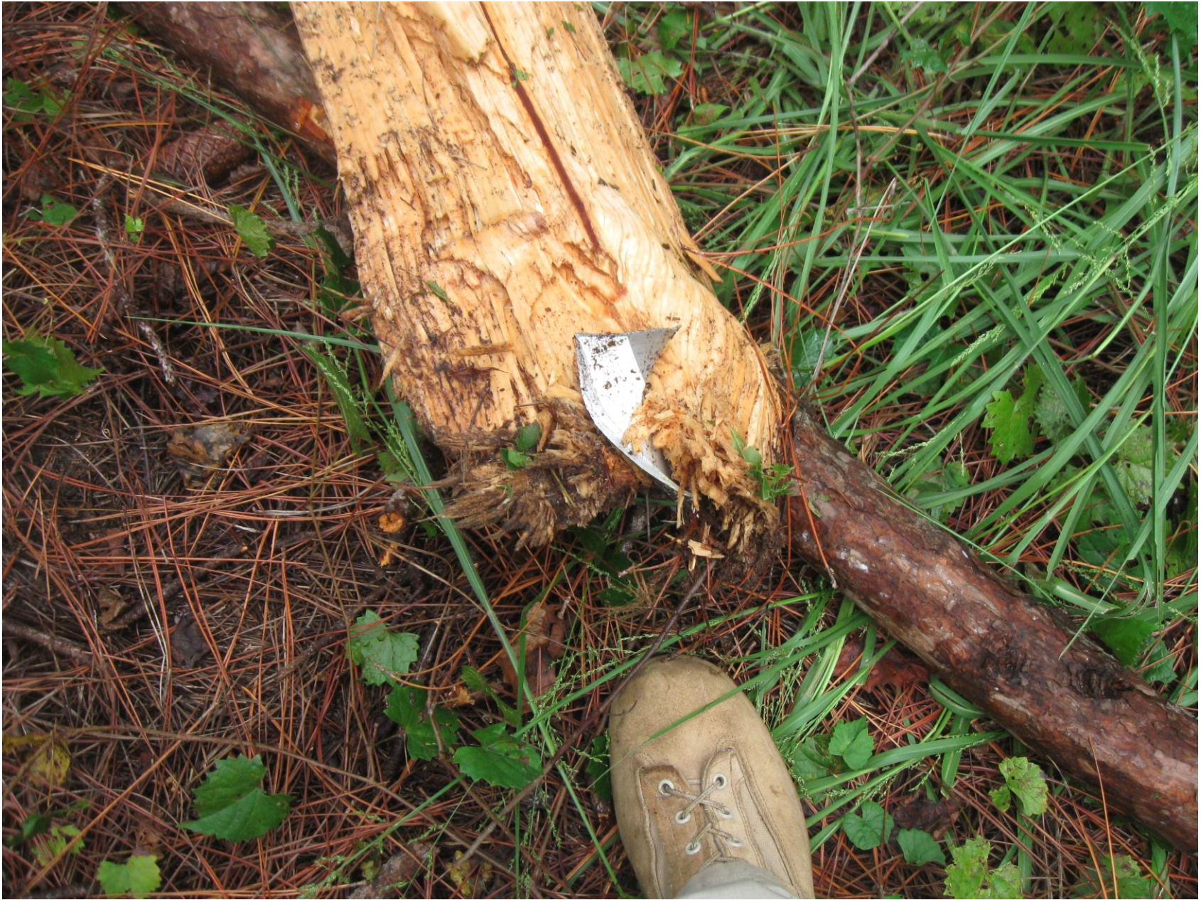
Photo 4 – View of Angular Cut Tree Trunk with Fractured Propeller Tip Embedded
