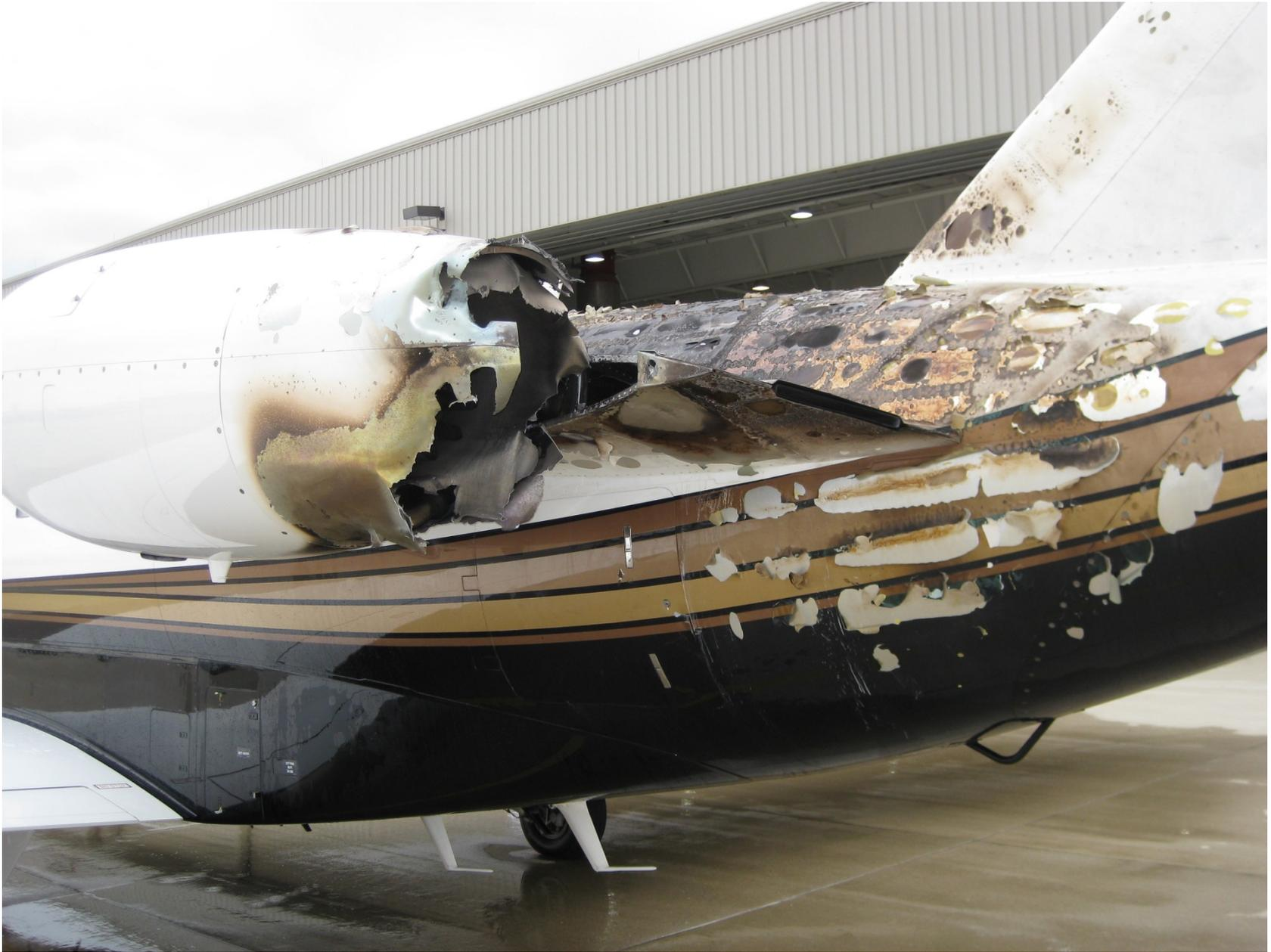
**Photo 3 – View of damage to left engine cowling and tail cone (FAA Photo)**
