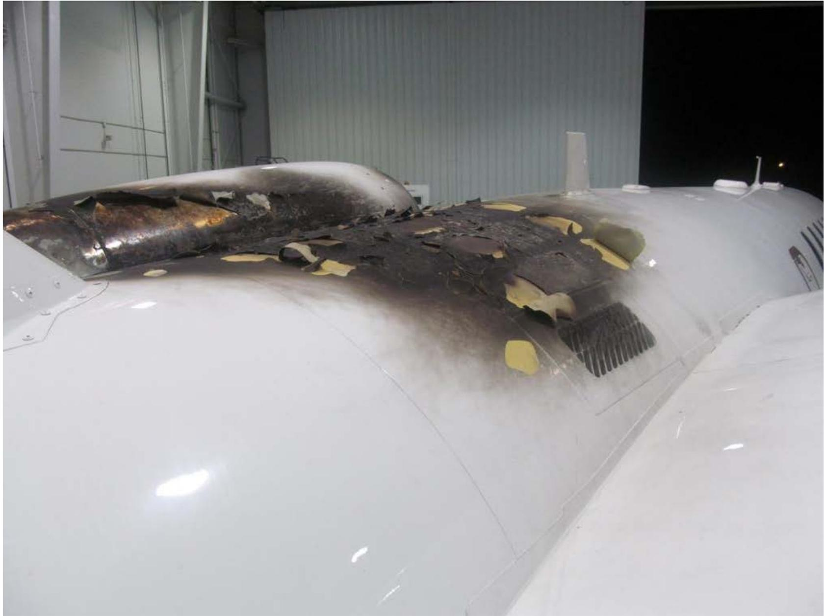
**Photo 5 – View of damage to the top of the tail cone and left engine cowling (Cessna Photo)**
