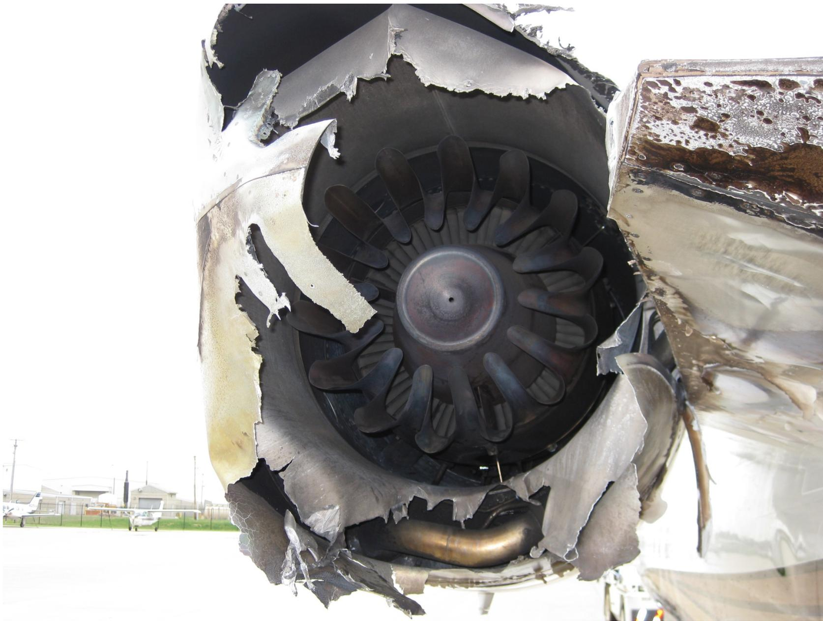
**Photo 4 – View of damage to the rear of the left engine area (FAA Photo)**
