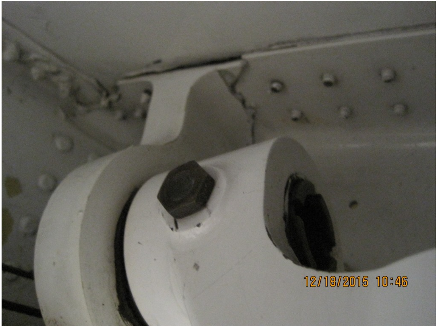
Photo 2 – View of substantial damage to the right landing gear trunnion (Courtesy of FAA)
