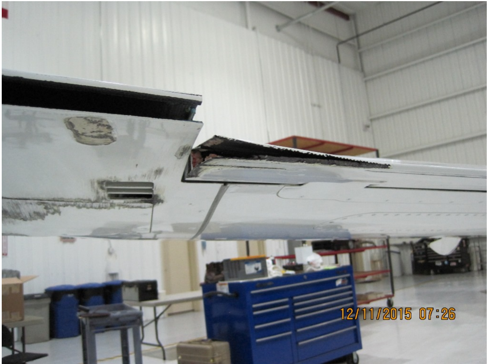
Photo 1 – View of substantial damage left wing aileron (Courtesy of FAA)
